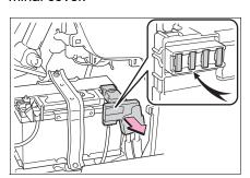
Remove the fuse with the pullout tool.Only type A fuse can be
