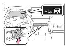
The height can be adjusted by pressing the height control switch.
