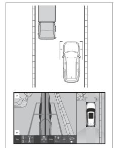
Check the positions and distance between the vehicle width guide line and a target object such as the obstacle or curb of the road. 4
