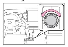
► Front-wheel drive control switch is in "4L"
