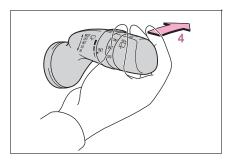
Pushing the lever operates the wiper and washer.
