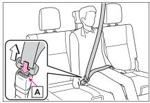
2 Insert the mechanical key (→P.112) or plate B into the notch of buckle and remove the belt.
