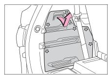
2 Unhook the belt, and loosen and remove the jack.
