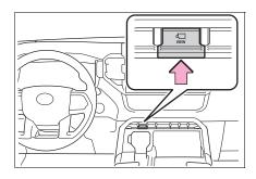
■ The Multi-terrain Monitor is displayed by operating ☐ when when vehicle speed is approximately 10 mph (16 km/h) or less. If the vehicle speed exceeds approximately 10 mph (16 km/h), the Multi-terrain Monitor display is canceled.
