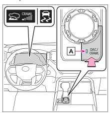
2 Turn the mode select switch left or right to select a mode on the multi-information display.
