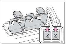
2 Return the head restraint securely to the locked position. (→P.156)
