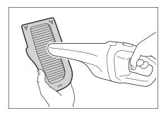
6 Reinstall the filter to the cover.
