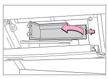
4 Unlock the filter cover (A), pull the filter cover out of the
