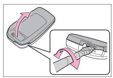
3 Remove the depleted battery.
