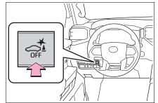
When the Parking Support Brake is disabled, the PKSB OFF indicator (→P.91) illuminates.
