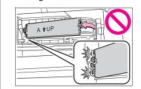
To prevent the fuel economy from being affected, visually inspect the hybrid battery (traction battery) air intake vent periodically for dust and clogs. If it is dusty or clogged or if "Maintenance Required for Traction Battery Cooling Parts See Owner's Manual" is displayed on the multi-information display, clean the air intake vent using the following procedures:
