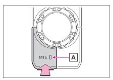
2 Select the Multi-terrain Select modes on the multi-information display while turning the mode select switch left and right.
