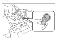
The hybrid system does not start and modes will be changed each time the switch is pressed. (→P.215)
