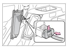
4 Remove the air intake vent filter.
