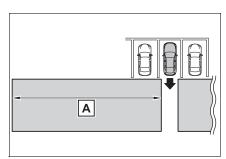
The buzzer can alert for faster vehicles approaching from farther away.
