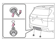
2 Pull the lower edge of the hitch cover toward you and remove the 10 craws.
