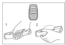
1 Grip the driver's door handle to unlock the door. Holding the driver's door handle for approximately 2 seconds unlocks all the doors. Grip front passenger door handle to unlock all the doors.\*
