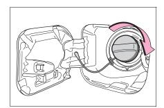
The fuel tank cap may be unfastened or loose. Turn the power switch to OFF, check the cap and tighten it securely. If the message remains, wait a few seconds and then turn the power switch to OFF once again.
