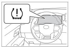
After 2 minutes, registration of a second wheel set is being performed. The tire pressure warning light will turn off and "--" will be displayed for the inflation pressure of each tire on the multi-information display.
