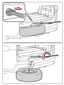
4 After the tire is lowered completely to the ground, remove the holding bracket.
