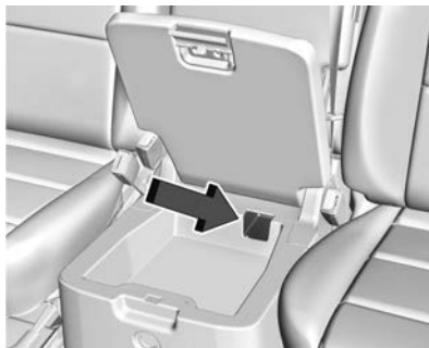
Transmitter Pocket without Bucket Seats (Lower Compartment)
