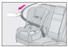
6 While pushing the child restraint system into the rear seat, allow the shoulder belt to retract until the
