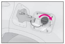
2 Close the fuel filler door, and press the center of the rear edge of the fuel filler door.
