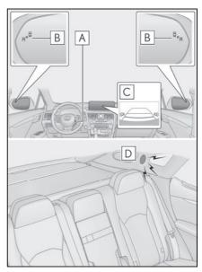
A Meter control switches Turning the RCTA function on/off. When the RCTA function is disabled, the RCTA OFF indicator illuminates.
