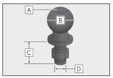
A Trailer ball load rating Matches or exceeds the gross trailer weight rating of the trailer.
