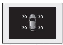
If the tire pressure drops below a predetermined level, the driver is warned by a screen display and a warning light. (→P.397)
