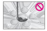
If the spare tire clamp bolt is turned without a tire on the hoist assembly, the wire cable may not be able to be lowered. If the wire cable cannot be lowered, contact your Lexus dealer.
