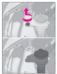
3 Turn the bulb base counterclockwise and remove it.
