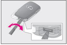
**3** Remove the depleted battery.
