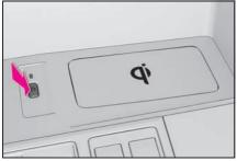
Place a portable device on the 2 charging area with its charging surface facing down.
