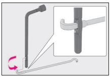
Connect the jack handle to the adapter socket. Turn the jack handle counterclockwise.
