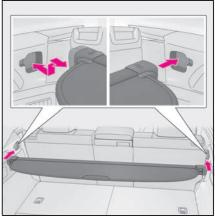
2 Pull out the luggage cover and hook it onto the anchors.
