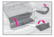
**2** Attach the hook to the upper edge of the back door opening as shown.
