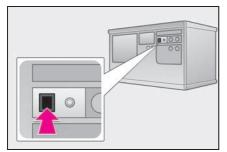
3 Press and hold the desired HomeLink<sup>®</sup> button (inside the vehicle) for 2 seconds and release it. Repeat this sequence (press/hold/release) up to 3 times to complete programming. If the garage door opener motor operates when the HomeLink<sup>®</sup> button is pressed, the garage door opener motor recognizes the HomeLink<sup>®</sup> signal.
