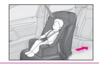
Do not allow the child to lean his/her head or any part of his/her body against the door or the area of the seat, front or rear pillars, or roof side rails from which the SRS side airbags or SRS curtain shield airbags deploy even if the child is seated in the child restraint system. It is dangerous if the SRS side airbags and curtain shield airbags inflate, and the impact could cause death or serious injury to the child.
