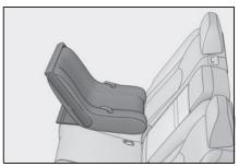
3 Run the seat belt through the child restraint system and insert the plate
