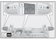
A Meter control switches Turning the Blind Spot Monitor on/off. **B** Outside rear view mirror indicators When a vehicle is detected in a blind spot of the outside rear view mirrors or approaching rapidly from behind into a blind spot, the outside rear view mirror indicator on the detected side will illuminate. If the turn signal lever is operated toward the detected side, the outside rear view mirror indicator flashes.
