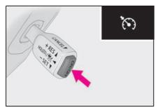
2 Accelerate or decelerate, with accelerator pedal operation, to the desired vehicle speed (at or above approximately 20 mph [30 km/h]) and push the lever down to set the speed.
