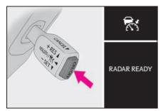
2 Accelerate or decelerate, with accelerator pedal operation, to the desired vehicle speed (at or above approximately 20 mph [30 km/h]) and push the lever down to set the speed.
