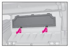
Unlock the filter cover (A), pull the filter cover out of the claws (B), and remove the filter cover.
