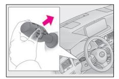
Temporarily switching to the low beams
