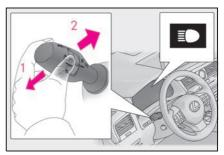
With the headlights on, push the lever away from you to turn on the high beams. Pull the lever toward you to the center position to turn the high beams off.
