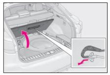
3 Attach the hook to the upper edge of the back door opening as shown.
