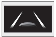
Indicates that the system is recognizing white (yellow) lines or a course<sup>\*</sup>. When the vehicle departs from its lane, the white line displayed on the side the vehicle departs from flashes orange.  Inside of displayed white lines is black
