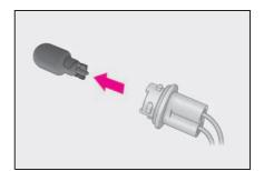
4 Install a new light bulb and then install the bulb base to the light unit by inserting it and turning it clockwise.
