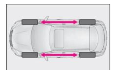
To equalize tire wear and extend tire life, Lexus recommends that tire rotation is carried out at the same interval as tire inspection.
