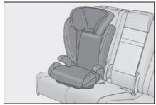
4 Sit the child in the child restraint system. Fit the seat belt to the child restraint system according to the manufacturer's instructions and insert the plate into the buckle. Make sure that the belt is not twisted. Check that the shoulder belt is correctly positioned over the child's shoulder and that the lap belt is as low as possible.  $(\rightarrow P.26)$
