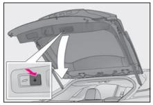
Closing the power back door using the back door handle
