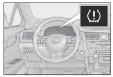
7 Drive the vehicle at approximately 25 mph (40 km/h) or more for approximately 10 to 30 minutes until the inflation pressure of each tire is displayed on the multi-information display.
