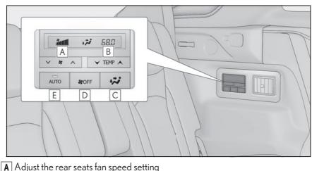
$\land$  to increase the fan speed and  $\checkmark$ Press 😽 **\*** to decrease the fan speed.
