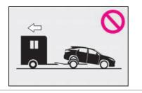
AWD models: Never tow this vehicle with any of the wheels on the ground. This may cause serious damage to the transmission and Dynamic Torque Control AWD system.
