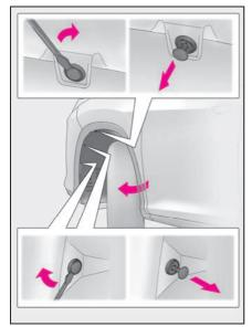
2 Pull back the fender liner until the connector is visible.
