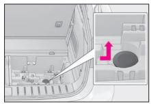
3 Attach the adapter socket to the spare tire clamp bolt.
