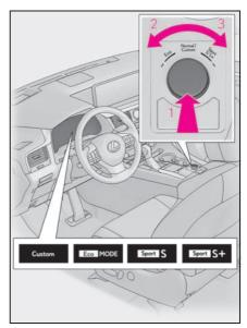
1 Normal mode/Custom mode Normal mode and custom mode are selected by pressing the driving mode select switch. Each time the switch is pressed, the driving mode changes between normal mode and custom mode. When custom mode is selected, the "Custom" indicator will be illuminated. When Eco drive mode or sport mode is selected, pressing the switch changes the driving mode to normal mode.
