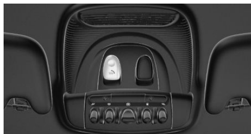
SOS button in the roofliner
