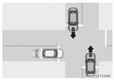
Junction Crossing function can help avoid a collision with oncoming vehicles on the left or right side when crossing an intersection by applying emergency braking. Also, Junction Crossing function may assist with braking your vehicle to help reduce collision speed or avoid a collision.
