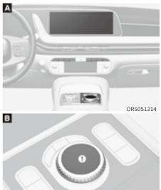
(A): Front seat, (B): Rear seat (if equipped)(D): Infotainment system controller
