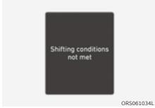
This message is displayed when engine RPM is too high, or when driving speed is too fast to shift the gear.
