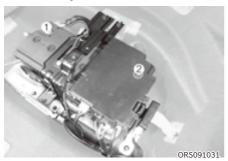
When replacing the battery, disconnect the negative (-) cable ① and remove the positive (+) battery fuse box ②.
