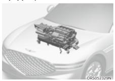
Freshens a vehicle's inner space by deodorization of lingering odor through PCM installed in HVAC system.
