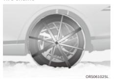
Since the sidewalls on some radial tires are thinner than other types of tires, they may be damaged by mounting certain types of tire chains on them. Do not mount tire chains on vehicles equipped with aluminum wheels; if possible use AutoSock® (fabric snow chain or similar). Install AutoSock® after reviewing the instructions provided with AutoSock®. Damage to your vehicle caused by improper use of fabric snow chains are not covered by your vehicle manufacturer's warranty.
