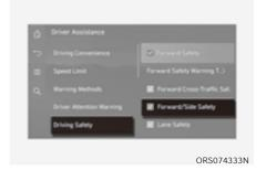
With the engine on, select or deselect 'Driver Assistance → Driving Safety → Forward/Side Safety' from the Settings menu to turn on Lane-Change Oncoming function, Lane-Change Side function,
