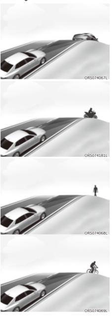
Forward Collision-Avoidance Assist may not detect other vehicles, powered two-wheelers, pedestrians or cyclists in front of you while driving uphill or downhill, adversely affecting the performance of the sensors.
