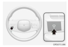
Each time the button is pressed, the headway changes as follows:
