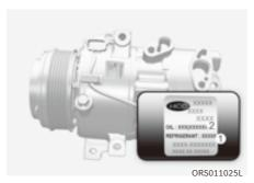
A compressor label informs you the type of compressor your vehicle is equipped with such as model, supplier part number, production number, refrigerant ① and refrigerant oil ②.
