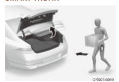
On a vehicle equipped with a smart key, the trunk can be opened with hands-free activation using the smart trunk system.
