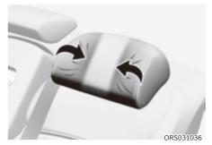
While driving, the wing-out head restraint supports the passenger's head from shaking. Hold both ends of the wing-out head restraint with your hands, and pull out or push in to adjust its position.
