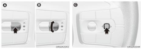
The cluster display modes can be changed by using the control switches.
