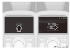
Convenience features can be adjusted using the rear armrest touchscreen. Quickly touch the screen twice to start the display. Climate, Seat, Massage, Lights, and Shades are adjustable from the armrest touchscreen.
