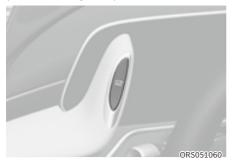
When the trunk is closed, press the power trunk open/close button for 1 second. The power trunk will open with a warning sound.
