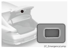
The trunk emergency lamp turns on when the trunk is opened.
