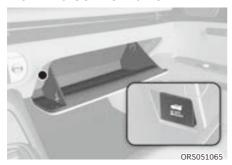
When the trunk lid control button is in the UNLOCK (button not pressed) position, the trunk can be controlled with the power trunk open or close button.
