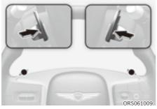
The paddle shifter allows the driver to shift gears without taking one's hands off the steering wheel.
