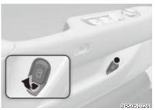
If the door does not open with the door open button due to battery discharge or vehicle breakdown, pull the emergency open lever under the door pocket twice to open the door. You may use the emergency open lever even if there is no problem with the door open button.
