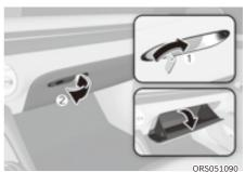
The glove box can be locked and unlocked with the mechanical key ①.
