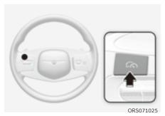
Press the Driving Assist (A) button to turn Manual Speed Limit Assist off. The Speed Limit (A) indicator will go off.
