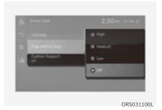
Select 'Setup → Seat → Driver Seat → Cushion Support' from the infotainment system. The driver's seat cushion support can be adjusted to high, normal, and low, or turned off.
