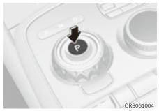
To shift the gear to R (Reverse), press the P button while depressing the brake pedal.
