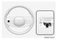
Press the **II** switch to temporarily pause the set speed limit. The set speed limit will turn off but the Speed Limit (**S**LIMIT) indicator will stay on.
