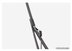
3. Disassemble the washer fluid hose by pulling downward while bending down the end of blade.
