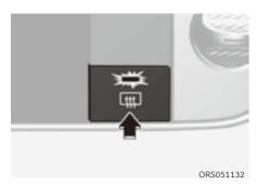
The defroster heats the window to remove frost, fog and thin ice from the interior and exterior of the rear window, while the engine is running.
