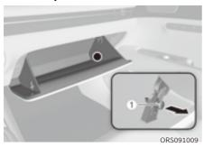
1. Open the glove box and remove the support rod ①.
