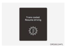
Transmission cooled and safe to drive This message is displayed when the vehicle is safe to drive.
