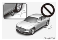
Never start or run the engine while an AWD vehicle is raised on a jack. The vehicle can slip or roll off of a jack causing serious injury or death to you or those nearby.
