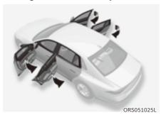
To close the door remotely, point the smart key towards the vehicle and press and hold the door lock button on the smart key for over 3 seconds while the engine is turned off. If the distance from the vehicle and your smart key changes while the door is being closed, the door may not be completely closed. Do not stand too far away from the door when remotely closing the door.
