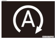
ISG system is not activated, when the prerequisites to activate the ISG system are unsatisfied.
