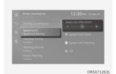
With the engine on, when 'Driver Assistance → Speed Limit → Speed Limit Offset' is selected, the Speed Limit Offset can be changed. Speed Limit Warning and Speed Limit Assist will operate by applying the Speed Limit Offset setting to the detected speed limit.
