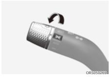
The parking lamp, license plate lamp and instrument panel lamp are turned ON.
