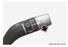
In the OFF position, pull the lever gently toward you to spray washer fluid on the windshield.
