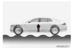
The vehicle adjusts vehicle height, spring stiffness, and shock absorber damping force when driving on a rough terrain such as an unpaved road, to optimize comfort and protect the vehicle.
