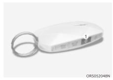
You can open the window remotely with the smart key.
