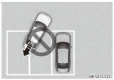
If Remote Smart Parking Assist is used in a parking space where the vehicle next to you is parked crooked, your vehicle can avoid contacting parked vehicles but may not park side by side.
