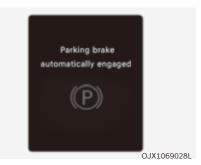
Parking brake automatically engaged When EPB is applied while Auto Hold is activated, a warning will sound and a message will appear.
