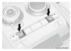
While the engine is on, press the seat heater button on the center console to select the temperature level.
