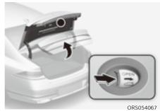
Your vehicle is equipped with an emergency trunk safety release lever located inside the trunk. When someone is inadvertently locked in the trunk, the trunk can be opened by moving the lever in the direction of the arrow and pushing the trunk lid to open.
