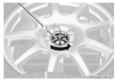
If it is hard to loosen the tire hold-down wing bolt by hand, you can loosen it easily using the wheel lug wrench ③. Turn the tire hold-down wing bolt counterclockwise with the wheel lug wrench.
