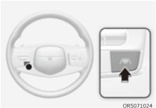
With the engine on, press and hold the Lane Driving Assist (♠) button located on the steering wheel to turn on and off. When Lane Keeping Assist is on, the gray or green / indicator illuminates.
