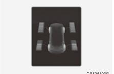
**Driving force distribution (if equipped)** The distribution status of the driving power of the front and rear wheels are displayed when Auto AWD mode is activated.
