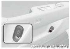
The door emergency lever lamp turns on when the light switch is turned on and all the doors are locked.
