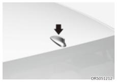
The shark fin antenna receives transmitted data (for example, AM/FM).
