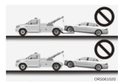
The flatbed tow truck must be a safety loader type which has a loading angle less than 6°.
