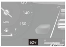
This gauge indicates the current outside air temperatures by increments of 1°F (1°C).
