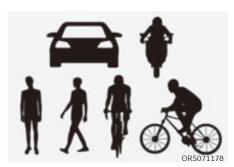
The illustration above shows the image the front view camera and front radar are capable of detecting as a vehicle, powered two-wheeler, pedestrian and cyclist.
