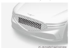
The active air flap system controls the air flap below the front bumper to cool vehicle parts and improve fuel efficiency.
