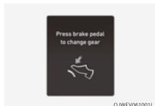
This message is displayed when the brake pedal is not depressed while shifting the gear.
