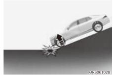
The vehicle adjusts vehicle height, spring stiffness, and shock absorber damping force when driving over a steep slope, to optimize comfort and protect the vehicle.
