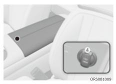
5. Plug the compressor power cord (9) into the vehicle power outlet.
