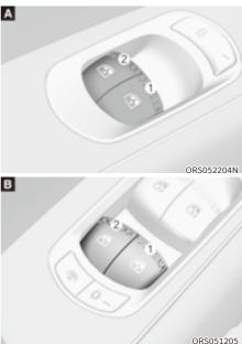
(A): Rear window switch, (B): Driver's window switch Use to block sunlight coming through the rear windows.
