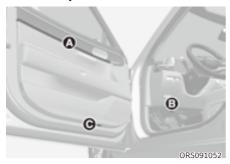
Mood lamp (A): The lamp turns on when 'Setup → Vehicle → Lights → Ambient Light' is selected from the infotainment system screen.
