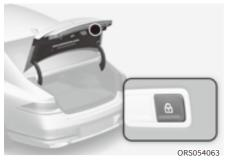
Press the power trunk lock button while carrying the smart key. The power trunk closes and locks automatically.
