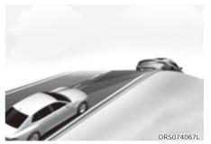
During uphill or downhill driving, Smart Cruise Control may not detect a moving vehicle in your lane, and cause your vehicle to accelerate to the set speed. Also, vehicle speed will rapidly decrease when the vehicle ahead is detected suddenly.
