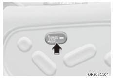
Seating position, seatback angle and cushion angle of the front passenger seat can be adjusted by operating the rear seat control switches.
