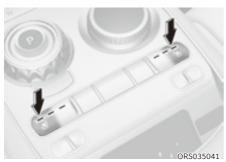
While the engine is on, press the seat ventilator button on the center console to select the intensity level.
