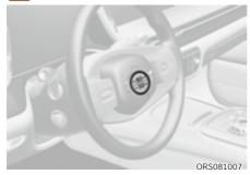
Detach the speed restriction label ① from the sealant bottle 2, and place it in a highly visible place inside the vehicle such as on the steering wheel to remind the driver not to drive too fast.
