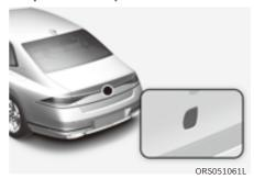
When the trunk is closed, press the power trunk open button to open the trunk
