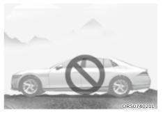
Remote Smart Parking Assist may cancel when the vehicle slips, or the vehicle cannot move due to road conditions such as pebbles or fragmented stones.
