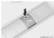
Press the Parking Safety (Pma) button to turn on Forward/Reverse Parking Distance Warning. Press the button again to turn off the function.
