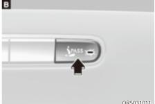
Seating position, seatback angle and cushion angle/height of the front passenger seat can be adjusted by operating the switches from the driver's seat.
