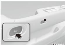
Press the door open button from inside the vehicle to open the door.
