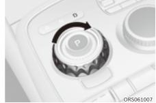
To shift the gear to D (Drive), rotate the shift dial clockwise while depressing the brake pedal.
