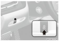
Electronic Stability Control helps to stabilize the vehicle during cornering maneuvers.
