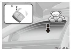
If a window senses any obstacle while it is closing automatically, it will stop and lower about 12 in. (30 cm) to allow the object to be cleared.
