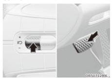
Press the **|| )** switch or depress the brake pedal to temporarily cancel Smart Cruise Control.
