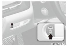
Press the ISG OFF button to turn off ISG system. The ISG OFF button indicator will illuminate. To use the system, press the ISG OFF button again.
