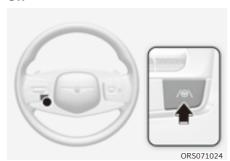
With the engine on, shortly press the Lane Driving Assist button located on the steering wheel to turn on Lane Following Assist. The grey or green  $\bigcirc$  indicator light will illuminate on the cluster.
