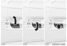
To resume Manual Speed Limit Assist after the function was paused, operate the +, -, || 5 switch.
