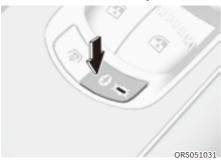
When the electronic child safety lock button is pressed and the indicator light on the button illuminates, the rear doors cannot be opened from inside the vehicle.
