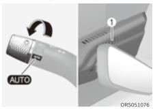
The parking lamp and headlight will be turned ON or OFF automatically depending on the amount of daylight as measured by the ambient light sensor ① at the upper end of the windshield glass.
