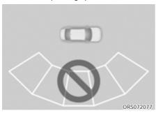
Remote Smart Parking Assist does not work properly when the parking lines are not parallel. Do not park even if the parking space is recognized by the sensor.
