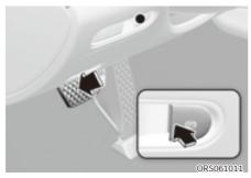
To release EPB (Electronic Parking Brake):
