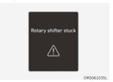
If the dial does not return to its original position after turning the shift dial, the above warning message is displayed. Have the vehicle inspected by an authorized retailer of Genesis Branded products.
