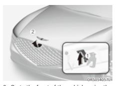
Go to the front of the vehicle, raise the hood slightly, push up the secondary hood release lever ① inside of the hood center and lift the hood ②.
