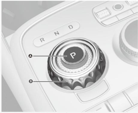
Depress the brake pedal whenever rotating the shift dial to change gear or shifting P.
