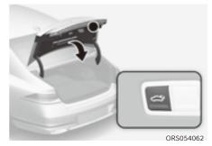
Press the power trunk close button. The trunk closes automatically.
