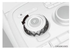
To shift the gear to R (Reverse), rotate the shift dial counterclockwise while depressing the brake pedal.
