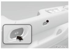
If Safe Exit Assist detects a vehicle approaching the rear corner of your vehicle, the the doors will not open even if the door open ((())) button is pressed.
