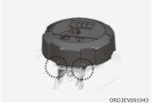
2. Make sure that the tiny protrusions inside the coolant cap are securely interlocked.
