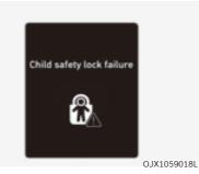
When electronic child safety lock does not work even though the button is pressed, the message will be displayed and an alarm will sound. If this occurs, have the vehicle inspected by an authorized retailer Genesis Branded
