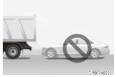
Do not use Remote Smart Parking Assist around vehicles with higher ground clearance, such as a bus, truck, etc. It may lead to an accident.
