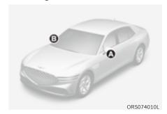
(camera located at bottom of the mirror)
