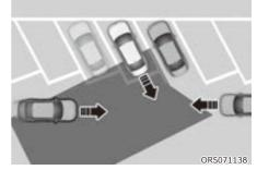
Rear Cross-Traffic Collision-Avoidance Assist may be limited when backing up diagonally, and may not detect the vehicle approaching from the left or right. If this occurs, the function may not warn the driver or control the brakes when necessary.
