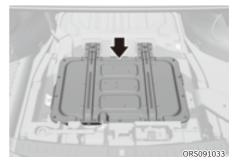
Vehicles with a 48V battery have the battery in the trunk. Have the battery replaced by an authorized retailer of Genesis Branded products.
