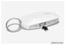
When the trunk is closed, press the power trunk open button for 1 second. The trunk will open with a warning sound.
