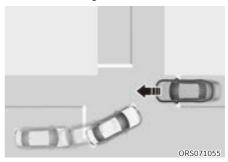
Junction Turning function can help avoid a collision with an oncoming vehicle in an adjacent lane when turning left at a crossroad with the turn signal on by applying emergency braking. Also, Junction Turning function may assist with braking your vehicle to help reduce collision speed or avoid a collision.
