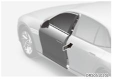
If a door does not close completely but is closed to the first detent position, the door will close automatically.
