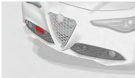
Front Fascia/Bumper Radar Location
