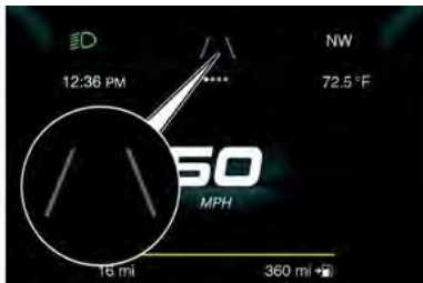
Lane Markings Not Detected
