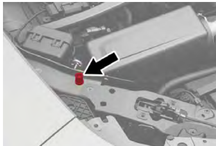
Remote Negative (-) Post Location
