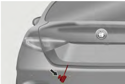
Manual Release Cord Shown With Trunk Closed
