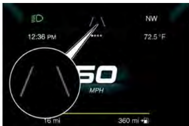
Lane Markings Not Detected
