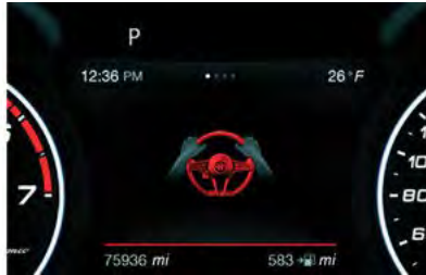
Hand Presence On The Steering Wheel Not Detected Display (Up To 6 Seconds)
