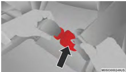
Detaching Mini-Buckle With Seat Belt Tongue
