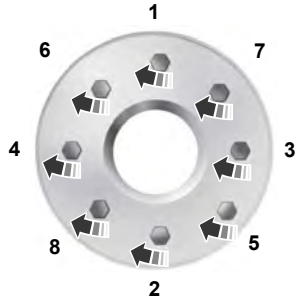
8-lug nut torque sequence
