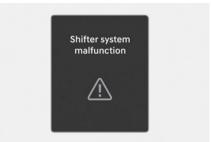
This message appears when the transmission or the shift dial does not properly operate in the P (Park) position.
