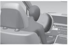
When the SRSCM detects a sufficiently severe impact to the front of the vehicle, it automatically deploys the front airbags.
