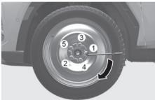
12.Use the wheel lug wrench to tighten the lug nuts in the order shown. Double-check each lug nuts until they are tight. After changing tires, have the vehicle inspected by an authorized HYUNDAI dealer tighten the lug nuts to their proper torque as soon as possible. The lug nut should be tightened to 79-94 lbf. ft (11-13 kgf.m). If you have a tire gauge, check the tire pressure (refer to the "Tires and wheels" section in chapter 10 for tire pressure instructions.).
