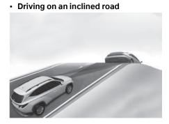
During uphill or downhill driving, the Smart Cruise Control may not detect a moving vehicle in your lane, and cause your vehicle to accelerate to the set speed. Also, vehicle speed will rapidly decrease when the vehicle ahead is detected suddenly.
