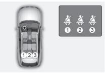
As a reminder to the rear passenger, the rear passenger's seat belt warning lights will illuminate for about 6 seconds each time the Engine Start/Stop button is in the ON position regardless of belt fastening.
