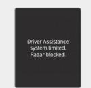
When the rear bumper around the rear corner radar or sensor is covered with foreign material, such as snow or rain, or installing a trailer or carrier, it can reduce the detecting performance and temporarily limit or disable Safe Exit Warning.
