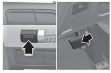
Press the **IID** switch or depress the brake pedal to temporarily cancel Smart Cruise Control.
