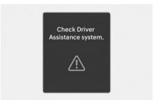
When Lane Keeping Assist is not working properly, the '**Check Driver Assistance system.**' warning message appears and the master (A) warning light and yellow Lane Safety (A) indicator light illuminates on the instrument cluster. If this occurs, have your vehicle inspected by an authorized HYUNDAI dealer.
