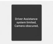
When the front windshield where the front view camera is located or the sensor is covered with foreign material, such as snow or rain, it can reduce the detecting performance and temporarily limit or disable Forward Collision-Avoidance Assist.
