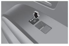
While the engine is running, press the button to warm the driver's seat or front passenger's seat.
