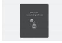
In the following situation, the "Watch for surrounding vehicles" warning message will appear on the instrument cluster, and an audible warning will sound and steering wheel will vibrate to warn the driver of road conditions ahead.
