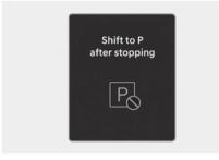
This message appears when the gear is shifted to P (Park) while the vehicle is moving.
