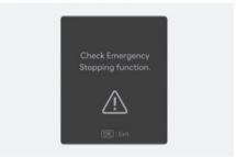
When Emergency Stop is not working properly, the "**Check Emergency Stopping function.**" warning message appears, and the master (A) warning light illuminates on the instrument cluster. If this occurs, have your vehicle inspected by an authorized HYUNDAI dealer.
