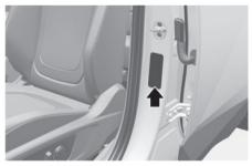
The vehicle certification label attached on the driver's side center pillar gives the vehicle identification number (VIN).
