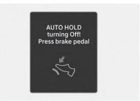
When the conversion from Auto Hold to EPB is not working properly, a warning sounds and a message appears.
