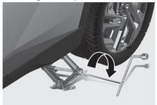
8. Insert the jack handle and wheel lug wrench into the jack and turn it clockwise, raising the vehicle until the tire clears the ground. Make sure the vehicle is stable on the jack. 9. Loosen the lug nuts with the wheel lug nuts wrench and remove them with your fingers.
