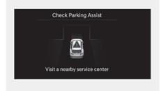
When Remote Smart Parking Assist is not working properly, the "**Check Parking Assist**" warning message will appear on the infotainment system. If the message appears, stop using Remote Smart Parking Assist, and have your vehicle inspected by an authorized HYUNDAI dealer.
