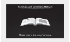
When "**Parking Assist Conditions Not Met**" message appears when Parking/View (沪) button has been pressed and held while Remote Smart Parking Assist is in standby. After a while, press and hold the Parking/View (沪) button again to see if Remote Smart Parking Assist works.
