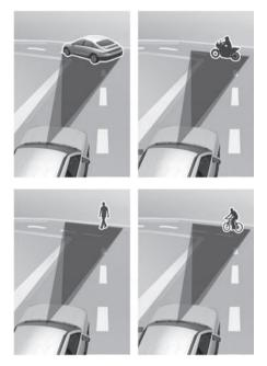
Forward Collision-Avoidance Assist may detect a vehicle, powered two-wheeler, pedestrian or cyclist in the next lane or outside the lane when driving on a curved road.
