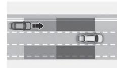
Blind-Spot Collision-Avoidance Assist helps detect and informs the driver that a vehicle is approaching at high speed from the blind spot area.
