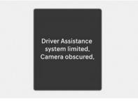
When the front windshield where the front view camera is located is covered with foreign material, such as snow or rain, it can reduce the detecting performance and temporarily limit or disable Driver Attention Warning.
