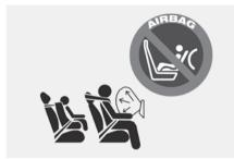
Even though your vehicle is equipped with the OCS, never install a Child Restraint System in the front passenger's seat. An inflating airbag may forcefully strike a child or child restraint resulting in serious or fatal injury.
