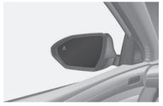
When the vehicle is detected in the rear left and right lanes, to warn the driver a vehicle is detected, the warning light on the side view mirror and Head-Up-Display (if equipped) will illuminates. Vehicle detection operates under following conditions.
