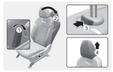
To remove the head restraint:
