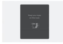
Forward Attention Warning determines whether the driver is focused on the road depending on information, such as the amount of time the driver is looking elsewhere, the amount of time the eyes are closed, how frequently the driver yawns, etc. If Forward Attention Warning judges the driver is not focused, the '**Keep** your eyes on the road.' warning message will appear on the cluster, and an audible warning will sound.
