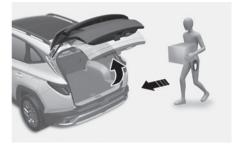
On a vehicle equipped with a smart key, the liftgate can be opened with hands-free activation using the smart liftgate system.
