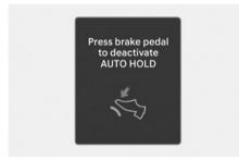
If you did not apply the brake pedal when you release Auto Hold by pressing the AUTO HOLD switch, a warning sounds and a message appears.
