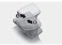
[A] Push the lever forwards once to shift up one gear.[B] Pull the lever backward once to shift down one gear.
