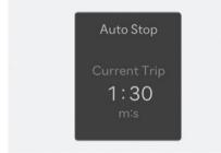
You can view the AUTO STOP elapsed time in the utility view. To view the elapsed time for **AUTO STOP** since the last reset, select **Setup > Cluster > AUTO STOP elapsed time** in the infotainment system. The AUTO STOP elapsed time reset depends on which utility view mode is linked.
