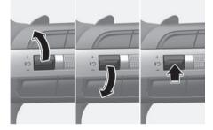
To resume Manual Speed Limit Assist after the function was paused, operate the +, -, IID switch.
