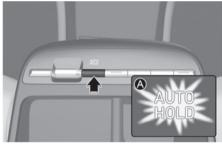
2. When you stop the vehicle completely by depressing the brake pedal, Auto Hold maintains the brake pressure to hold the vehicle stationary. The indicator changes from white to green.
