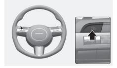
To turn Smart Cruise Control off, press the Driving Assist (෬ඁ) button.
