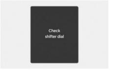
This message appears when there is a malfunction with the rotary gear shift dial. Have the vehicle inspected by an authorized HYUNDAI dealer.
