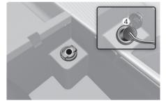
6. With the ignition switch ON, switch on the compressor and let it run for approximately 5~7 minutes to fill the sealant up to proper pressure. (refer to the "Tires and wheels" section in chapter 10). The inflation pressure of the tire after filling is unimportant and will be checked/corrected later.
