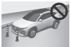
Remote Smart Parking Assist performance may reduce or collision with an obstacle may occur when there is a narrow object, circular pillar, square pillar, or a pillar surrounded by objects such as a fire extinguisher, etc., near the parking space. The driver should park the vehicle manually. • Parking in a parking space with a vehicle on one side only
