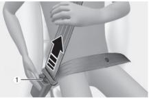
Press the release button (1) in the locking buckle.
