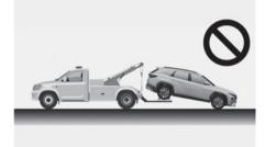
• Do not tow vehicles with sling-type equipment. Only use wheel lift or flatbed equipment.
