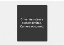
When the front windshield where the front view camera is located is covered with foreign material, such as snow or rain, it can reduce the detecting performance and temporarily limit or disable Intelligent Speed Limit Assist. If this occurs, the "**Driver Assistance system limited. Camera obscured.**" warning message and ( $\Box$ ) warning light will appear on the instrument cluster.
