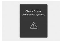
When Intelligent Speed Limit Assist is not working properly, the "**Check Driver Assistance system.**" warning message will appear on the instrument cluster for several seconds, and the master (A) warning light and ( $\Box$ ) warning light will illuminate on the instrument cluster. If this occurs, have your vehicle inspected by an authorized HYUNDAI dealer.
