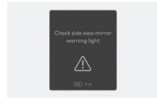
When the side view mirror warning light is not working properly, the "**Check side view mirror warning light**" warning message will appear on the instrument cluster for several seconds, and the master (**(**) warning light will illuminate on the instrument cluster. If this occurs, have your vehicle inspected by an authorized HYUNDAI dealer.
