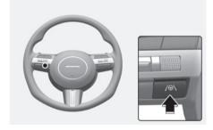
With the engine on, shortly press the Lane Driving Assist button located on the steering wheel to turn on Lane Following Assist. The gray or green (☉) indicator light will illuminate on the instrument cluster.
