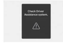
When Highway Driving Assist is not working properly, the "Check Driver Assistance system." warning message and yellow Lane Keeping Assist (/A) warning light appears on the instrument cluster. If this occurs, have your vehicle inspected by an authorized HYUNDAI dealer.
