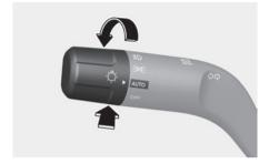
High Beam Assist automatically adjusts the headlights between high beam and low beam depending on the light detected from oncoming vehicles or vehicles in front using the front view camera.
