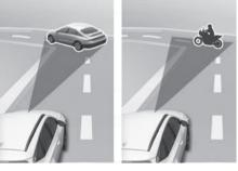
Forward Collision-Avoidance Assist may not detect other vehicles, pedestrians or cyclists in front of you when driving on curved roads adversely affecting the performance of the sensors. This may result in no warning or braking assist when necessary.
