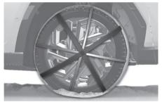
Since the sidewalls of radial tires are thinner than other types of tires, they may be damaged by mounting some types of tire chains on them. Therefore, the use of snow tires is recommended instead of tire chains. If tire chains must be used, use genuine HYUNDAI Parts and install the tire chains after reviewing the instructions provided with the tire chains. Damage to your vehicle caused by improper tire chain use is not covered by your vehicle manufacturer's warranty.
