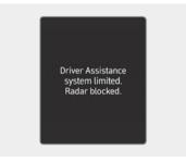
When the rear bumper around the rear-side radar or sensor is covered with foreign material, such as snow or rain, or installing a trailer or carrier, it can reduce the detecting performance and temporarily limit or disable Rear Cross-Traffic Collision-Avoidance Assist.
