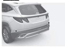
The rear corner radars are mounted near the rear corners of your vehicle above the bumper.
