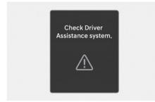
When Blind-Spot Collision-Avoidance Assist is not working properly, the "**Check Driver Assistance system.**" warning message will appear on the instrument cluster for several seconds, and the master (<u>A</u>) warning light will appear on the instrument cluster. If this occurs, have your vehicle inspected by an authorized HYUNDAI dealer.
