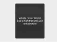
If you continue to drive with overheated transmission, the above warning message appears and self-protection mode restricts the power output of the vehicle.
