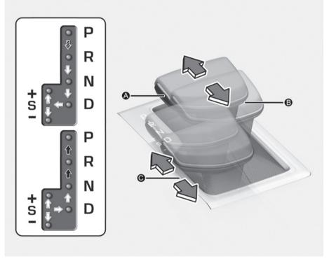
[A] Shift lever[B] Shift release button[C] Manual shift mode
