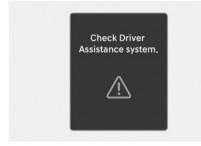
When Lane Following Assist is not working properly, the "**Check Driver Assistance system.**" warning message will appear on the instrument cluster for several seconds, and the master (A) warning light appears on the instrument cluster. If this occur, have your vehicle inspected by an authorized HYUNDAI dealer.
