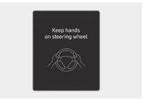
If the driver takes their hands off the steering wheel for several seconds, the '**Keep hands on steering wheel**' warning message appears on the instrument cluster, and an audible warning sounds in stages.
