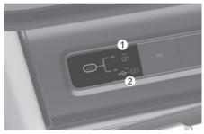
Press the USB port selection button while the vehicle is running. Press the upper portion of the button (1) to charge an electronic device. Press the lower portion of the button (2) to charge and listen to music with a media storage device. The USB port can be used after either indicator light turns on.
