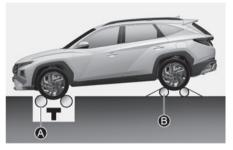
[A] Roll tester (Speedometer)[B] Temporary free roller
