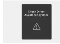
When Driver Attention Warning is not working properly, the "**Check Driver Assistance system**" warning message will appear on the cluster for several seconds, and the master (企) warning light and the inattentive driving (逆) warning light will appear on the instrument cluster. If this occurs, have your vehicle inspected by an authorized HYUNDAI dealer.
