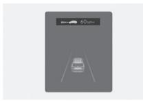
The current operation condition of Manual Speed Limit Assist, Smart Cruise Control, Lane Following Assist, etc. appears.
