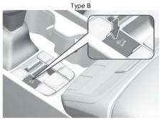
Downhill Brake Control assists when descending down a steep hill without having to depress the brake pedal.
