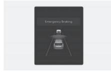
To warn the driver that emergency braking will be assisted, the '**Emergency Braking**' warning message will appear on the cluster, an audible warning will sound and the steering wheel will vibrate.
