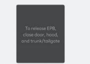
If the hood, liftgate, doors are open, and you try to drive with EPB applied, a warning sounds and a message appears.
