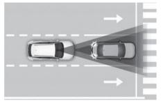
Forward Collision-Avoidance Assist uses the front view camera and front radar to help detect a vehicle, a powered two-wheeler, a pedestrian, or a cyclist ahead on the road. The function may warn you with a warning message on the instrument cluster and an audible warning if a collision is imminent. If necessary, it may assist with braking your vehicle to help reduce collision speed and avoid a collision.
