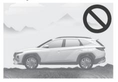
Remote Smart Parking Assist may cancel when the vehicle slips, or the vehicle cannot move due to road conditions such as pebbles or fragmented stones. • Parking behind a truck
