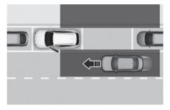
While your vehicle is stopped, and if Safe Exit Warning detects a vehicle approaching the rear corner of your vehicle and a passenger opens a door, Safe Exit Warning may warn you with a warning message and a warning sound to help avoid a collision.
