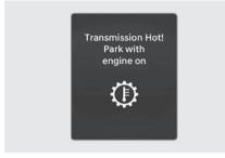
Repeated sudden acceleration and quick start may overheat the transmission. If the transmission is overheated, the self protection mode alarms the driver with an audible sound warning message.
