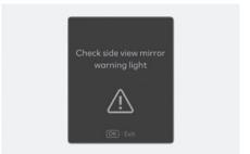
When the side view mirror warning light is not working properly, the "**Check side view mirror warning light**" warning message will appear on the instrument cluster for several seconds, and the master warning light ( $\triangle$ ) will appear on the instrument cluster. If this occurs, have your vehicle inspected by an authorized HYUNDAI dealer.
