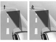
Forward Collision-Avoidance Assist may not detect other vehicles, powered two-wheelers, pedestrians or cyclists in front of you when driving on curved roads adversely affecting the performance of the sensors. This may result in no warning, braking assist or steering assist (if equipped) when necessary.
