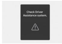
When Forward Collision-Avoidance Assist is not working properly, the "**Check Driver Assistance system.**" warning message will appear, and the (⚠) or (♣) warning lights will illuminate on the cluster display. Have the vehicle inspected by an authorized HYUNDAI dealer.
