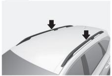
Your vehicle may come equipped with roof side rails. If your vehicle is equipped with roof side rails, you can add roof rack crossbars as an accessory (not shown).
