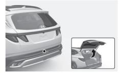
When the liftgate is closed, press the power liftgate open/close button to open the liftgate.
