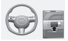
Press the **IID** switch to temporarily pause the set speed limit. The set speed limit will turn off but the Speed Limit ((CLIMIT) indicator will stay on.
