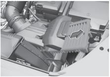
4. Reassemble the air cleaner filter cover in the reverse order.
