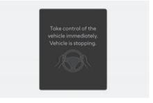
To warn you that Emergency Stop is operating the '**Take control of the vehicle immediately. Vehicle is stopping.**' warning message appears on the instrument cluster, an audible warning sounds, and the steering wheel vibrates.
