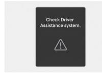
When Smart Cruise Control is not working properly, the "**Check Driver Assistance system.**" warning message will appear, and the ( $\triangle$ ) warning light will illuminate on the instrument cluster. Have your vehicle inspected by an authorized HYUNDAI dealer.
