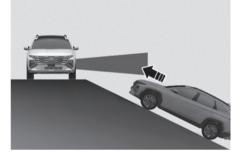
Rear Cross-Traffic Collision-Avoidance Assist may be limited when the vehicle is on a uphill or downhill slope, or near it, and may not detect the vehicle approaching from the left or right. If this occurs, the function may not warn the driver or control the brakes when necessary.
