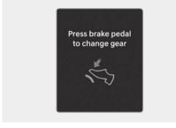
This message appears when the brake pedal is not depressed while shifting the gear.
