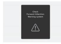
When Forward Attention Warning is not working properly, the "Check Forward Attention Warning system" warning message will appear on the cluster. If this occurs, have the vehicle inspected by an authorized HYUNDAI dealer.
