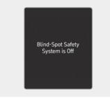
When the vehicle is restarted with Blind-Spot Collision-Avoidance Assist off, the "**Blind-Spot Safety System is Off**" message will appear on the instrument cluster. If you select "**Blind-Spot Safety**", warning light on the side view mirror will blink for three seconds. In addition, if the vehicle is turned on, when "**Blind-Spot Safety**" is selected, the warning light on the side view mirror blinks for three seconds.
