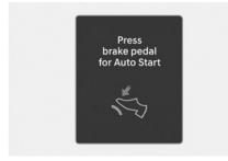
When the gear is shifted from N (Neutral) to R (Reverse), D (Drive), or Manual shift mode without the brake pedal depressed, a message appears on the cluster display. To activate auto start, depress the brake pedal.
