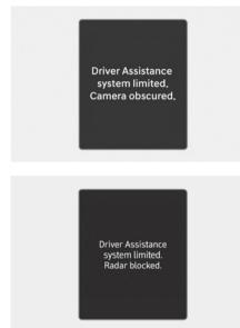
When the front windshield where the front view camera is located, front radar cover, bumper (if equipped) or sensor is covered with foreign material, such as snow or rain, it can reduce the detecting performance and temporarily limit or disable Forward Collision-Avoidance Assist.
