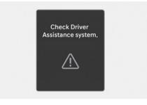
When Rear Cross-Traffic Collision-Avoidance Assist is not working properly, the "**Check Driver Assistance system.**" warning message appears on the instrument cluster for several seconds, and the master (A) warning light illuminates on the instrument cluster. If this occur, have vehicle inspected by an authorized HYUNDAI dealer.
