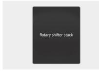
This message appears when the rotary gear shift dial does not return back to it's normal position after rotating it.
