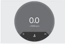
The engine coolant temperature gauge indicates the temperature of the engine coolant when the Engine Start/Stop button is in the ON position.
