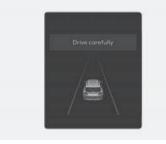
• When the vehicle is stopped due to emergency braking, the "**Drive carefully**" warning message will appear on the instrument cluster.
