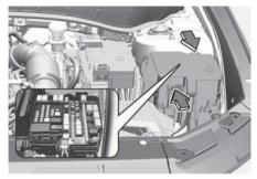
Inside the fuse panel cover, you can find the label describing fuse names and ratings.
