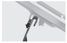
5. With the Engine Start/Stop button in the ON position, turn the wiper switch to any ON position to return the wipers to the bottom resting position.
