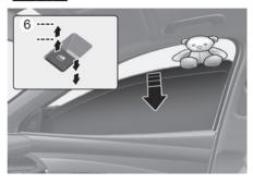
If a window senses any obstacle while it is closing automatically, it stops and lowers approximately 12 in. (30 cm) to allow the object to be cleared.
