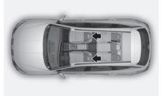
The driver's and front passenger's seats are equipped with adjustable head restraint for the passengers safety and comfort.
