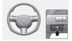
Press the button repeatedly to cycle through the headway settings from **Distance 4 > Distance 3 > Distance 2 > Distance 1 > Distance 4**.
