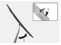
3. Lift up the wiper blade clip (1). Then pull down the wiper blade (2).
