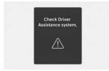
When Safe Exit Warning is not working properly, the "**Check Driver Assistance system.**" warning message will appear on the instrument cluster for several seconds, and the master warning light (<u>A</u>) will appear on the instrument cluster. If this occurs, have your vehicle inspected by an authorized HYUNDAI dealer.
