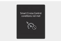
If the Driving Assist button, + switch, switch or **IIO** switch is operated when Smart Cruise Control operating conditions are not satisfied, the **"Smart Cruise Ctrl. conditions not met**" will appear on the instrument cluster, and an audible warning will sound.
