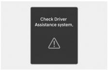
When Reverse Parking Collision-Avoidance Assist or other related functions are not working properly, the "**Check Driver Assistance system.**" warning message appears on the instrument cluster, and Reverse Parking Collision-Avoidance Assist turns off automatically. Have your vehicle inspected by an authorized HYUNDAI dealer.
