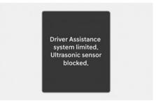
If this occurs the "**Driver Assistance** system limited. Ultrasonic sensor blocked." warning message appears on the instrument cluster. Parking Distance Warning operates properly when snow, rain or foreign material is removed. If Parking Distance Warning does not operate properly after obstruction (snow, rain, or foreign material) is removed (including trailer, carrier, etc., from the rear bumper), have your vehicle inspected by an authorized HYUNDAI dealer.
