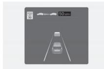
Manual Speed Limit Assist or Smart Cruise Control assists the vehicle to adjust its speed according to the speed limit. When the cruising speed is set as same as the speed limit, the vehicle automatically adjusts its speed if the speed limit changes. The function operates on the road which has a speed limit of 44 mph (70 km/h) or higher. When the function is active, the cruising speed on the instrument cluster appears in green.
