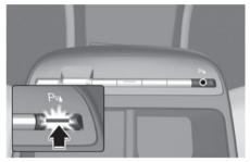
Press and hold the Parking Safety ( $P_{W}$ ) button more than 2 seconds, to turn the Parking Collision-Avoidance Assist on or off.
