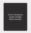
When the front radar cover or sensor is covered with snow, rain, or foreign material, it can reduce the detecting performance and temporarily limit or disable Smart Cruise Control.
