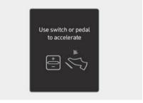
When Highway Driving Assist is operating, your vehicle will stop if the vehicle ahead of you stops. Also, if the vehicle ahead of you starts moving within 30 seconds after the stop, your vehicle will start as well. In addition, after the vehicle has stopped and 30 seconds have passed, the "**Use switch or pedal to accelerate**" message will appear on the instrument cluster. Depress the accelerator pedal or operate the + switch, - switch or **IIO** switch to start driving.
