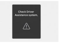
When Forward Collision-Avoidance Assist is not working properly, the "**Check Driver Assistance system.**" warning message will appear, and the (企) or (左) warning lights will illuminate on the instrument cluster. Have your vehicle inspected by an authorized HYUNDAI dealer.
