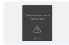
When the side view mirror warning light is not working properly, the "**Check side view mirror warning light**" warning message appears on the instrument cluster for several seconds, and the master (**A**) warning light illuminates on the instrument cluster. If this occur, have your vehicle inspected by an authorized HYUNDAI dealer.
