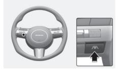
• Whenever the vehicle is turned on, Lane Keeping Assist always turn on, and the grey or green (/⊕\) indicator light illuminates on the cluster.
