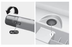
The headlights and parking lights are turned ON or OFF automatically depending on the amount of daylight as measured by the ambient light sensor (1) in front of the instrument panel.
