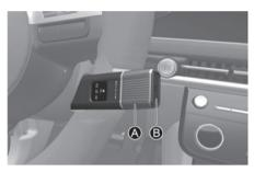
[A] Rotary gear shift dial[B] P button
