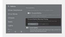
With the vehicle on, select **Setup** > **Vehicle** > **Driver Assistance** > **Driving Safety** > **Forward Safety Warning Timing** settings menu in the infotainment system to change the initial warning activation time for Forward Collision-Avoidance Assist. The warning time can be set to either **Standard** or Late.
