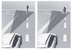
Forward Collision-Avoidance Assist may detect a vehicle, pedestrian or cyclist in the next lane or outside the lane when driving on a curved road.
