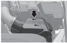
The air cleaner filter can be cleaned for inspection using compressed air. Do not attempt to wash or rinse it, because water can damage the filter. If soiled, replace the air cleaner filter.
