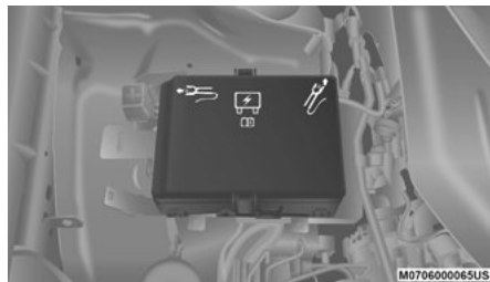
Front Power Distribution Center
