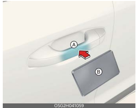
[A]: Door handle authentication pad, [B]: Card key NFC antenna
