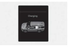
The engine charges the high voltage battery according to the vehicle and surrounding conditions.
