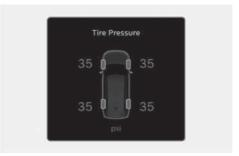
• You can check the tire pressure in the utility view mode in the cluster display. Refer to the "View modes" section in chapter 4.
