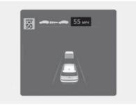
When driving at a speed higher than the displayed speed limit, the speed limit is displayed in red.
