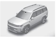
The front view camera is mounted near the top of the windshield inside your vehicle.
