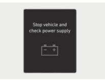
This message appears when a failure occurs in the power supply system. If this occurs, have your vehicle inspected by an authorized HYUNDAI dealer.
