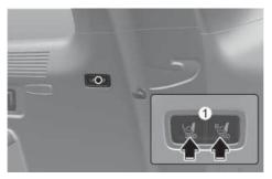
With the liftgate open, this feature allows you to conveniently fold the 2nd row seatback forward.
