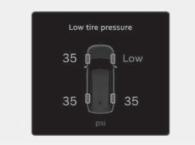
This warning message appears if the tire pressure is low. The corresponding tire on the vehicle is illuminated.
