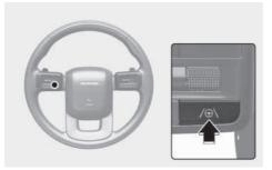
• With the engine on, press and hold the Lane Driving Assist button (/⊕\) located on the steering wheel to turn on Lane Keeping Assist. The (/=\) indicator light illuminates on the instrument cluster.
