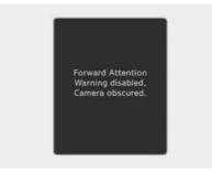
When there is an object right in front of the in-cabin camera or between the driver and the camera for a certain period of time, Forward Attention Warning does not operate properly, and the "Forward Attention Warning disabled. Camera obscured" warning message appears on the instrument cluster, and an audible warning sounds.
