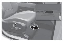
The hybrid battery cooling duct is located below the passenger seat. The cooling duct cools down the hybrid battery. When the hybrid battery cooling duct is blocked, the hybrid battery may be overheated.
