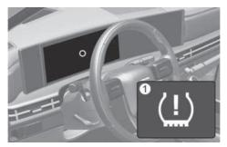
The TPMS Malfunction Indicator illuminates after it blinks for about one minute when there is a problem with the Tire Pressure Monitoring System. Have the system inspected by an authorized HYUNDAI dealer as soon as possible.
