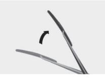
3. Lift up the wiper blade clip (1). Then pull down the wiper blade (2). Remove the wiper blade from the wiper arm.
