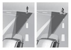
Forward Collision-Avoidance Assist may detect a vehicle, powered twowheeler, pedestrian or cyclist in the next lane or outside the lane when driving on a curved road.
