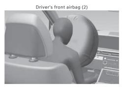
Upon deployment, tear seam in the pad cover separates from the expansion of the airbags.
