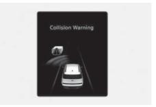
• To warn the driver of a collision, Forward Safety warning light (♣) blinking, the "**Collision Warning**" warning message will appear on the cluster, an audible warning will sound, and the steering wheel will vibrate.
