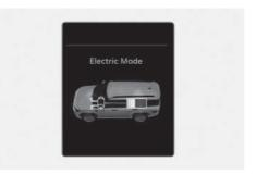
Only the motor power is used to drive the vehicle. (Battery  $\rightarrow$  Wheel)
