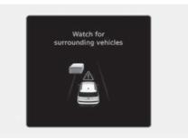
In the following situation, the "**Watch for surrounding vehicles**" warning message will appear on the instrument cluster, and an audible warning will sound to warn the driver of road conditions ahead.
