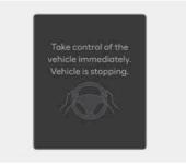
To warn you that Emergency Stop is operating the "**Take control of the vehicle immediately. Vehicle is stopping.**" warning message appears on the instrument cluster, an audible warning sounds, and the steering wheel vibrates.
