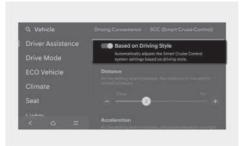
Smart Cruise Control operates based on your driving style, such as vehicle distance, acceleration, and reaction speed.
