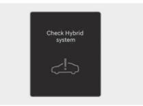
This message appears when there is a problem with the hybrid control system. Refrain from driving when the warning message appears.
