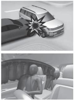
Side and curtain airbags are designed to inflate when an impact is detected by side collision sensors depending on the severity of impact resulting from a side impact collision.
