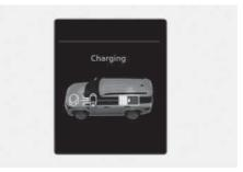
The engine and regenerative brake system charges up the high voltage battery. (Engine and Wheel  $\rightarrow$  Battery)
