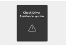
When Smart Cruise Control is not working properly, the "**Check Driver Assistance system.**" warning message will appear, and the "A" warning light will illuminate on the instrument cluster. Have your vehicle inspected by an authorized HYUNDAI dealer.
