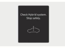
This message appears when there is a problem with the hybrid control system. The READY indicator will blink and a warning chime will sound until the problem is solved. Refrain from driving when the warning message appears.
