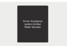
When the rear bumper around the rear corner radar or sensor is covered with foreign material, such as snow or rain, or installing a trailer or carrier, it can reduce the detecting performance and temporarily limit or disable Safe Exit Assist.
