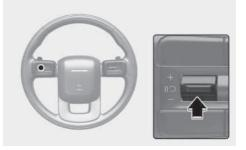
Press the **IID** switch to temporarily pause the set speed limit. The set speed limit will turn off but the Speed Limit (SCLIMIT) indicator will stay on.
