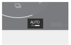
The smart regeneration system is ON and the regenerative braking level appears as "**AUTO**".
