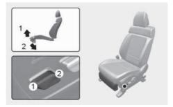
Push the control switch forward (1) to raise the leg support. Push the control switch rearward (2) to lower the leg support.
