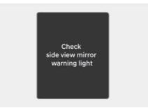
When the side view mirror warning light is not working properly, the "**Check** side view mirror warning light" warning message will appear on the instrument cluster for several seconds, and the master ( $\triangle$ ) warning light will illuminate on the instrument cluster. If this occurs, have your vehicle inspected by an authorized HYUNDAI dealer.
