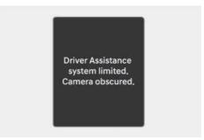
When the front windshield where the front view camera is located is covered with foreign material, such as snow or rain, it can reduce the detecting performance and temporarily limit or disable Driver Attention Warning.
