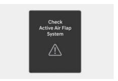
The active air flap system may not operate normally if the air flap is temporarily opened due to foreign factors or if the controller is contaminated by snow or rain, etc.
