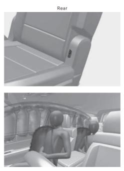
The side airbags are designed to deploy during certain side impact collisions, depending on the crash severity.
