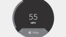
The speedometer indicates the speed of the vehicle and is calibrated in miles per hour (MPH) and/or kilometers per hour (km/h).
