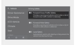
With the engine on, select **Setup** > **Vehicle** > **Driver Assistance** > **Forward Cross-Traffic Safety** in the infotainment system to turn on Junction Crossing function and deselect to turn off the function.
