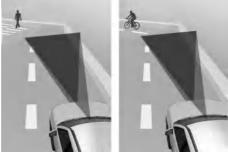
Forward Collision-Avoidance Assist may not detect other vehicles, powered two-wheelers, pedestrians or cyclists in front of you when driving on curved roads adversely affecting the performance of the sensors. This may result in no warning, braking assist or steering assist (if equipped) when necessary.
