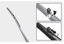
4. Install a new wiper blade assembly in the reverse order of removal.
