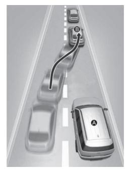
When a vehicle moves into your lane from an adjacent lane, it cannot be detected by the sensor until it is in the sensor's detection range. The smart regeneration system may not immediately detect the vehicle when your vehicle changes lanes abruptly.
