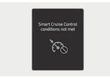
If the Driving Assist button, + switch, - switch or **II'D** switch is operated when Smart Cruise Control operating conditions are not satisfied, the **"Smart Cruise Ctrl. conditions not met**" will appear on the instrument cluster, and an audible warning will sound.
