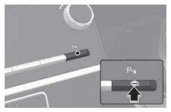
Press the Parking Safety (P™) button to turn on Forward/Reverse Parking Distance Warning. Press the button again to turn off the function.
