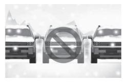
Snow may interfere with sensor operation, or Remote Smart Parking Assist may cancel if the road is slippery while parking.
