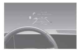
The Head-Up Display is an optional feature that allows the driver to view information projected onto a transparent screen while still keeping your eyes on the road ahead while driving.
