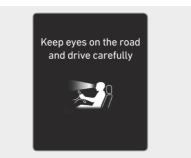
Forward Attention Warning determines whether the driver is focused on the road depending on information, such as the amount of time the driver is looking elsewhere, the amount of time the eyes are closed, how frequently the driver yawns, etc. If Forward Attention Warning judges the driver is not focused, the "**Keep eyes on the road and drive carefully**" warning message will appear on the cluster, and an audible warning will sound.
