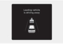
When a detected vehicle in front departs from a stop, Leading Vehicle Departure Alert will inform the driver by displaying the "**Leading vehicle is driving away**" message on the instrument cluster and an audible warning will sound.
