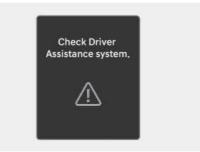
When Safe Exit Assist is not working properly, the "**Check Driver Assistance system.**" warning message appears on the instrument cluster for several
