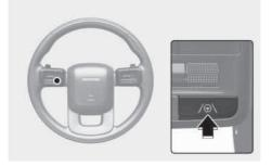
With the engine on, shortly press the Lane Driving Assist button located on the steering wheel to turn on Lane Following Assist. The gray or green ( $\Theta$ ) indicator light will illuminate on the instrument cluster.
