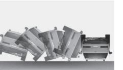
Front airbags may not inflate in rollover crash because front airbag deployment would not provide additional occupant protection.
