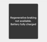
Regenerative braking is temporarily limited to protect the battery because the high voltage battery is fully charged.
