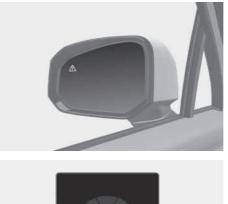
• When an approaching vehicle from the rear is detected at the moment a door is opened, the "**Collision Warning**" warning message appears on the instrument cluster, and an audible warning sounds.
