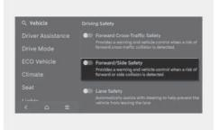
With the engine on, select **Setup** > **Vehicle** > **Driver Assistance** > **Forward/Side Safety** in the infotainment system to set whether to use each function.
