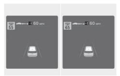
If the speed limit of the road changes during the operation of Manual Speed Limit Assist or Smart Cruise Control, an arrow in the direction of up or down is displayed to inform the driver that the set speed needs to be changed. At this time, the driver can change the set speed according to the speed limit by using the + or - switch on the steering wheel.
