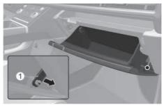
2. Push in both sides of the glove box to release the glove box stopper pins and allow the glove box to hang open.
