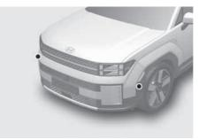
These ultrasonic sensors are mounted near the front wheels outside your vehicle.
