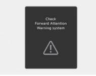
When Forward Attention Warning is not working properly, the "**Check Forward Attention Warning system**" warning message will appear on the cluster. If this occurs, have the vehicle inspected by an authorized HYUNDAI dealer.
