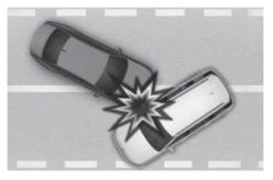
In an angled collision, the force of impact may position the occupants in a direction where the airbags would not be able to provide any additional benefit, and thus the sensors may not deploy any airbags.
