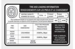
The label located on the driver's door jamb shows the original tire size, cold tire pressures recommended for your vehicle, the number of people that can be in your vehicle and vehicle capacity weight.
