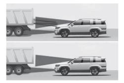
If the vehicle in front of you has cargo that extends rearward from the cab, or when the vehicle in front of you has higher ground clearance, additional special attention is required. Forward Collision-Avoidance Assist may not be 506 able to detect the cargo extending from the vehicle. In these instances, you must maintain a safe braking distance from the rearmost object, and if necessary, steer your vehicle and depress the brake pedal to reduce your driving speed in order to maintain distance.
