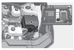
High voltage cut-off switch is a device located inside the engine compartment to block the battery's high voltage when your vehicle is inspected at an authorized HYUNDAI dealer.
