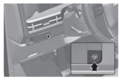
Press the Tow mode button to turn on or off the function.
