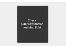
When the side view mirror warning light is not working properly, the "**Check** side view mirror warning light" warning message appears on the instrument cluster for several seconds, and the master ( $\triangle$ ) warning light illuminates on the
