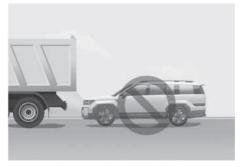
Do not use Remote Smart Parking Assist around vehicles with higher ground clearance, such as a bus, truck, etc. It may lead to a collision.
