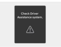
When Lane Keeping Assist is not working properly, the "**Check Driver Assistance system.**" warning message appears, the master ( $\triangle$ ) warning light and the yellow Lane Safety ( $\frown$ ) indicator light illuminates on the instrument cluster. If this occurs, have your vehicle inspected by an authorized HYUNDAI dealer.
