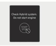
This message appears when the hybrid battery power (SOC) level is low. A warning chime will sound until the problem is solved. Refrain from driving when the warning message appears.
