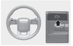
To turn Smart Cruise Control off, press the Driving Assist ( ) button.
