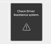
When Reverse Parking Collision-Avoidance Assist or other related functions are not working properly, the "**Check Driver Assistance system.**" warning message appears on the instrument cluster, and Reverse Parking Collision-Avoidance Assist turns off automatically. Have your vehicle inspected by an authorized HYUNDAI dealer.
