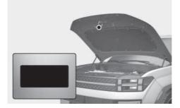
You can find out which air conditioning refrigerant is applied to your vehicle on the label located inside of the hood.
