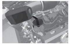
Use only the specified engine oil (Refer to the "Recommended lubricants and capacities" section in chapter 10).
