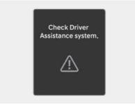
When Rear Cross-Traffic Collision-Avoidance Assist is not working properly, the "Check Driver Assistance system." warning message appears on the instrument cluster for several seconds, and the master ( $\triangle$ ) warning light illuminates on the instrument cluster. If this occur, have vehicle inspected by an authorized HYUNDAI dealer.
