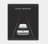
• When the vehicle is stopped due to emergency braking, the "Drive carefully" warning message will appear on the instrument cluster.
