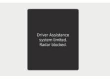
When the rear bumper around the rear corner radar or sensor is covered with foreign material, such as snow or rain, or installing a trailer or carrier, it can reduce the detecting performance and temporarily limit or disable Blind-Spot Collision-Avoidance Assist.
