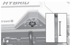
7. If the oil level is below the L, add enough oil to bring the level to F.
