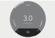
This gauge indicates the remaining hybrid battery power. If the SOC is near the L (Low) level, the vehicle automatically operates the engine to charge the battery.
