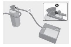
3. Unscrew the valve cap from the valve of the defective wheel and screw the filling hose (3) of the sealant bottle onto the tire valve.
