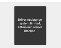
If this occurs the "**Driver Assistance system limited. Ultrasonic sensor blocked.**" warning message appears on the instrument cluster. Parking Distance Warning operates properly when snow, rain or foreign material is removed. If Parking Distance Warning does not operate properly after obstruction (snow, rain, or foreign material) is removed (including trailer, carrier, etc., from the rear bumper), have your vehicle inspected by an authorized HYUNDAI dealer.
