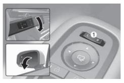
When the gear is shifted to the R (Reverse) position, the side view mirrors rotate downwards to aid with driving in reverse.
