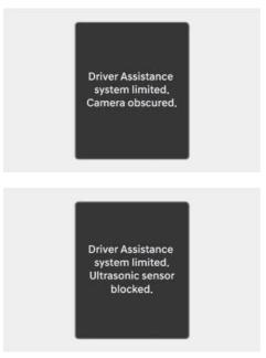
The "Driver Assistance system limited. Camera obscured." or "Driver Assistance system limited. Ultrasonic sensor blocked." warning message appears on the instrument cluster if the following situations occur:
