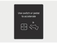
In traffic, your vehicle will stop if the vehicle ahead of you stops. Also, if the vehicle ahead of you starts moving, your vehicle will start as well. In addition, after the vehicle has stopped and a certain time have passed, the "**Use switch or pedal to accelerate**" message will appear on the instrument cluster. Depress the accelerator pedal or operate the + switch, - switch or **IIO** switch to start driving.
