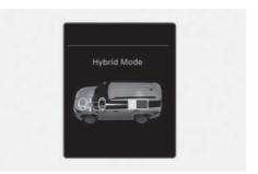
Both the motor and the engine power are used to drive the vehicle. (Battery & Engine  $\rightarrow$  Wheel)
