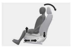
Relaxation comfort seats help distribute body pressure and concentrated weight on specific body parts that occur while sitting in the same position for a long period of time. The seat helps relieve fatigue and discomfort by providing the optimal sit position.
