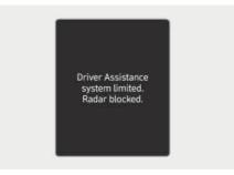
When the front windshield where the front view camera is located, front radar cover, bumper (if equipped) or sensor is covered with foreign material, such as snow or rain, it can reduce the detecting performance and temporarily limit or disable Forward Collision-Avoidance Assist.
