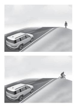
Forward Collision-Avoidance Assist may not detect other vehicles, powered two-wheelers, pedestrians or cyclists in front of you while driving uphill or downhill, adversely affecting the performance of the sensors.
