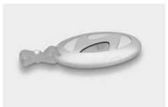
You can start the vehicle using the Remote Start ( ) button on the smart key. To start the vehicle remotely:
