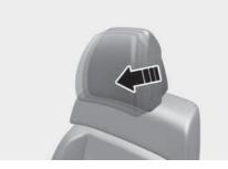
The head restraint may be adjusted forward to 3 different positions by pulling the head restraint forward to the desired detent. To adjust the head restraint to it's furthest rearwards position, pull it fully forward to the farthest position and release it.
