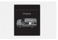
The high voltage battery is charged up by the regenerative brake system. (Wheel  $\rightarrow$  Battery)
