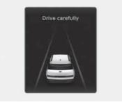
• When the vehicle is stopped due to emergency braking, the "Drive carefully" warning message will appear on the cluster.
