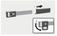
Turn the knob (2) of the mechanical key after removing the key protector (1). After using the mechanical key, turn the key knob (2) and insert the key protector (1).
