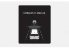
To warn the driver that emergency braking will be assisted, Forward Safety warning light (♣) blinking, the "**Emergency Braking**" warning message will appear on the cluster, an audible warning will sound, and the steering wheel will vibrate.
