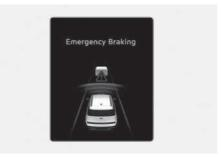
• To warn the driver that emergency braking will be assisted, Forward Safety warning light (♣) blinking, the "**Emergency Braking**" warning message will
