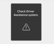
When Forward Collision-Avoidance Assist is not working properly, the **Check Driver Assistance system.** warning message will appear, and the  $\Delta$ ,  $\leq$ , or  $\leq$  warning lights will illuminate on the instrument cluster. Have your vehicle inspected by an authorized HYUNDAI dealer.
