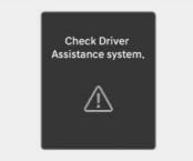
When Blind-Spot Collision-Avoidance Assist is not working properly, the "**Check Driver Assistance system.**" warning message will appear on the instrument cluster for several seconds, and the master ( $\underline{\Lambda}$ ) warning light will appear on the instrument cluster. If this occurs, have your vehicle inspected by an authorized HYUNDAI dealer.
