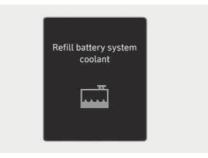
This message appears when the battery system coolant is nearly empty. You should refill the battery system coolant.
