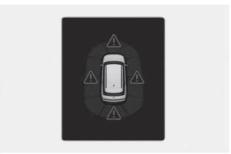
When the Parking Distance Warning is operating, if the function is not working normally or the ultrasonic sensor is blocked, the master warning light ( $\triangle$ ) appears in the direction of the corresponding sensor. You can check the warning in the Utility view on the cluster.
