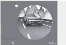
Blind-Spot View Monitor uses the wide-side view cameras to display the rear blind spot areas of your vehicle on the instrument cluster when the turn signal is turned on to help with safe lane changes.
