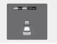
If you want to speed up temporarily without altering the set speed while Smart Cruise Control is operating, depress the accelerator pedal. While the accelerator pedal is depressed, the set speed, distance level and target distance will blink on the instrument cluster.
