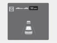
Manual Speed Limit Assist or Smart Cruise Control assists the vehicle to adjust its speed according to the speed limit. When the cruising speed is set as same as the speed limit, the vehicle automatically adjusts its speed if the speed limit changes. The function operates on the road which has a speed limit of 45 mph (70 km/h) or higher. When the function is active, the cruising speed on the instrument cluster appears in green.
