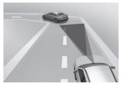
On curves, Smart Cruise Control may not detect a vehicle in the same lane, and may accelerate to the set speed. Also, vehicle speed may rapidly decrease when the vehicle ahead is detected suddenly.
