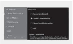
With the engine on, select or deselect **Setup** > **Vehicle** > **Driver Assistance** > **Speed Limit** from the infotainment system to set whether to use each function.
