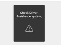
When Intelligent Speed Limit Assist is not working properly, the "**Check Driver Assistance system.**" warning message will appear on the instrument cluster for several seconds, and the master ( $\triangle$ ) warning light and ( $\square$ ) warning light will illuminate on the instrument cluster. If this occurs, have your vehicle inspected by an authorized HYUNDAI dealer.
