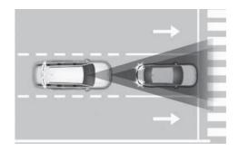
Forward Collision-Avoidance Assist uses the front view camera and front radar to help detect a vehicle, a pedestrian, or a cyclist ahead on the road. The function may warn you with a warning message on the instrument cluster and an audible warning if a collision is imminent. If necessary, it may assist with braking your vehicle to help reduce collision speed and avoid a collision.
