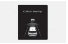
While Smart Cruise Control is operating, when the collision risk with the vehicle ahead is high, the "**Collision Warning**" warning message will appear on the instrument cluster, an audible warning will sound, and the steering wheel will vibrate to warn the driver. Always have your eyes on the road while driving, and if necessary, depress the brake pedal to reduce your driving speed in order to maintain a safe distance.
