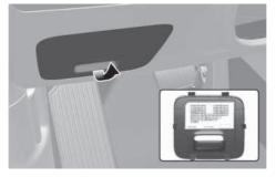
Inside the fuse panel cover, you can find the label describing fuse names and ratings.
