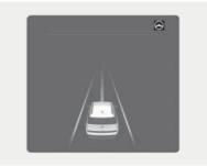
If the vehicle ahead and/or both lane markings are detected and your vehicle speed is below 110 mph (180 km/h), the green  $(\Theta)$  indicator light appears on the cluster, and Lane Following Assist helps center the vehicle in the lane by assisting the steering wheel.
