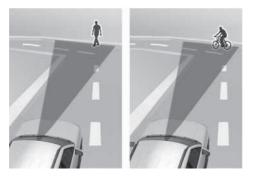
On curves, the smart regeneration system may not detect a vehicle in the same lane, and may accelerate the vehicle by lowering the regenerative braking intensity automatically. Your vehicle speed may decelerate by increasing regenerative braking intensity automatically if a vehicle is detected in an adjacent lane or when a vehicle ahead is detected suddenly. Apply the brake pedal or accelerator pedal depending on the road and driving conditions. Driving on hills
