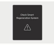
If the rear radar is covered by any foreign material, such as snow, rain, or dirt, the detecting performance may decrease and disable the smart regeneration system.
