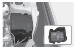
Inside the fuse panel cover, you can find the label describing fuse names and ratings.
