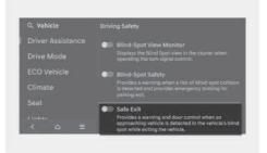
With the engine on, select **Setup** > **Vehicle** > **Driver assistance** > **Driving Safety** > **Safe Exit** from the Settings menu to turn on Safe Exit Assist and deselect to turn off the function.
