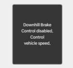
If Downhill Brake Control is not working properly, this warning message appears on the cluster display and you may hear a warning sound. If this occurs, control the vehicle speed by depressing the brake pedal.
