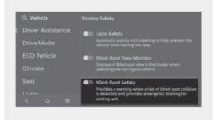
With the engine on, select **Setup** > **Vehicle** > **Driver Assistance** > **Driving Safety** > **Blind-Spot Safety** in the infotainment system to set whether to use each function.
