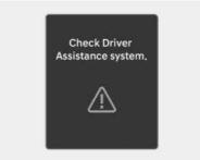
When Driver Attention Warning is not working properly, the "**Check Driver Assistance system.**" warning message will appear on the cluster for several seconds, and the master ( $\triangle$ ) warning light and the driver's attention (D) warning light will appear on the instrument cluster. If this occurs, have your vehicle inspected by an authorized HYUNDAI dealer.
