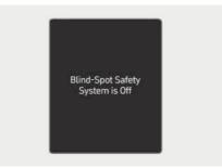
When the vehicle is restarted with Blind-Spot Collision-Avoidance Assist off, the "Blind-Spot Safety System is Off" message will appear on the instrument cluster.
