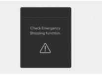
When Emergency Stop is not working properly, the "**Check Emergency Stopping function.**" warning message appears, and the master ( $\triangle$ ) warning light illuminates on the instrument cluster. If this occurs, have your vehicle inspected by an authorized HYUNDAI dealer.
