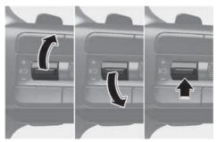
To resume Manual Speed Limit Assist after the function was paused, operate the +, -, IIO switch.
