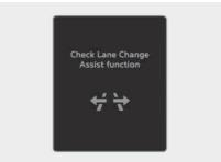
When Highway Driving Assist is not working properly, the "**Check Driver** Assistance system." or "**Check Lane Change Assist function**" warning message and Master ( $\underline{\Lambda}$ ) warning light appears on the instrument cluster. If this occurs, have your vehicle inspected by an authorized HYUNDAI dealer.
