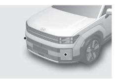
The front corner radars are mounted near the front corners of your vehicle above.
