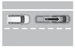
If the vehicle in front abruptly departures, Leading Vehicle Departure Alert may not operate properly.
