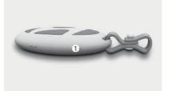
2. Remove the old battery and insert a new battery. Make sure the battery position is correct. An improperly positioned battery may discharge the battery, causing smart key failure.
