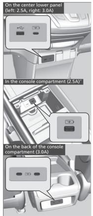
■ USB charging/connector port ( ← ← ) The USB port (2.5A) is for charging devices, playing audio files, and connecting compatible phones with Apple CarPlay or Android Auto.
