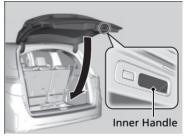
When all the doors are unlocked or press the tailgate unlock button<sup>\*</sup> on the remote transmitter, the tailgate is unlocked.
