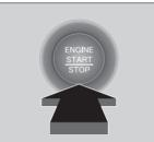
If you carry the keyless remote and press **ENGINE START/STOP** button without depressing the brake pedal, the power mode will change in this order: VEHICLE OFF $\rightarrow$ ACCESSORY $\rightarrow$ ON $\rightarrow$ VEHICLE OFF.
