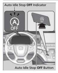
To turn the Auto Idle Stop system off, press this button. The Auto Idle Stop system stops.
