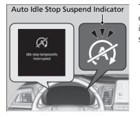
The Auto Idle Stop suspend indicator comes on and a message appears on the driver information interface when the Auto Idle Stop system cannot be activated.
