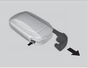
1. Remove the built-in key.
