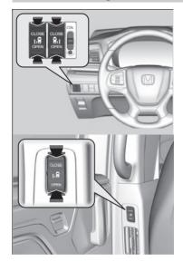
The power sliding door opens when you press the **OPEN** side of the  $[\underline{1,0}] / [\underline{0,1}]$  switch, and closes when you press the **CLOSE** side of the  $[\underline{1,0}] / [\underline{0,1}]$  switch.
