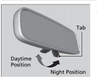
Flip the tab to switch the position. The night position will help reduce the glare from headlights behind you when driving after dark.
