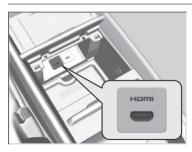
There is an HDMI<sup>™</sup> port in the console compartment. The rear entertainment system will accept HDMI<sup>™</sup> cable connections with video equipment that is equipped with an HDMI<sup>™</sup> port.
