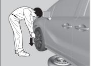
**8.** Loosen each wheel nut about one turn using the wheel nut wrench.
