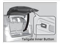
Press the tailgate inner button on the tailgate to close the power tailgate. ► The beeper sounds.
