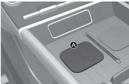
[A] Vehicle authentication pad (Wireless charging pad)
