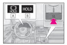
Turns the brake hold system on
