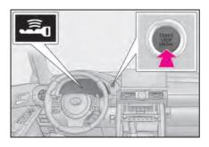
4 Press the engine switch shortly and firmly.
