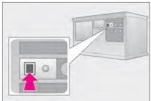
Locate the "Learn" or "Smart" button on the garage door opener motor in the garage.
