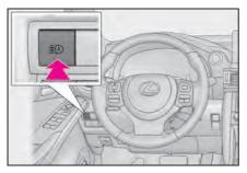
Press the Automatic High Beam switch.
