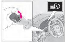
1 Press the Automatic High Beam switch.
