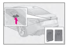
While carrying the electronic key, press the button on the trunk lid.
