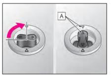
2 Turn the upper knob of each retaining hook (clip) to secure the floor mats in place.
