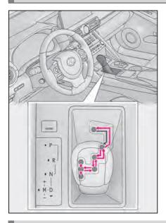
While the engine switch is in IGNI-TION ON mode, move the shift lever with the brake pedal depressed.
