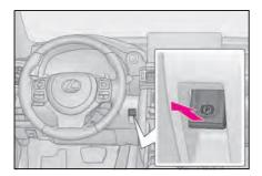
While the vehicle is stopped, pull and hold the parking brake switch until "EPB Shift Interlock Function Deactivated" will be displayed on the multi-information display.
