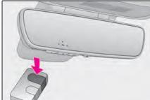
Point the remote control transmitter for the device at the rear view mirror, 1 to 3 in. (25 to 75 mm) from the HomeLink<sup>®</sup> buttons.
