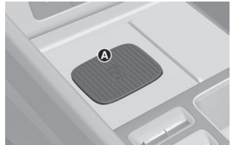
[A] Vehicle authentication pad (wireless charging pad)
