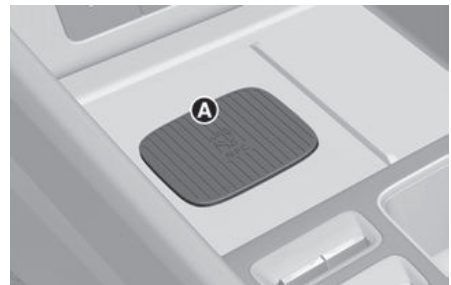
[A] Vehicle authentication pad (Wireless charging pad)
