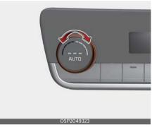
Press the temperature control button and turn the temperature control switch to the desired temperature.
