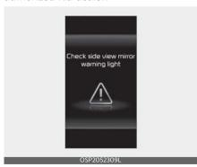
When the warning light on the side view mirror (outside mirror) is not working properly, the warning message will appear for several seconds and the varning light will appear on the cluster.
