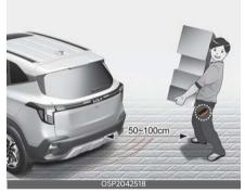
If you are positioned in the detecting area (50 ~ 100 cm (20 ~ 39 inches) behind the vehicle) carrying a smart key, the hazard warning lights will blink and chime will sound for about 3 seconds to alert you the smart key has been detected and the liftgate will open.
