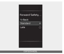
With the ignition switch or ENGINE START/STOP button in the ON position, select User Settings → Driver Assistance → Driving Safety → Forward Safety Warning Timing on the LCD display or Setup → Vehicle → Driver Assistance → Driving Safety → Forward Safety Warning Timing on the Infotainment system screen to change the initial warning activation timing for Forward Collision-Avoidance Assist.
