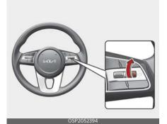
Push up the + switch, and release it immediately. The set speed will increase by 1 km/h (1 mph) each time the switch is operated in this manner.
