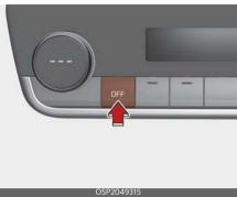
Press the OFF button to turn off the front and rear air climate control system.
