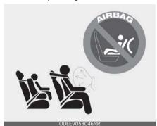
If the air bag deploys, it would impact the rear-facing child restraint, causing serious or fatal injury.
