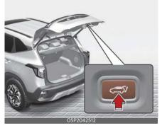
Press the power liftgate open/close button. The liftgate opens or closes with a warning sound.
