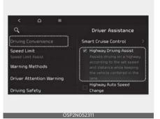
With the ignition switch or ENGINE START/STOP button in the ON position, select **Setup** → **Vehicle** → **Driver Assistance** → **Driving Convenience** → **Highway Driving Assist** on the Infotainment system screen to set whether to use the function.
