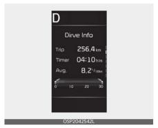
The trip computer mode displays information related to vehicle driving parameters including fuel economy, tripmeter information and total driving time.
