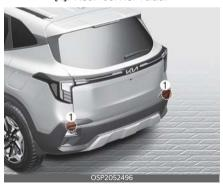
Refer to the picture for the detailed location of the detecting sensors.
