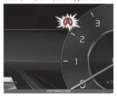
The engine will stop and the green AUTO STOP ((A)) indicator on the instrument cluster will appear.
