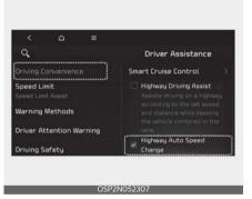
With the ignition switch or ENGINE START/STOP button in the ON position, select 'Setup → Vehicle → Driver Assistance → Driving Convenience → Highway Auto Speed Change' on the Infotainment system screen to set whether to use the function.
