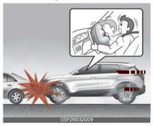
Front air bags are designed to inflate in a frontal collision depending on several factors, including the severity of impact of the front collision.
