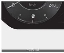
This gauge indicates the approximate amount of fuel remaining in the fuel tank.
