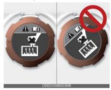
Maker sure that the tiny protrusions inside the coolant cap are securely interlocked. Maintenance Engine coolant
