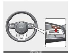
2. Push the (+) switch up or (-) switch down, and release it at the desired speed. The set speed will increase by 1 km/h (1 mph) each time the switch is operated in this manner.
