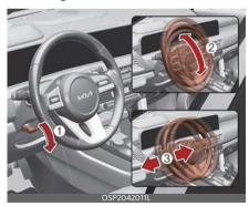
To change the steering wheel angle, pull down the lock release lever (1).
