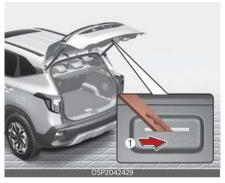
To unlock and open the liftgate manually from inside the luggage compartment, perform the following procedure:
