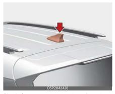
Shark-fin antenna transmit and receive signals such as AM/FM and GPS. Additional signals are sent and received according to vehicle options.
