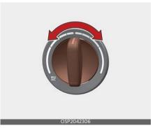
To change the air temperature in the passenger compartment, turn the knob
