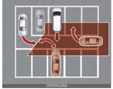
Rear Cross-Traffic Collision-Avoidance Assist may detect vehicles which are parking or pulling out near your vehicle (for example, a vehicle leaving beside your vehicle, a vehicle parking or pulling out in the rear area, a vehicle approaching your vehicle making a turn, etc.). If this occurs, Rear Cross-Traffic Collision-Avoidance Assist may unnecessarily warn the driver and control the brake. Always check your surroundings while backing up.
