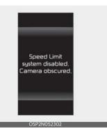
When the front windshield where the front view camera is located is covered with foreign material, such as snow or
