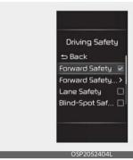
With the ignition switch or ENGINE START/STOP button in the ON position, select **User Settings** → **Driver Assistance** → **Driving Safety** on the LCD display or **Setup** → **Vehicle** → **Driver Assistance** → **Driving Safety** on the Infotainment system screen to set whether to use the function.
