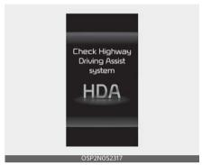
When Highway Driving Assist is not working properly, the warning message will appear, and the ( ) warning light will appear on the cluster. Have Highway Driving Assist be inspected by an authorized Kia dealer.
