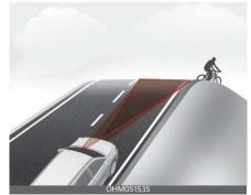
Forward Collision-Avoidance Assist may not detect other vehicle, pedestrian or cyclist in front while driving uphill or downhill and this may result
