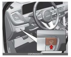
When the liftgate is closed, press the power liftgate open/close button for 1 second. The power liftgate opens with a warning sound.
