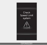
When Intelligent Speed Limit Assist is not working properly, the warning message will appear on the cluster for several seconds, and the master ( ) warning light and speed limit warning light ( ) will appear on the cluster. In this case, have the vehicle inspected by an authorized Kia dealer.
