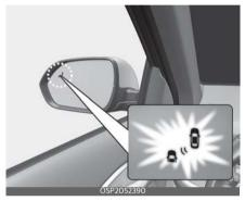
The warning light on the outside rear view mirror and head-up display (if equipped) will appear when the vehicle on both lanes is detected from the rear. A Vehicle detection will operate in the following conditions.
