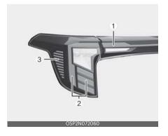
If the tail lamp (1)/tail and stop lamp&side marker lamp (2)/side marker lamp (3) is not functioning, please have your vehicle inspected by an authorized Kia dealer. The LED lamp cannot be replaced as a single unit because it is an integrated component. Instead, the entire LED lamp unit must be replaced. It's essential to have a skilled technician check or repair the tail lamp (1)/tail and stop lamp&side marker lamp (2)/side marker lamp (3) to prevent any damage to related vehicle parts.
