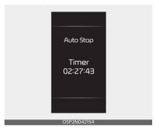
This mode displays the elapsed time of Auto Stop by "Idle stop and go system". For more details, refer to "Idle Stop and Go (ISG) system (if equipped)" on page 5-46.
