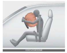
A fully inflated airbag (with a properly fastened seat belt) slows the forward motion of the driver or passenger, reducing the risk of head and chest injury.
