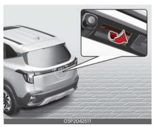
When the liftgate is closed, press the power liftgate open/close switch to open the liftgate.
