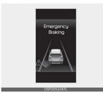
The warning light on the outside rear view mirror, head-up display (if equipped) and an audible warning will warn the driver of a collision. It assists in braking control to prevent a collision with a vehicle approaching from the blind spot area. Collision-Avoidance Assist will be activated in the following conditions.
