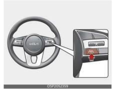
• With the vehicle on, press and hold the Lane Driving Assist button to turn on/off Lane Keeping Assist. If Lane Keeping Assist is activated, the indicator ( ) will be displayed on the cluster.
