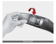
Even if the light switch is in the OFF position, the low beam headlights, taillights and the low beam indicator light turns ON automatically to provide better safety during low light environment.
