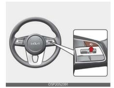
Press the Driving Assist button to turn Cruise Control off. The Cruise indicator will go off.
