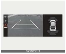
You can change Rear View Monitor 'Display Contents' and 'Display Settings' or by touching the setup icon (♠) on the screen while Rear View Monitor is operating, or selecting 'Setup → Vehicle → Driver Assistance → Parking Safety → Camera Settings' from the Settings menu while the engine is on.
