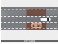
Blind-Spot Collision-Avoidance Assist helps detect and informs the driver that a vehicle is in the blind spot.
