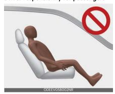
The driver must advise the passengers to keep the seatback in an upright position whenever the vehicle is in motion. If a seat is reclined during an accident, the restraint system's ability to restrain the passenger will be greatly reduced.
