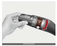
The fog lights will turn on when the fog light switch (1) is turned to the on position after the headlight is turned on. To turn off the fog lights:
