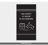
When Highway Driving Assist is operating, your vehicle will stop if the vehicle ahead of you stops. Also, if the vehicle ahead of you starts moving within 30 seconds after the stop, your vehicle will start as well. In addition, after the vehicle has stopped and 30 seconds have
