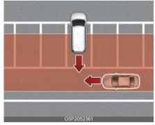
Rear Cross-Traffic Collision-Avoidance Assist may detect vehicles passing by behind you when parking backwards into a parking space. If this occurs, Rear Cross-Traffic Collision-Avoidance Assist may unnecessarily warn the driver and control the brake.
