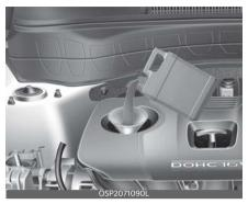
Use a funnel to help prevent oil from being spilled on engine components. Use only the specified engine oil. (Refer to "Recommended lubricants and capacities" on page 9-9.)
