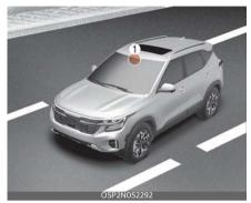
The front view camera is used as a detecting sensor to detect lane markings and front vehicles. Refer to the picture above for the detailed location of the detecting sensor.
