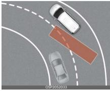
Blind-Spot Collision-Avoidance Assist may not operate properly when driving on a curved road. Blind-Spot Collision-Avoidance Assist may not detect the vehicle in the next lane.
