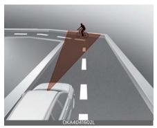
Forward Collision-Avoidance Assist may detect a vehicle, pedestrian or cyclist in the next lane or outside the lane when driving on a curved road. If this occurs, Forward Collision-Avoidance Assist may unnecessarily warn the driver and control the brake or steering wheel. Always check the traffic conditions around the vehicle.
