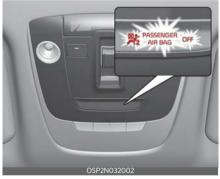
The ODS is designed to detect the presence of a properly-seated front passenger and determine if the passenger's front air bag should be enabled (may inflate) or not. Only the front passenger front air bag is controlled by the ODS. Do not put anything in front of the passenger air bag "ACC" indicator.
