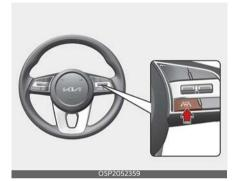
With the ignition switch or ENGINE START/STOP button in the ON position, press the Lane Driving Assist button located on the steering wheel to turn on Lane Following Assist. The white or green (((A)) indicator light will appear on the cluster.
