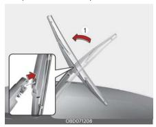
2. Install the new blade assembly by inserting the center part into the slot in the wiper arm until it clicks into the place.
