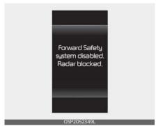
When the front windshield where the front view camera is located, front radar cover or sensor is covered with foreign material such as snow or rain, it can reduce the detecting performance and temporarily limit or disable Forward Collision-Avoidance Assist. If this occurs the warning message will appear and the
