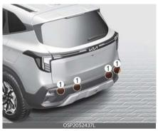
Refer to the picture above for the detailed location of the detecting sensors.
