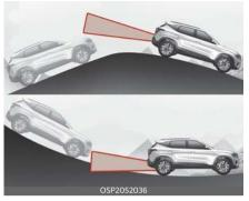
Blind-Spot Collision-Avoidance Assist may not operate properly when driving on a slope. Blind-Spot Collision-Avoidance Assist may not detect the vehicle in the next lane or may incorrectly detect the ground or structure.
