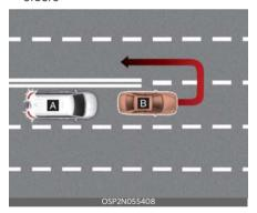
[A]: Your vehicle, [B]: Front vehicle If the vehicle in front makes a sharp turn, such as to turn left or right or make a Uturn, etc., Leading Vehicle Departure Alert may not operate properly.
