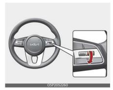
3. The set speed limit will be displayed on the cluster. If you would like to drive over the preset speed limit, depress the accelerator pedal. The set speed limit will blink and chime will sound until you return the vehicle speed within the speed limit.
