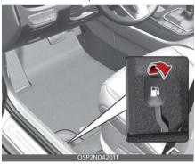
3. Pull the fuel filler door (1) out to fully open.
