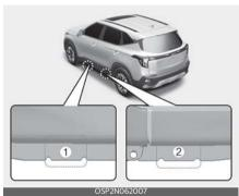
8. Insert the wheel lug nut wrench into the jack and turn it clockwise, raising the vehicle until the tire just clears the ground. This measurement is approximately 2.5 cm (1 in).
