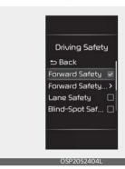
With the ignition switch or ENGINE START/STOP button in the ON position, select **User Settings** → **Driver Assistance** → **Driving Safety** on the LCD display or **Setup** → **Vehicle** → **Driver Assistance** → **Driving Safety** on the Infotainment system screen to set
