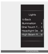
With the ignition switch or ENGINE START/STOP button in the ON position, select 'Lights → High Beam Assist' from the Settings menu to turn on High Beam Assist and deselect to turn off the function.
