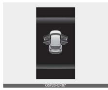
• This warning is displayed indicating which door, hood or liftgate is open.
