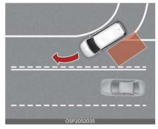
Blind-Spot Collision-Avoidance Assist may not operate properly when driving where the road merges or divides. Blind-Spot Collision-Avoidance Assist may not detect the vehicle in the next lane. Always pay attention to road and driving conditions while driving.
