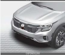
The front view camera and front radar are used as a detecting sensor to detect vehicles in front. Refer to the picture for
