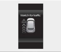
The warning light on the side view mirror will blink and the warning message will appear on the cluster, and an audible warning will sound.
