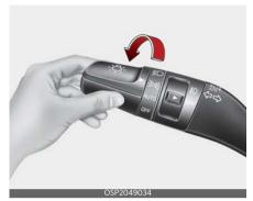
When the light switch is in the position lamp position, the tail, license and instrument panel lights will turn ON.
