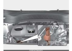
If the coolant level is low, add enough specified coolant to provide protection against freezing and corrosion. Bring the level to F, but do not overfill.
