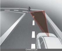
Forward Collision-Avoidance Assist may not detect the vehicle, pedestrian or cyclist traveling in front on a curved road.
