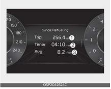
Fuel efficiency is calculated after the vehicle has run for more than 300 meters (0.2 miles).
