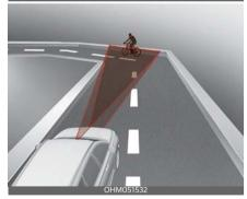
Forward Collision-Avoidance Assist may detect the vehicle, pedestrian or cyclist in the next lane or outside the lane when driving on a curved road. If this occurs, Forward Collision-Avoidance Assist may unnecessarily warn the driver and control the brake.
