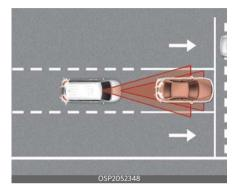
Forward Collision-Avoidance Assist is designed to help detect and monitor the vehicle ahead or help detect a pedestrian or cyclist in the roadway and warn the driver that a collision is imminent with a warning message, audible warning and apply emergency braking.
