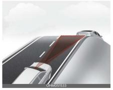
During uphill or downhill driving, Smart Cruise Control may not detect a moving vehicle in your lane, and cause your vehicle to accelerate to the set speed.
