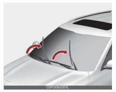
To inspect or replace the windshield wiper blades and to prevent damaging the hood, move the windshield wiper blades as follows:
