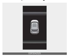
If the driver turns off the engine when the sunroof is not fully closed, the warning chime will sound for several seconds and the sunroof open warning will appear on the cluster LCD display. Close the sunroof securely when leaving your vehicle.
