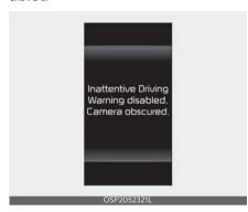
When the front view camera is located is covered with foreign material, such as snow or rain, it can reduce the detecting performance and temporarily limit or disable Driver Attention Warning. If this occurs the warning message, and ( \( \bigcirc \)) warning light will appear on the cluster. Driver Attention Warning will operate normally when snow, rain or foreign material is removed. Always keep it clean.
