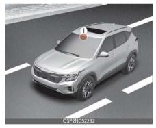
The front view camera is used as a detecting sensor to help detect driving patterns and front vehicle departure while vehicle is being driven.
