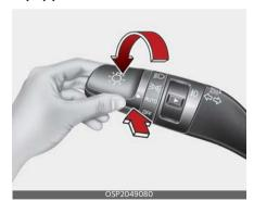
High Beam Assist is a function that automatically adjusts the headlamp range (switches between high beam and low beam) depending on the brightness of
