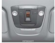
The sunroof can only be operated when the ignition switch or the ENGINE START/STOP button is in the ON or START position. The sunroof can be operated for approximately 3 minutes after the ignition switch or the ENGINE START/STOP button is in the ACC or LOCK/OFF position. However, if the front door is open, the sunroof cannot be operated even within the 3 minutes period.
