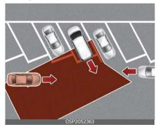
Rear Cross-Traffic Collision-Avoidance Assist may be limited when backing up diagonally, and may not detect the vehicle approaching from the left or right. If this occurs, Rear Cross-Traffic Collision-Avoidance Assist may not warn the driver or control the brakes when necessary.
