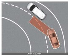
Blind-Spot Collision-Avoidance Assist may not operate properly when driving on the curved road. Blind-Spot Collision-Avoidance Assist may recognize the vehicle in the same lane.
