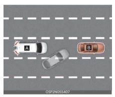
[A]: Your vehicle, [B]: Front vehicle If a vehicle cuts in front of your vehicle, Leading Vehicle Departure Alert may not operate properly.
