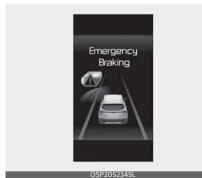
The warning message and an audible warning to warn the driver that emergency braking will be assisted. The brake assist will be activated and it helps avoiding collision of a vehicle. Emergency braking will be activated in the following conditions.
