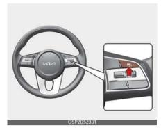
Press the Driving Assist button to turn on Smart Cruise Control. The set speed will be set to the current speed on the cluster.
