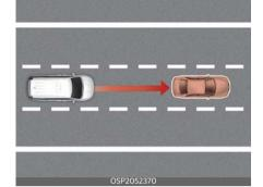
Highway Driving Assist is designed to help detect vehicles and lanes ahead, and help maintain distance from the vehicle ahead, maintain the set speed, help center the vehicle in the lane while driving on the highway (or motorway).
