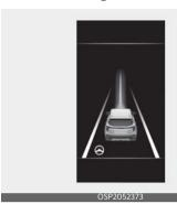
If the vehicle ahead or both lane markings are detected and your vehicle speed is below 180 km/h (110 mph), the green ( ) indicator light will appear on the cluster, and the function will help center the vehicle in the lane by controlling the steering wheel.
