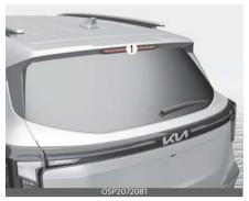
If the high-mounted stop lamp (LED) (1) is not functioning, please have your vehicle inspected by an authorized Kia dealer. The LED lamp cannot be replaced as a single unit because it is an integrated component. Instead, the entire LED lamp unit must be replaced. It's essential to have a skilled technician check or repair the high-mounted stop lamp (LED) to prevent any damage to related vehicle parts.
