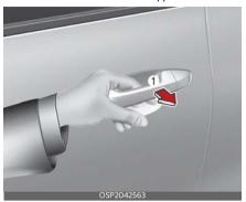
Pressing the button of the front outside door handle (for button type) or put your hand inside the door handle pocket (1) and touch the door unlock sensor on the inside of the outside door handle (for touch sensor type), with all doors (and liftgate) closed and locked, unlocks all the doors (and liftgate), if the 2 Press Unlock function is deactivated.
