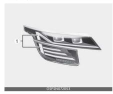
If the LED (1) lamp is not functioning, please have your vehicle inspected by an authorized Kia dealer. The LED lamp cannot be replaced as an individual component since it is an integrated unit. Instead, the entire LED lamp unit must be replaced.
