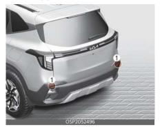
Refer to the picture above for the detailed location of the detecting sensors.
