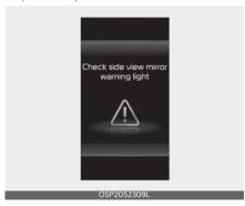
When the outside rear view mirror warning light is not working properly, the warning message will appear on the cluster for several seconds, and the master warning light ((!\)) will appear on the cluster. Have Safe Exit Warning be inspected by an authorized Kia dealer.
