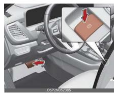
To release the EPB manually: Press the EPB switch in the following condition.
