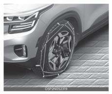
Since the sidewalls of radial tires are thinner, they can be damaged by mounting some types of snow chains on them. Therefore, the use of snow tires is recommended instead of snow chains. Do not mount tire chains on vehicles equipped with aluminum wheels; snow chains may cause damage to the wheels. If snow chains must be used, use fabric-type chains or wire-type chains with a thickness of less than 12 mm (0.47 in).
