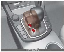
Whether the vehicle is stationary or in motion, sports mode can be selected by pushing the shift lever from the D (Drive) position into the manual gate. To return to D (Drive) range operation, push the shift lever back into the main gate. SPORT mode manages the driving dynamics by automatically adjusting the steering effort, and the engine and transmission control logic for enhanced driver performance.
