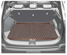
To keep items from shifting in the cargo area, you can use the 4 holders located in the cargo area to attach the luggage net. (if equipped)
