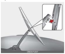
Make sure the blade assembly is installed firmly by trying to pull it slightly. To prevent damage to the wiper arms or other components, have the wiper blade replaced by an authorized Kia dealer.
