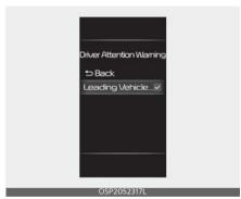
With the ignition switch or ENGINE START/STOP button in the ON position, select User Settings → Driver Assistance → Driver Attention Warning on the LCD display or Setup → Vehicle → Driver Assistance → Driver Attention Warning on the Infotainment system screen.
