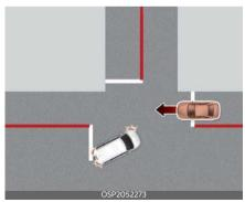
Junction Turning function can help avoid a collision with an oncoming vehicle in an adjacent lane when turning left at a
