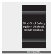
When the rear bumper around the rearside radar or sensor is covered with foreign matters, such as snow or rain, or installing a trailer or carrier, it can reduce the detecting performance and temporarily limit or disable Safe Exit Warning. If this occurs, the 'Blind-Spot Safety system disabled. Radar blocked' warning message will appear on the cluster.
