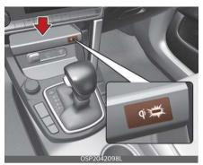
Firmly close all doors, and ignition switch is ON. To start wireless charging, place the smart phone equipped with wireless charging function on the wireless charging pad.
