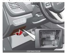
3. Pull the suspected fuse straight out.
