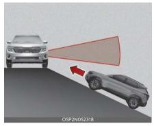
Rear Cross-Traffic Collision-Avoidance Assist may be limited when the vehicle is on a uphill or downhill slope, or near it, and may not detect the vehicle approaching from the left or right. If this occurs, Rear Cross-Traffic Collision-Avoidance Assist may not warn the driver or control the brakes when necessary.
