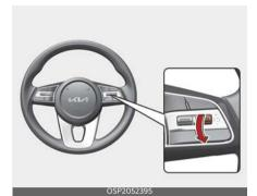
Push down the - switch, and release it immediately. The set speed will decrease by 1 km/h (1 mph) each time the switch is operated in this manner.
