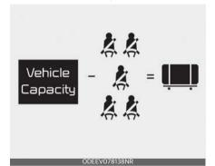
Item Total Description Vehicle Capacity 385 kg Α Weight (849 lbs.) Subtract Occupant 340 kg В Weight (750 lbs.) 68 kg (150 lbs.)×5 Available Cargo and 45 kg C Luggage weight (99 lbs.)
