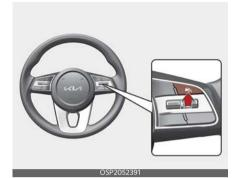
Press the Driving Assist button to turn Manual Speed Limit Assist off. The Speed Limit indicator will go off. Always press the Driving Assist button to turn Manual Speed Limit Assist off when not in use.
