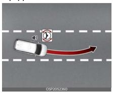
Lane Keeping Assist is designed to help detect lane markings (or road edges) while driving over a certain speed. Lane Keeping Assist will warn the driver if the vehicle leaves the lane without using the turn signal, or will automatically assist the driver's steering to help prevent the vehicle from departing the lane.
