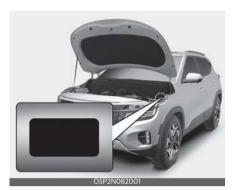
You can find out which air conditioning refrigerant is applied your vehicle at the label inside of the engine compartment.
