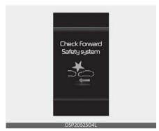
When Forward Collision-Avoidance Assist is not working properly, the warning message will appear and the
