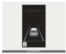
When driving at a speed higher than the displayed speed limit, the road sign indicator will be red.
