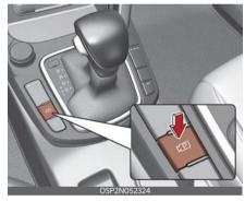
Press the Parking/View button to turn on Rear View Monitor.
