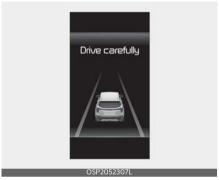
When the vehicle is stopped due to emergency braking, the warning message will appear on the cluster. For your safety, the driver should depress the brake pedal immediately and check the surroundings.
