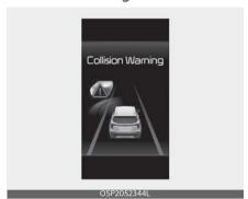
Collision warning will alert the driver with a warning message and an audible warning. Collision warning will be activated in the following conditions.
