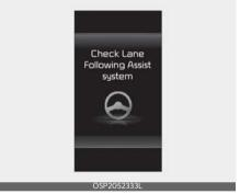
When Lane Following Assist is not working properly, the warning message will appear for several seconds and ( ) warning light will appear on the cluster. If this occurs, have the vehicle inspected by an authorized Kia dealer.
