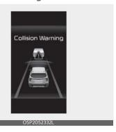
Collision warning will alert the driver with a warning message and an audible warning. Collision Warning will be activated in your driving speed and the following conditions.
