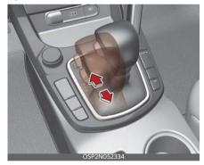
Whether the vehicle is stationary or in motion, sports mode is selected by pushing the shift lever from the D (Drive) position into the manual gate. To return to D (Drive) range operation, push the shift lever back into the main gate. In sports mode, moving the shift lever backwards and forwards will allow you to make gearshifts rapidly. In contrast to a manual transmission, the sports mode
