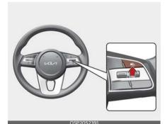
Press the Driving Assist button at the desired speed. The set speed and Cruise (CRUISE) indicator will appear on the cluster.
