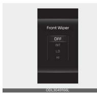
This indicator displays which wiper speed is selected using the wiper control.
