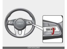
To resume Manual Speed Limit Assist after the function was paused, operate the +, - or  $||\bigcirc$  switch.
