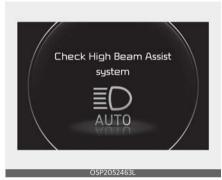
When High Beam Assist is not working properly, the 'Check High Beam Assist system' warning message will appear and ( ) warning light will appear on the cluster. If this occurs, we recommended that the function be inspected by an authorized Kia dealer
