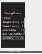
With the ignition switch or ENGINE START/STOP button in the ON position, and select User Settings → Driver Assistance → Driving Safety → Exit Safety on the instrument cluster or Setup → Vehicle → Driver Assistance → Driving Safety → Exit Safety on the infotainment system.
