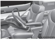
A rearward-facing child seat provides restraint with the seating surface against the back of the child. The harness system holds the child in place, and in an accident, acts to keep the child positioned in the seat and reduce the stress to the neck and spinal cord.
