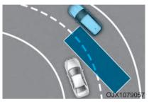
Blind-Spot Collision Warning may not operate properly when driving on a curved road. The function may not detect the vehicle in the next lane.
