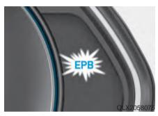
This warning light illuminates if the ignition switch is set to the ON position and goes off in approximately 3 seconds if the system is operating normally.
