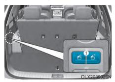
Push the 2nd row seat back folding switch (1) located on the left side of the cargo area. (L : Left seatback folding, R : Right seatback folding)
