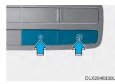
2. The fan speed can be set to the desired speed by pushing the fan speed control button. The higher the fan speed is, the more air is delivered.
