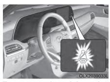
Front passenger's seat belt warning As a reminder to the front passenger, the front passenger's seat belt warning lights will illuminate for approximately 6 seconds each time you place the ignition switch to the ON position regardless of belt fastening. If you continue not to fasten the seat belt and you drive over 6 mph (9 km/h), the warning light will stay illuminated.
