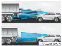
If the vehicle in front of you has cargo that extends rearward from the cab, or when the vehicle in front of you has higher ground clearance, additional special attention is required. Forward Collision-Avoidance Assist may not be able to detect the cargo extending from the vehicle. In these instances, you must maintain a safe braking distance from the rearmost object, and if necessary, steer your vehicle and press the brake pedal to reduce your driving speed in order to maintain distance.
