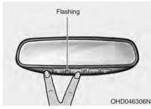
1. When programming the buttons for the first time, press and hold the left and center buttons (⊉, <u>1</u>) simultaneously for approximately 20 seconds until the indicator light begins to flash. (This procedure erases the factory-set default codes. Do not perform this step to program additional hand-held transmitters.)
