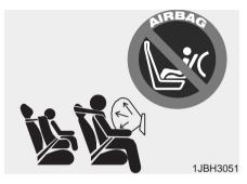
Even though your vehicle is equipped with the OCS, never install a child restraint in the front passenger's seat. An inflating air bag can forcefully strike a child or child restraint resulting in serious or fatal injury.
