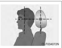
Adjust the head restraints so the middle of the head restraint is at the same height as the height of the top of the eyes.
