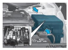
Inside the fuse/relay box cover, you can find the fuse/relay label describing fuse/relay names and ratings.
