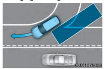
Blind-Spot Collision Warning may not operate properly when driving where the road merges or divides. The function may not detect the vehicle in the next lane.
