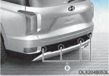
[A] : Front ultrasonic sensor,[B] : Rear ultrasonic sensor
