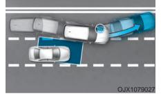
When changing lanes by detecting the lane ahead, if the function judges that there is a collision risk with an approaching vehicle in the blind spot, the function will help avoid collision by applying the brake.
