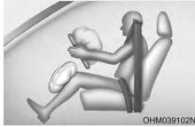
When the SRSCM detects a sufficiently severe impact to the front of the vehicle, it will automatically deploy the front air bags.
