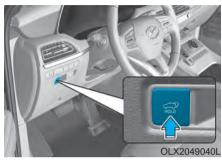
Power liftgate button Press the power liftgate button for approximately one second.
