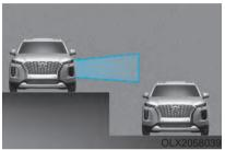
Blind-Spot Collision Warning may not operate properly when driving where the heights of the lanes are different. The function may not detect the vehicle on a road with different lane heights (underpass joining section, grade separated intersections, etc.).
