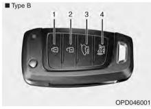
Your HYUNDAI uses a remote key, which you can use to lock or unlock the driver and passenger doors or the rear liftgate.
