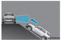
Rear Cross-Traffic Collision Warning may be limited when the vehicle is on a uphill or downhill slope, or near it, and may not detect the vehicle approaching from the left or right. If this occurs, the function may not warn the driver when necessary.
