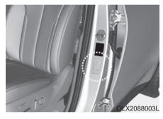
All specifications (sizes and pressures) can be found on a label attached to the driver's side center pillar.
