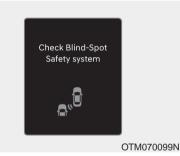
When Blind-Spot Collision-Avoidance Assist is not working properly, the 'Check Blind-Spot Collision-Avoidance Assist' warning message will appear on the cluster, and the function will turn off automatically or the function will be limited. Have the vehicle inspected by an authorized HYUNDAI dealer.
