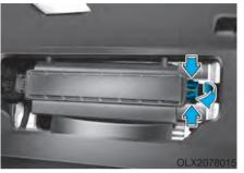
3. Remove the climate control air filter case while pressing the lock on right side of the cover.
