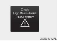
When High Beam Assist is not working properly, the warning message will come on for a few second. After the message disappears, the master warning light  $(\triangle)$  will illuminate.
