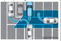
Rear Cross-Traffic Collision Warning may detect vehicles which are parking or pulling out near your vehicle (for example: a vehicle leaving beside your vehicle, a vehicle parking or pulling out in the rear area, a vehicle approaching your vehicle making a turn, etc.). If this occurs, the function may unnecessarily warn the driver.
