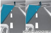
Forward Collision-Avoidance Assist may not detect other vehicles, pedestrians or cyclists in front of you on curved roads adversely affecting the performance of the sensors. This may result in no warning or braking assist when necessary.
