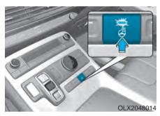
When the ignition switch is in the ON position or when the engine is running, press the heated steering wheel button to warm the steering wheel. The indicator on the button will illuminate.
