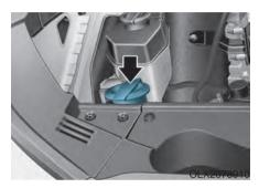
Check the fluid level in the washer fluid reservoir and add fluid if necessary. Plain water may be used if washer fluid is not available. However, use washer solvent with antifreeze characteristics in cold climates to prevent freezing.
