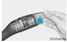
Push the lever away from you to spray rear washer fluid and to run the rear wipers 1~3 cycles. The spray and wiper operation will continue until you release the lever.
