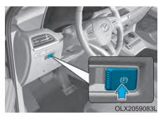
To release the EPB (Electronic Parking Brake):
