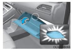
The glove box lamp comes on when the glove box is opened.
