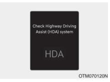
When Highway Driving Assist or Highway Lane Change function is not working properly, the 'Check Highway Driving Assist (HDA) system' warning message will appear, and the A warning light will illuminate on the cluster. Have the vehicle inspected by an authorized HYUNDAI dealer.
