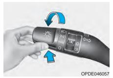
High Beam Assist will automatically adjust the headlamp range (switches between high beam and low beam) according to the brightness of other vehicles and road conditions. Detecting sensor (Front view camera)
