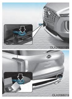
If towing is necessary, we recommend you have it done by an authorized HYUNDAI dealer or a commercial tow truck service. If towing service is not available in an emergency, your vehicle may be temporarily towed using a cable or chain secured to the emergency towing hook at the front (or rear) of the vehicle.
