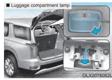
1. Using a flat-blade screwdriver, gently pry the lens from the interior lamp housing.
