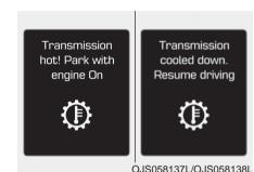
• Under certain conditions, such as repeated stop-and-go launches on steep grades, sudden take off or acceleration, or other harsh driving conditions (mud or sand road), the transmission temperatures will increase excessively. Finally the transmission could be overheated.
