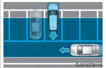
Rear Cross-Traffic Collision Warning may detect vehicles passing by behind you when parking backwards into a parking space. If this occurs, the function may unnecessarily warn the driver.
