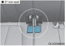
• The rear seat belt buckles can be stowed in the pocket between the rear seatback and cushion when not in use.
