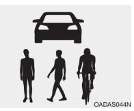
The illustration above shows the image the front view camera will detect as a vehicle, pedestrian and cyclist.
