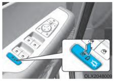
In addition, when the electronic child safety lock button is in the LOCK position and an approaching vehicle from the rear area is detected, the electronic child safety lock button will not unlock even if the driver presses the button to prevent the rear doors from opening.
