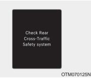
When Rear Cross-Traffic Collision Warning is not working properly, the 'Check Rear Cross-Traffic Safety system' warning message will appear on the cluster, and the function will turn off automatically, or the function will be limited. Have the vehicle inspected by an authorized HYUNDAI dealer.
