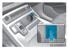
The Downhill Brake Control (DBC) feature assists the driver to descend down a steep hill without having to depress the brake pedal.
