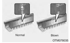
A vehicle's electrical system is protected from electrical overload damage by fuses.
