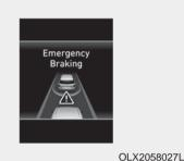
In emergency braking situation, braking is assisted with strong braking power by the system to help prevent collision with the vehicle ahead.
