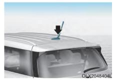
Your vehicle uses a roof antenna to receive AM or/and FM broadcast signals. This antenna pole is removable. To remove the roof antenna pole, turn it counterclockwise.
