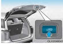
Power liftgate inner button Press the power liftgate inner button
