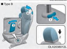
To reinstall the head restraint:
