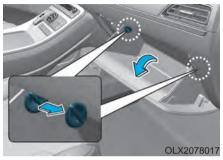
1. With the glove box open, remove the stoppers on both sides to allow the glove box to hang freely on the hinges.
