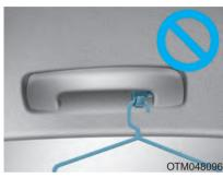
Do not hang other objects such as hangers or hard objects except clothes. Also, do not put heavy, sharp or breakable objects in the clothes pockets. In an accident or when the curtain air bag is inflated, it may cause vehicle damage or personal injury.
