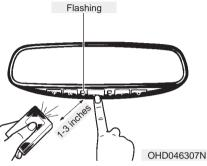
3. While the HomeLink indicator light (4) (Fig. 2) is flashing slowly in red, press and hold the hand-held remote button. Continue pressing the HomeLink button and the hand-held remote button until the HomeLink indicator light (4) light changes from slowly to rapidly. You may now release the buttons.
