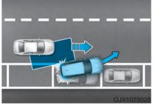
When you are driving forward out of a parking space, if the function judges that there is a collision risk with an approaching vehicle in the blind spot, the function will help avoid collision by applying the brake.
