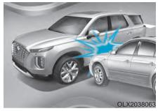
Front air bags may not inflate in side impact collisions, because occupants move in the direction of the collision, and thus in side impacts, front air bag deployment would not provide additional occupant protection.
