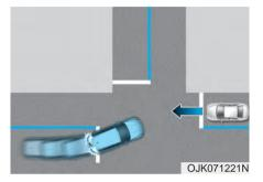
Junction Turning function will help avoid a collision with an oncoming vehicle in an adjacent lane when turning right at a crossroad with the turn signal on by applying emergency braking.
