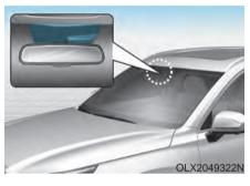
Auto defogging helps reduce the possibility of fogging up the inside of the windshield by automatically sensing the moisture on inside the windshield.
