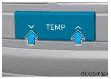
2. The temperature of delivered air can be set to the desired temperature by pushing the temperature control button.
