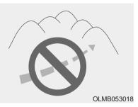
Do not drive across the contour of steep hills. A slight change in the wheel angle can destabilize the vehicle, or a stable vehicle may lose stability if the vehicle stops its forward motion. Your vehicle may roll over and lead to a serious injury or death. Driving through water
