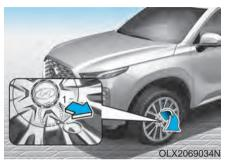
6. Insert the tool (1, if equipped) into the hole and pull out the wheel cover.
