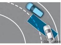
Blind-Spot Collision Warning may not operate properly when driving on the curved road. The function may recognize the vehicle in the same lane.
