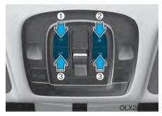
Front Room Lamp (1) ( 亦): Press the button to turn the front and rear room lamps on or off.
