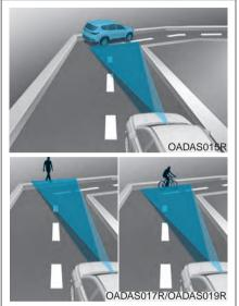
Forward Collision-Avoidance Assist may detect a vehicle, pedestrian or cyclist in the next lane or outside the lane when driving on a curved road. If this occurs, the function may unnecessarily warn the driver and control the brake. Always check the traffic conditions around the vehicle.
