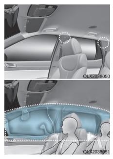
Curtain air bags are located along both sides of the roof rails above the front and rear doors. They are designed to help protect the heads of the front seat occupants and the rear outboard seat occupants in certain side impact collisions.
