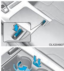
Push the button and the cover opens. Push the buttons and the cup supporter protrudes from the front console. Push in the cup supporter securely after use.
