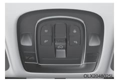
The sunroof can only be operated when the ignition switch is in the ON position.
