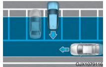
Rear Cross-Traffic Collision-Avoidance Assist may detect vehicles passing by behind you when parking backwards into a parking space. If this occurs, the function may unnecessarily warn the driver and control the brake.
