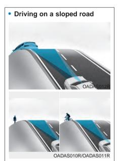
Forward Collision-Avoidance Assist may not detect other vehicles, pedestrians or cyclists in front of you while driving uphill or downhill adversely affecting the performance of the sensors. This may result in unnecessary warning or braking assist, or no warning or braking assist when necessary.
