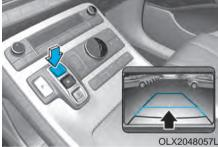
Rear View Monitor will show the area behind the vehicle to assist you when parking or backing up. Detecting sensor
