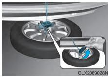
6. Draw out the retainer guide (1) through the center hole of the spare tire.
