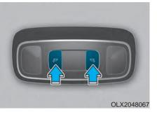
Rear Room Lamp ( ァ 도): Press either buttons to turn the room lamp on or off.
