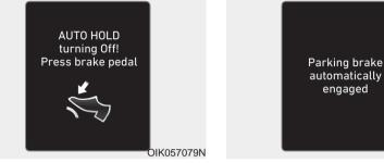
AUTO HOLD turning Off! Press brake pedal
