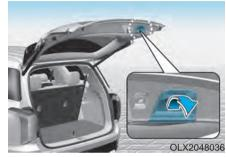
Lower the liftgate lid and press down until it locks. To be sure the liftgate lid is securely fastened, always check by trying to pull it up again without pressing the liftgate handle switch.
