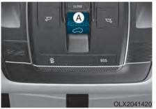
The sunshade opens automatically when the sunroof glass is opened by pushing the sunroof switch (A) rearward, but the sunshade does not close automatically when the sunroof glass is closed. Also, only the sunshade cannot be closed when the sunroof glass is opened.
