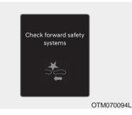
When Forward Collision-Avoidance Assist is not working properly, the 'Check Forward Safety system(s)' warning message will appear, and the so and A warning lights will illuminate on the cluster. have the vehicle inspected by an authorized HYUNDAI dealer.
