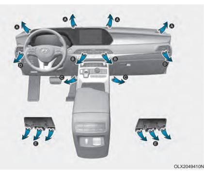
The mode selection button controls the direction of the air flow through the ventilation system. Air can be directed to the floor, dashboard outlets, or windshield. Five symbols are used to represent Face, Bi-Level, Floor, Floor-Defrost and Defrost air position.
