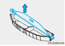
3. While pushing the guide pin, pull out the cargo security screen.
