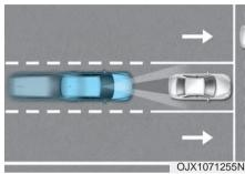
Forward Collision-Avoidance Assist is designed to help detect and monitor the vehicle ahead or help detect a pedestrian or cyclist in the roadway and warn the driver that a collision is imminent with a warning message and an audible warning, and if necessary, apply emergency braking. Junction Turning function (if equipped)
