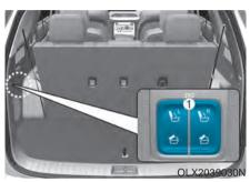
Push the 3rd row seat back folding switch (1) located on the left side of the cargo area. (L : Left seatback folding/unfolding, R : Right seatback folding/unfolding)
