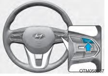
To turn off Smart Cruise Control Pushing the CRUISE/ Dutton. The cruise indicator will go off. If you wish not to use the cruise control system, always turn the function off by pushing the CRUISE/ Dutton.
