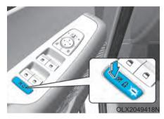
If you push the Electronic child safety lock switch and the indicator illuminates, rear passengers cannot open the rear door from inside the vehicle. To cancel the Electronic child safety lock system, push the Electronic child safety lock system switch one more time and then the indicator turns off.
