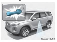
Puddle lamp (if equipped) and door handle lamp (if equipped)
