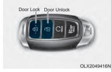
Press the button on the driver's outside door handle while carrying the Smart Key with you or press the Door Unlock button on the Smart Key, the driver's door will unlock. If you press the button on the front passenger's outside door, all doors will unlock.
