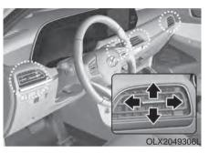
The instrument panel vent air flow can be directed up/down or left/right using the vent adjustment lever.
