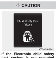
If the Electronic child safety lock system is not operated when pushing the Electronic child safety lock switch, the message is displayed and the alarm will sound.
