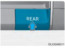
If you press the rear climate control button, rear passengers can control the rear climate system.
