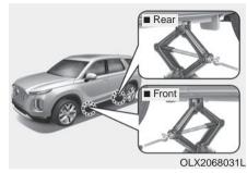
8. Place the jack at the designated jacking position under the frame closest to the tire you are changing. The jacking positions are plates welded to the frame with two notches. Never jack at any other position or part of the vehicle. Doing so may damage the side seal molding or other parts of the vehicle.
