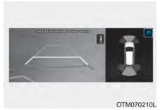
You can change Rear View Monitor 'Display Contents' or 'Display Settings' by touching the setup icon (O) on the screen while Rear View Monitor is operating, or selecting 'Driver Assistance  $\rightarrow$  Parking Safety  $\rightarrow$  Camera Settings' from the Settings menu while the engine is on.
