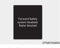
When the front windscreen where the front view camera is located, front radar cover or sensor is covered with foreign material, such as snow or rain, it can reduce the detecting performance and temporarily limit or disable Forward Collision-Avoidance Assist.
