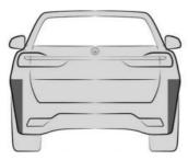
The radar sensors are located on the side of the rear bumper.
