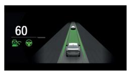
An example of active Driver Assistance: the indicator and warning lights for Distance Control and Assisted Driving Mode are displayed. At the same time, the Distance Control is animated in Assisted View.
