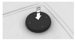
Push the controller in the corresponding direction to switch between menus, for example.
