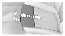
To adjust the thigh support, pull the thigh support lever at the front of the seat then push the thigh support forward or backward.
