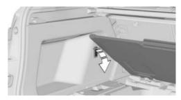
Do not place any weight on the cargo area floor when folded up. Before folding the cargo area floor down, fold in the holder.
