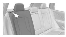
Pull the lever in the recess and fold the rear seat backrest forward.
