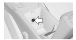
A socket is provided in the front center armrest under a cover. Pull off the cover before using the socket.
