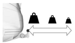
The gross vehicle weight of the loaded rear carrier depends on how far its center of gravity is from the ball head.
