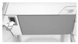
To open the glove compartment, press the button on the glove compartment.
