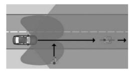
The sensors detect the traffic situation in their detection range on a straight road.
