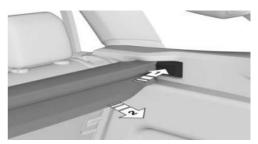
To remove the cargo cover, press the release button, arrow 1, and pull the cargo cover out toward the rear, arrow 2.
