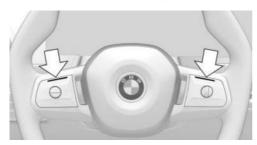
Similar to the displays for Assisted Driving Mode on the instrument cluster, the two LEDs above the keypads on the steering wheel illuminate.
