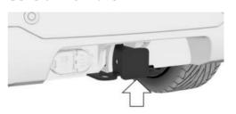
The mount for the trailer hitch is located on the rear of the vehicle, see arrow.
