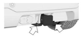
Two eyes can be found on the mount for the trailer hitch for attaching the trailer safety chain.
