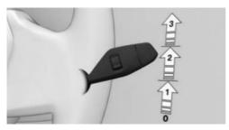
To activate the rain sensor: Push the wiper lever upward from position 0, arrow 1, once.
