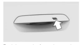
Touch the grooved surface on the external door handle of a closed front door with your
