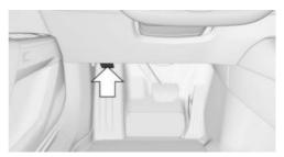
The unlock lever for the hood is located in the driver's footwell.
