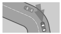
When Distance Control is on, if your set speed is too high for a bend, your vehicle will be slowed slightly in the bend. Because curves may not be anticipated in advance, drive into a curve at an appropriate speed.
