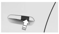
Hold the smartphone NFC antenna directly at the center of the driver's door handle. The position of the near field communication antenna depends on the smartphone model.
