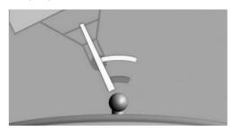
Two static circle segments are displayed in the camera image. These circle segments help to estimate the distance of the trailer to the trailer hirch
