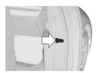
Side door lock for manually locking the doors.
