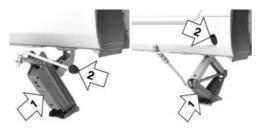
Insert the jack into the rectangular recess of the jacking point closest to the wheel to be changed.
