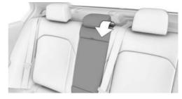
Pull down the sliding button to the right of the head restraint and fold the center section forward.
