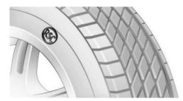
Run-flat tires are indicated by a circular icon containing the letters "RSC" on the tire sidewall.
