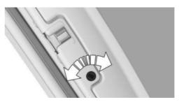
To secure the rear doors, release/lock the safety switch on the rear door using the integrated key.
