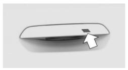
To close a window using the door handle of a closed front door, place a finger on the arooved surface of the door handle and hold it there without reaching into the recessed grip.
