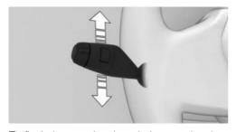
To flash the turn signal, push the turn signal lever up or down past the resistance point.
