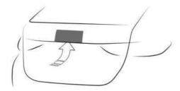
Press the button on the cargo area to access the vehicle while in deep sleep mode. Deep sleep mode remains on in this case.
