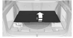
Fold out the cargo area floor holder in order to hold the cargo area floor in the folded-up position.
