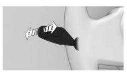
To reactivate the High Beam Assistant, press the turn signal lever up, arrow 1.
