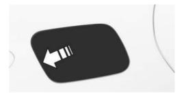
2. Open the fuel filler cap counterclockwise.
