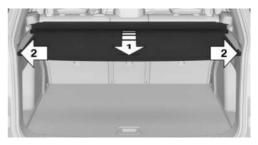
To close the cargo cover, slowly pull the cargo cover out and straight forward, arrow 1, and hook it to the holders on both sides, arrows 2.
