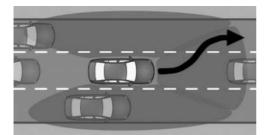
The sensors monitor and detect the clearance in front of the vehicle. Depending on the vehicle equipment, the areas next to the vehicle are also monitored.
