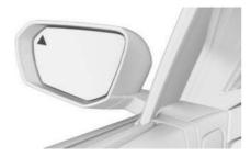
The warning light in the exterior mirror flashes if the rear sensors detect other vehicles when the vehicle is reversing.
