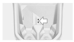
Two USB ports are located on the front center console.
