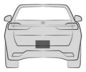
The Rear View Camera is located above the license-plate carrier.
