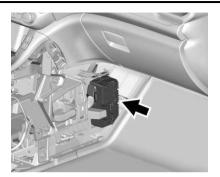
After accessing the fuses, ensure the fuse block cover is reinstalled, if equipped. To reinstall the fuse panel door, push the door back into its original location.
