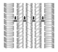
Treadwear indicators are one way to tell when it is time for new tires. Treadwear indicators appear when the tires have only 1.6 mm (1/16 in) or less of tread remaining. See *Tire Inspection* ♀ 327 and *Tire Rotation* ♀ 327.
