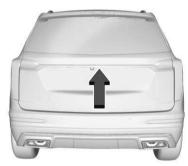
To open the liftgate, press the touch pad under the liftgate handle and lift up.
