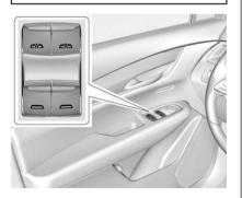
The power windows work when the vehicle is on, in accessory mode, or when Retained Accessory Power (RAP) is active. See *Retained Accessory Power (RAP)* ⇔ 206.
