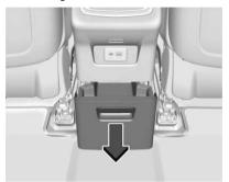
If equipped, pull the handle forward to access the rear storage drawer.
