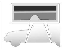
4. Position the jack lift head at the jack location nearest the tire being changed. The jacking location is indicated by a half circle notch in the metal flange. The jack must not be used in any other position.
