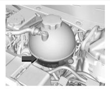
Check to see if coolant is visible in the coolant surge tank. If the coolant inside the coolant surge tank is boiling, do not do anything else until it cools down. If coolant is visible but the coolant level mark is not at or above the indicated mark, add a 50/50 mixture of clean, drinkable water and DEX-COOL coolant. Be sure the cooling system is cool before this is done. See Engine Overheating \$\times 298\$.
