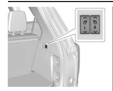
To return the seatback to the seating position from the cargo area, press and hold the seatback folding switch on the passenger side of the rear cargo area.
