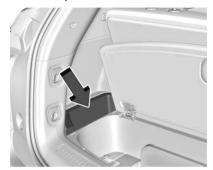
The rear compartment fuse block is in the cargo area, on the driver side of the vehicle behind the lower trim panel. To access the fuses in the Rear Electrical Center, remove the center cargo bin, then small side bin. See *Rear Storage* ❖ 87. See your dealer if additional assistance is needed.
