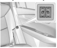
To return the seatback to the seating position from the second row seating area, press and hold the seatback folding switch on the right or left side of the second row seating area.
