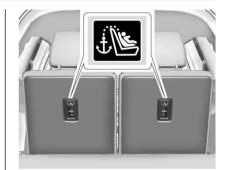
The top tether anchors are on the rear of the seatback for each seating position in the third row.
