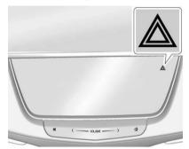
A: Touch on the center stack to make the front and rear turn signal lamps flash on and off. Touch again to turn the flashers off.
