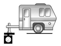
The trailer tongue weight contributes to the Gross Vehicle Weight (GVW). GVW includes the curb weight of your vehicle, any passengers, cargo, equipment, and the trailer tongue weight. Vehicle options, passengers, cargo, and
