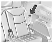
Insert the SD card into the card reader in the trim panel of the left-hand rear seat. Disable the system from the playback screen before removing the SD card from the reader. Do not remove the card while recording is enabled. This could corrupt the video file and/or the SD card
