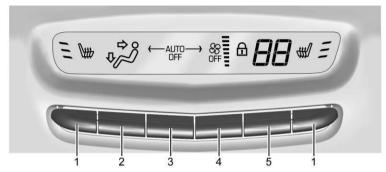
**Rear Climate Controls, Equipped with Heated Seats**
