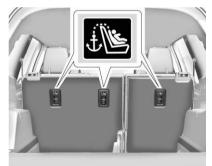
The top tether anchors are on the rear of the seatback for each seating position in the second row
