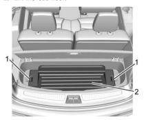
3. Remove the cargo management system tray (2) by pulling on the handles (1). See Cargo Management System ⇔ 91.
