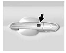
If equipped, the remote key must be within 1 m (3 ft) of the liftgate or door being opened.
