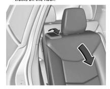
Pull the handle on the top of the seat forward and pull the seat forward.
