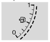
When the ignition is on, the fuel gauge indicates the approximate amount of fuel left in the tank
