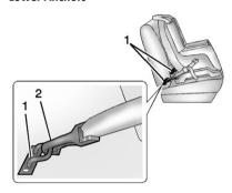
Lower anchors (1) are metal bars built into the vehicle. There are two lower anchors for each LATCH seating position that will accommodate a child restraint with lower attachments (2).
