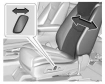
Tilt the top of the control rearward to recline. Tilt the top of the control forward to raise.
