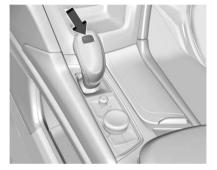
**P:** This position locks the drive wheels. Use P (Park) when starting the engine because the vehicle cannot move easily.
