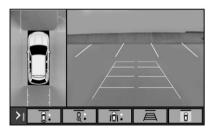
Touch the camera view buttons along the bottom of the infotainment display to access each view:
