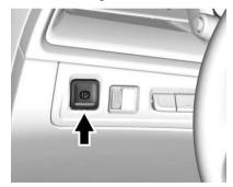
The Electric Parking Brake (EPB) can always be applied, even if the vehicle is off. In case of insufficient electrical power, the EPB cannot be applied or released. To prevent draining the battery, avoid unnecessary repeated cycles of the FPB
