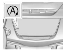
The automatic engine Stop/Start feature can be disabled and enabled by touching the A symbol. Auto Stop is enabled each time you start the vehicle.
