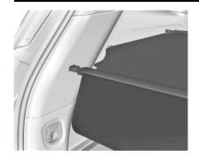
8. Insert the two rearward ends into the remaining slots on each side.
