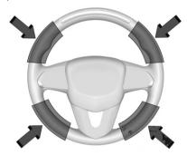
Any time the steering wheel light bar flashes red, resume manual steering immediately. The instrument cluster light , will also turn red and a message will display in the Driver Information Center (DIC). In addition, beeps will sound, or the Safety Alert Seat will vibrate. To view available settings from the infotainment home screen, touch Settings > Vehicle > Collision/Detection Systems. After you begin steering manually, then Super Cruise will disengage.
