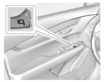
If equipped, press to power fold the mirrors. Press again to unfold.
