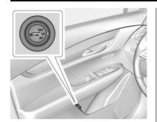
If equipped, the power liftgate switch is on the driver door. The vehicle must be in P (Park).
