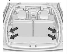
The vehicle has four cargo tie-downs in the rear compartment.
