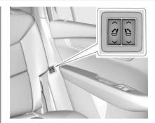
To fold the third row seatback from the second row seating area, press and hold the seatback folding switch on the right or left side of the second row seating area.
