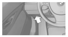
On the driver's side, there is a socket for onboard diagnosis to check components that are relevant for the vehicle's emission mix.
