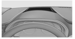
The protective glass of the Head-up display is located in the position marked.
