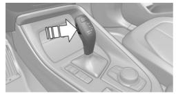
3. Push the selector lever in the desired direction, past a resistance point, if needed. The
