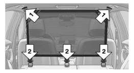
Hook the lower three hooks of the cargo area partition net into the three loops of the folded down rear backrest, arrow 2, raising the backrests slightly, if needed.
