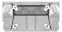
3. Use the hooks to hook the cargo area partition net into the upper lashing eyes in the cargo area, arrow 2.
