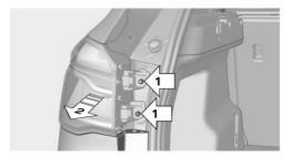
4. Detach the connector from the light bracket and detach the tail light wiring.
