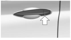
2. Unlock or lock the door lock using the integrated key.
