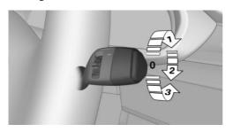
Turn the outer switch upward.
