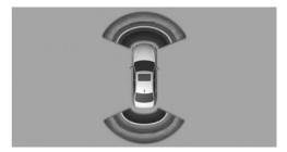
The approach of the vehicle to an object is shown on the Control Display. Objects that are farther away are already displayed on the Control Display before a signal sounds.
