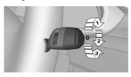
Turn the outer switch upward.
