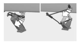
Take your hand away from the jack as soon as the jack is under load and continue turning the jack crank handle or lever with one hand. Make sure that the car jack foot stands vertically and at a right angle beneath the jacking point.
