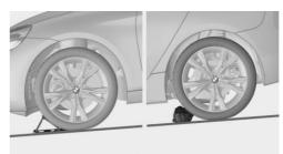
If you need to change a wheel on a slight downhill grade, place chocks and other suitable objects, for instance rocks, under the wheels of both the front and rear axles against the rolling direction.
