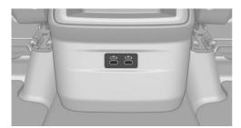
Two USB ports are located in the rear center console.
