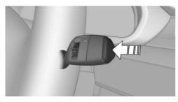
Press the button on the wiper lever.
