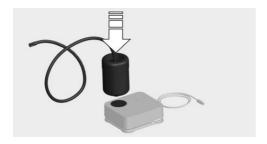
4. Screw the filler hose of the sealant bottle onto the tire valve of the faulty wheel.
