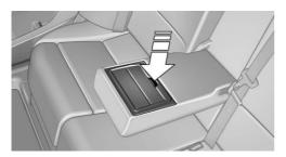
Pull the center armrest forward at the loop. To open: press the button.
