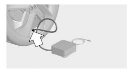
4. Insert the connector into the power socket in the vehicle interior.
