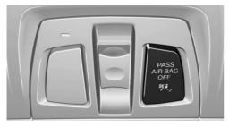
The indicator light for the front passenger airbags indicates the operating state of the front passenger airbags.
