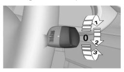
Turn the outer switch upward.
