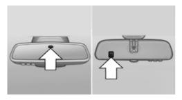
Photocells are used for control:
