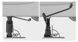
7. Crank the vehicle up, until the vehicle jack is with the entire surface on the ground and the relevant wheel is maximum 1.2 inches/3 cm above ground.
