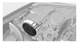
3. Detach the bulb holder directly to the rear, arrow 1, and remove.
