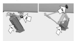
2. Insert the jack into the rectangular recess of the jacking point closest to the wheel to be changed.
