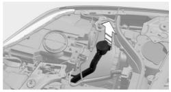
Turn the bulb socket counterclockwise and remove.
