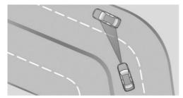
When you approach a curve the system may briefly report vehicles in the next lane due to the bend of the curve. If the system decelerates you may compensate it by briefly accelerating. After releasing the accelerator pedal the system is reactivated and controls speed independently.
