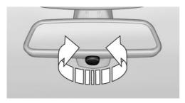
Turn the button to reduce the blinding glare by the interior mirror.
