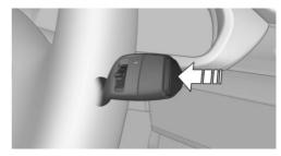
Press the button on the wiper lever.
