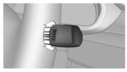
Turn the thumbwheel on the wiper lever.
