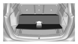
The cargo floor panel can be folded. To open the cargo floor panel, lift slightly and push toward the front.
