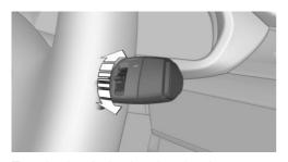
Turn the thumbwheel on the wiper lever.
