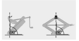
Make sure that the car jack foot stands vertically and perpendicularly beneath the jacking point after extending the vehicle jack.
