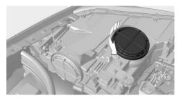
2. Detach the bulb holder directly to the rear, arrow 1, and remove.
