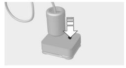
Let the compressor run for max. 10 minutes to fill the tire with sealing compound and achieve a tire inflation pressure of approx. 2.0 bar.
