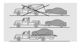
Your vehicle should be transported with a tow truck with a so-called spectacle lift or on a loading platform.
