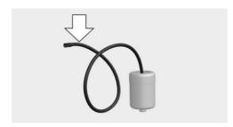
Slide the sealant bottle into the mount on the compressor housing, ensuring that it engages audibly.
