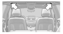
3. Insert each of the two top retaining pins of the cargo area partition net into the recep-
