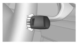
Turn the thumbwheel to adjust the interval period or sensitivity of the rain sensor.
