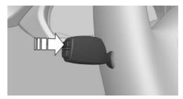
Press the button on the turn signal lever. Information is displayed in the Info Display of the instrument cluster. Pressing the button repeatedly displays additional information.
