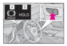
Turns the brake hold system on
