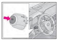
$Press\ the\ Automatic\ High\ Beam\ switch.$
