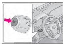
1 Press the Automatic High Beam switch.
