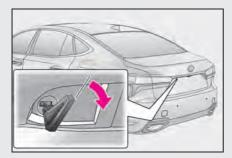
Turn the mechanical key clockwise to open.
