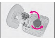
2 Turn the fuel tank cap slowly and remove it, then put it into the holder on the fuel filler door.
