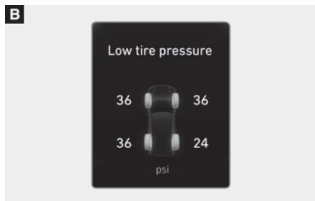
[A] : Low Tire Pressure Warning Light [B] : Low Tire Pressure Position and Tire Pressure Telltale
