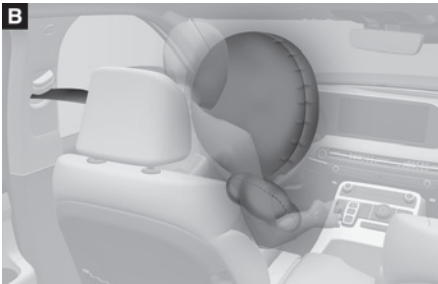
[B] : Driver's front air bag (2)
