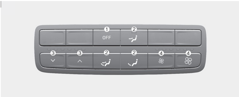
2nd row air conditioning control
