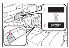
Each time the switch is pressed, the system changes between sport mode and normal mode.
