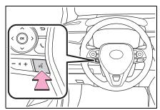
The voice command system and its list of commands can be operated. (→P.339)
