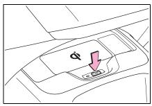
Place a portable device on the charging area with its charging surface facing down. While charging, the operation indicator light (orange) will be illuminated.
