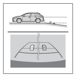
The distance guide lines will appear to be further from the vehicle than the actual distance. Because of
