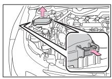
Engine compartment: type B fuse box
