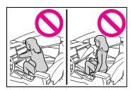
Do not allow a child to stand in front of the SRS front passenger airbag unit or sit on the knees of a front passenger.
