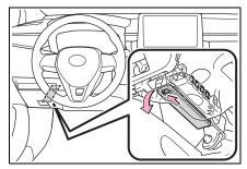
Remove the fuse with the pullout tool.
