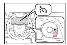
2 Accelerate or decelerate, with accelerator pedal operation, to the desired vehicle speed (at or above approximately 20 mph [30 km/h]) and press the "-SET" switch to set the speed.
