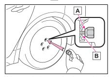
When replacing an aluminum wheel with a steel wheel, tighten the wheel nuts until the tapered portion A comes into loose contact with
