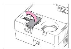
**7** Remove the power plug from the compressor.
