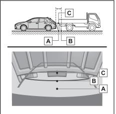
Visually check the surroundings and the area behind the vehicle. On the screen, it appears that a truck is parking at point B. However, in reality if you back up to point A, you will hit the truck. On the screen, it appears that A is closest and C is farthest away. However, in reality, the distance to A and C is the same, and B is farther than A and C.
