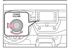
"POWER VOLUME" knob: Press to turn the audio/visual system on and off. The system turns on in the last mode used. Turn this knob to adjust the volume.
