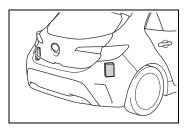
Do not attach accessories, stickers (including transparent stickers), aluminum tape, etc. to a sensor or its surrounding area on the rear bumper.
