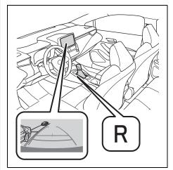
The rear view monitor system will be deactivated when the shift lever is shifted to any position other than R.
