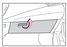
Pull up the lever to open the glove box.
