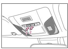
1 Turns the door position on/off When a door is opened while the door position is on, the lights turn
