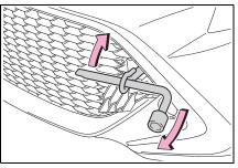
5 Securely attach cables or chains to the towing eyelet.
