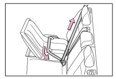
5 After installing the child restraint system, rock it back and forth to ensure that it is installed securely. (→P.53)
