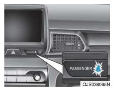
As a reminder to the front passenger, the front passenger's seat belt warning lights will illuminate for approximately 6 seconds each time you place the ignition switch to the ON position regardless of belt fastening. If you continue not to fasten the seat
