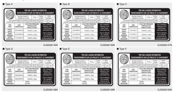
The label located on the driver's door sill gives the original tire size, cold tire pressures recommended for your vehicle, the number of people that can be in your vehicle and vehicle capacity weight.
