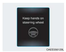
Keep hands on steering wheel If the driver takes their hands off the steering wheel for several seconds while the LKA system is activated, the system will warn the driver.
