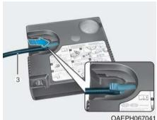
2. Connect the filling hose (3) directly into the compressor.
