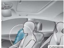
Your vehicle is equipped with a side air bag in each front seat. The purpose of the air bag is to provide the vehicle's driver and the front passenger with additional protection than that offered by the seat belt alone.
