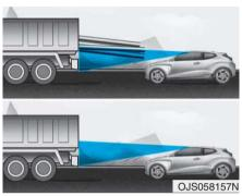
• Detecting the vehicle in front of you If the vehicle in front of you has cargo that extends rearward from the cab, or when the vehicle in front of you has higher ground clearance, additional special attention is required. The FCA system may not be able to detect the cargo extending from the vehicle. In these instances, you must maintain a safe braking distance from the rearmost object, and if necessary, depress the brake pedal to reduce your driving speed in order to maintain distance.
