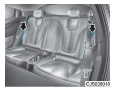
Move the seatbelt toward the outboard position before folding down the seatback to avoid the seatbelt system interfering with the seatback.
