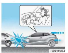
In certain low-speed collisions the air bags may not deploy. The air bags are designed not to deploy in such cases because they may not provide benefits beyond the protection of the seat belts.
