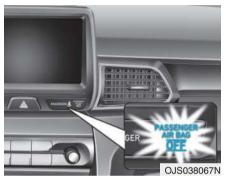
Your vehicle is equipped with an Occupant Classification System (OCS) in the front passenger's seat.
