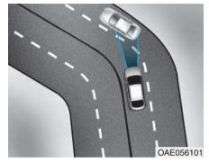
Forward Collision-Avoidance Assist system may recognize in the next lane or outside the lane when driving on a curved road.
