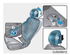
To reinstall the head restraint:
