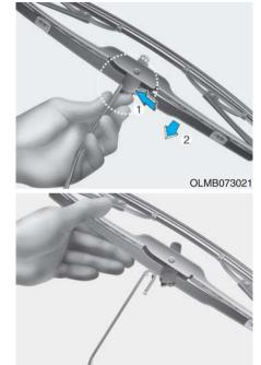
3. Press the clip (1) and slide the blade assembly downward (2).
