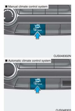
The defroster heats the window to remove frost, fog and thin ice from the interior and exterior of the rear window, while the engine is running.
