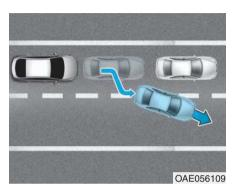
When driving in stop-and-go traffic, and a stopped vehicle in front of you merges out of the lane, the FCA system may not immediately detect the new vehicle that is now in front of you. In this case, you must maintain a safe braking distance, and if necessary, depress the brake pedal to reduce your driving speed in order to maintain a safe distance.
