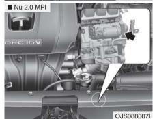
The engine number is stamped on the engine block as shown in the drawing.
