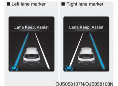
If the vehicle leaves a lane, the lane marker you cross will blink on the LCD display and the warning sound is provided. When the conditions below are met, LKA will be enable to assist steering.
