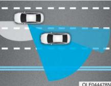
The Blind Spot Mirror (BSM) is a supplemental mirror that minimizes the driver's blind spot zone by expanding the field of view on the rear side of the vehicle.
