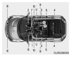
The SRS consists of the following components:
