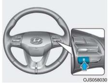
When the Smart Cruise Control system is ON, you can set and maintain the distance from the vehicle ahead of you without pressing the accelerator or brake pedal.
