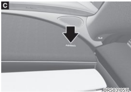
Ⓐ : Driver's front air bag, Ⓑ : Driver's knee air bag, Ⓒ : Passenger's front air bag
