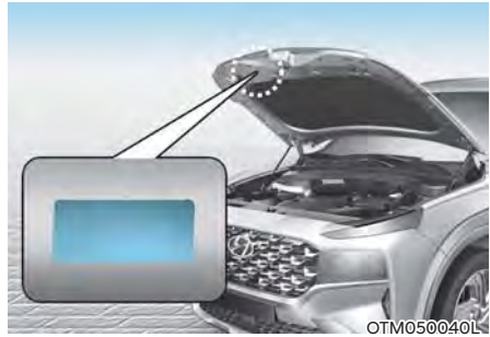
Air Conditioning refrigerant label
