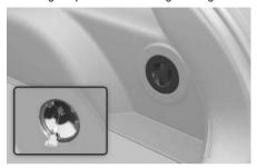
• If the charging connector does not disconnect after pulling the emergency cable, have your vehicle inspected by an authorized HYUNDAI dealer.
