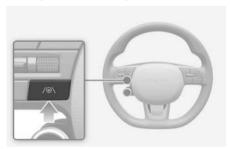
With the vehicle on, tap the Lane Driving Assist button located on the steering wheel to turn on Lane Following Assist. The gray or green (2) indicator light will illuminate on the instrument cluster.
