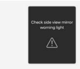
When the side view warning light is not working properly, the "Check Side View mirror Warning Light" warning message will appear on the instrument cluster for several seconds, and the master (A) warning light will illuminate on the instrument cluster. If this occurs, have your vehicle inspected by an authorized HYUNDAI dealer
