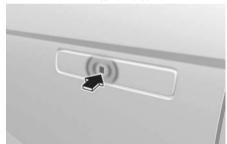
To lock your vehicle using the door handle touch sensor or the Smart Key:
