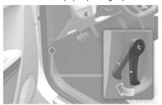
3 Go to the front of the vehicle, raise the hood slightly, push to the left the secondary hood release lever (1) inside of the hood center and lift the hood (2).
