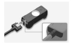
Check the arrow at the top of the connector, insert it in the correct direction into the ICCB coupling, and push it all the way towards the ICCB (Push it until the connector fits into the ICCB.).
