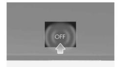
Press the **OFF** button to turn the climate control system off. You can still operate the mode and air intake buttons as long as the Start/Stop button is in the ON position.
