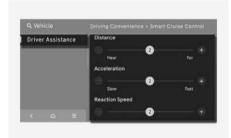
With the vehicle on, select Setup > Vehicle > **Driver Assistance > Driving Convenience >** Smart Cruise Control is selected from the infotainment system, you can change the vehicle distance, the acceleration, and the reaction speed manually.
