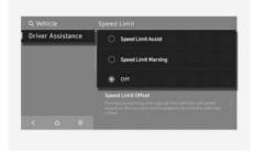
With the vehicle on, select or deselect Setup > Vehicle > Driver Assistance > Speed Limit from the infotainment system to set whether to use each function
