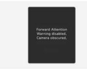
If there is an object right in front of the in-cabin camera or between you and the camera for a certain period of time Forward Attention Warning does not operate properly.
