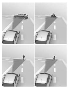
Forward Collision-Avoidance Assist may detect a vehicle, powered two-wheeler, pedestrian or cyclist in the next lane or outside the lane when driving on a curved road.
