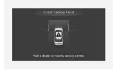
When Remote Smart Parking Assist is not working properly, the 'Check Parking Assist' warning message will appear on the infotainment system. If the message appears, stop using Remote Smart Parking Assist. and have the vehicle inspected by an authorized HYUNDAI dealer.
