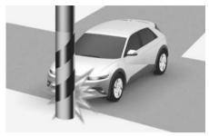
Air bags may not inflate if the vehicle collides with objects such as utility poles or trees, where the point of impact is concentrated and the collision energy is absorbed by the vehicle structure.
