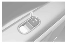
While the vehicle is running, press seat warmer switches located in each seats to warm the rear seat.
