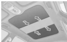
The power sunshade can only be operated when the Start/Stop button is in the ON or START position.
