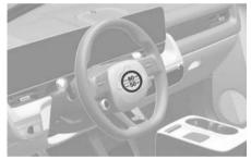
Detach the speed restriction label (1) from the sealant bottle (2), and place it in a highly visible place inside the vehicle such as on the steering wheel to remind the driver not to drive too fast
