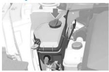
Check the fluid level in the washer fluid reservoir and add fluid if necessary. Plain water may be used if washer fluid is not available. However, use washer solvent with antifreeze characteristics in cold climates to prevent freezina.
