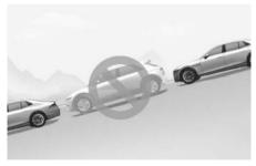
Park or exit manually when the vehicle is on inclines.
