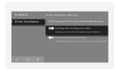
With the vehicle on, select or deselect **Setup** > Vehicle > Driver Assistance > Driver Attention Warning and then enable Leading Vehicle **Departure alert** in the infotainment system to set whether to use each function.
