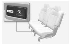
2 Open the power outlet cover by sliding it to the left, and connect the power plug of the electric device to the power socket.
