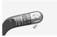
In the OFF position, pull the lever gently toward you to spray washer fluid on the windshield and to run the wipers 1-3 cycles. The spray and wiper operation will continue until you release the lever. If the washer does not work, you may need to add washer fluid to the washer fluid reservoir.
