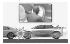
Front air bags are designed to inflate in a frontal collision depending on the severity of impact of the front collision.
