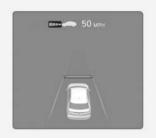
When Based on Driving Style is operating, the vehicle distance level and target distance will be displayed white based on the driving style.
