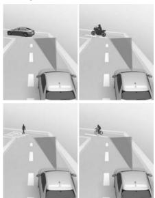
Forward Collision-Avoidance Assist may not detect other vehicles, powered two-wheelers, pedestrians or cyclists in front of you when driving on curved roads adversely affecting the performance of the sensors. This may result in no warning. braking or steering (if equipped) assist when necessary.
