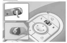
When the gear is shifted to the R (Reverse) position, the side view lever(s) will rotate downwards to aid with driving in reverse.
