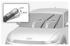
Within 20 seconds of turning off the vehicle, push down and hold the wiper lever to the MIST position for about 2 seconds until the wipers move to the top wipe position.
