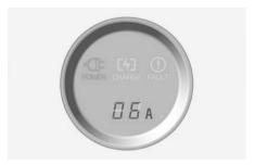
The ICCB automatically performs removable connector recognition upon power application. When recognition is completed normally, the current screen is displayed.
