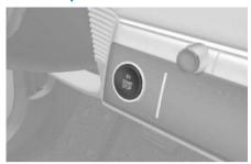
Whenever the front door is opened, the Start/Stop button will illuminate and will go off for a few seconds after the door is closed.
