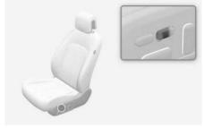
Press the front portion of the switch more than 0.5 seconds with the Start/Stop button is in the ACC or ON position.
