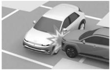
Front air bags may not inflate in side impact collisions, because occupants move in the direction of the collision, and thus in side impacts, front air bag deployment would not provide additional occupant protection.
