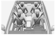
Your vehicle is equipped with driver's, front passenger's and rear passenger's (except rear center seat) pretensioner seat belts (retractor pretensioner). The pretensioner makes sure the seat belts fit tightly against your body in certain frontal or side collision(s). The pretensioner seat belts may be activated in some crashes where the frontal or side collision(s) is severe enough, together with the airbags.
