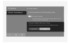
With the vehicle on, select Setup > Vehicle > Driver Assistance > Driving Safety > Forward Safety Warning Timing in the infotainment system to change the initial warning activation time for Forward Collision-Avoidance Assist. The warning time can be set to either "Standard" or "Late"
