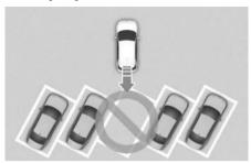
Remote Operation function may not operate properly in a diagonal parking space.
