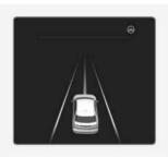
If the vehicle ahead and/or both lane markings are detected and your vehicle speed is below 110 mph (180 km/h), the green (⊖) indicator light appears on the cluster, and Lane Following Assist helps center the vehicle in the lane by assisting the steering wheel.
