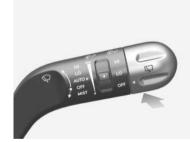
Push the lever away from you to spray rear washer fluid and to run the rear wipers 1-3 cycles. The spray and wiper operation continues until you release the lever.
