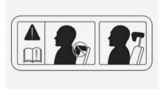
When sitting on the rear seat, do not adjust the height of the head restraint to the lowest position.
