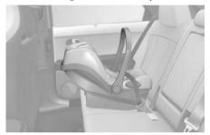
A rearward-facing Child Restraint System provides restraint with the seating surface against the back of the child. The harness system holds the child in place, and in an accident, acts to keep the child positioned in the Child Restraint Systems and reduce the stress to the fragile neck and spinal cord.
