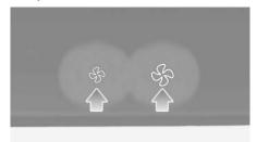
Press the \$\frac{1}{2}\$ button to increase fan speed and airflow. Press the \* button to decrease fan speed and airflow.
