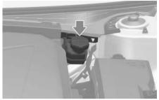
Check the fluid level in the reservoir periodically. The fluid level should be between MAX and MIN marks on the side of the reservoir. Before removing the reservoir cap and adding brake fluid, clean the area around the reservoir cap thoroughly to prevent brake fluid
