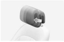
The head restraint may be adjusted forward by pulling the head restraint forward to the desired detent. To adjust the head restraint to it's furthest rearwards position, pull it fully forward to the farthest position and release it.
