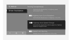
With the vehicle on, select Setup > Vehicle > **Driver Assistance > Driving Convenience >** Highway Auto Speed Change from the infotainment system to turn on Navigation based Smart Cruise Control and deselect to turn off the function.
