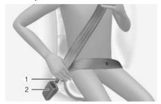
Pull it out of the retractor and insert the metal tab (1) into the buckle (2). There will be an audible "click" when the tab locks into the buckle.
