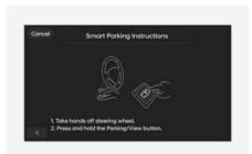
If Remote Smart Parking Assist cannot activate Remote Parking function, only the Smart Parking guide will be displayed on the infotainment system.
