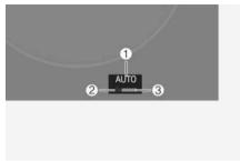
The instrument cluster displays 'AUTO' (1) when the smart regeneration system is on. Depending on the conditions, the system adjusts the regenerative braking level (2). The indicator light (3) illuminates when the vehicle recognizes a vehicle.
