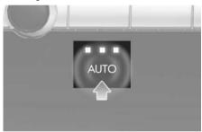
2 Press the temperature control button to set the desired temperature. If the temperature is set to the lowest setting, the air conditioning system operates continuously. After the interior has cooled sufficiently, adjust the button to a higher temperature set point whenever possible.
