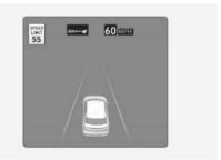
When driving at a speed higher than the displayed speed limit, the speed limit is displayed in red.
