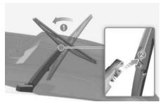
3 Install the new blade assembly by inserting the center part into the slot in the wiper arm until it clicks into place (3).
