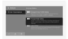
With the vehicle on, select Setup > Vehicle > Driver Assistance > Driving Safety > Forward/Side safety in the infotainment system to set whether to use each function.
