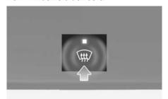
Press the front windshield defroster button (indicator light ON) to turn on the front windshield defroster. If the windshield defogging is set, outside (fresh) mode is automatically selected and the air conditioning turns on according to the detected ambient temperature.
