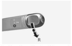
Use this position to drive the vehicle rearward. To shift the gear to R (Reverse), rotate the rotary gear shift dial to R (Reverse) while depressing the brake pedal.
