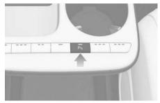
Press the Parking Safety (P™) button to turn on Forward/Reverse Parking Distance Warning. Press the button again to turn off the function.
