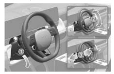
To adjust the steering wheel angle and height:
