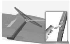
4 If the replacement is complete, put down the wiper arm onto the rear windshield, and turn the vehicle ON and operate the wipers to check the blade is installed correctly.
