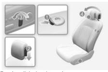
To reinstall the head restraint:
