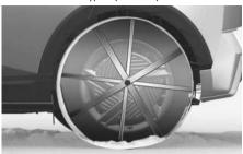
Since the sidewalls of radial tires are thinner than other types of tires, they may be damaged by mounting some types of tire chains on them. Therefore, the use of snow tires is recommended instead of tire chains.
