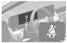
As a reminder to the driver, the driver's seat belt warning lights will illuminate for about 6 seconds each time the Start/Stop button is in the ON position regardless of belt fastening. If the seatbelt is not fastened, the warning chime will sound for about 6 seconds.
