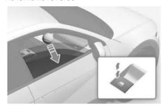
If a window senses any obstacle while it is closing automatically, it will stop and lower about 12 in. (30 cm) to allow the object to be cleared.
