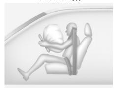
Upon deployment, tear seam molded directly into the pad cover will separate under pressure from the expansion of the air bags. Further opening of the covers allows full inflation of the air bags.
