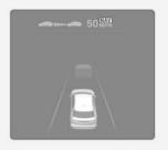
Navigation-based Smart Cruise Control standby If the operating conditions are satisfied, the green NAV indicator light illuminates.
