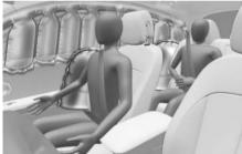
Your vehicle is equipped with a side air bag in each front seat. The purpose of the air bag is to provide the vehicle's driver and the front passenger with additional protection than that offered by the seat belt alone.
