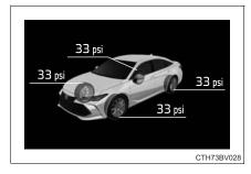
If the tire pressure drops below a predetermined level, the driver is warned by a screen display and a warning light. (→P. 459)
