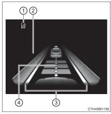
(2) Operation display of steering wheel operation support
