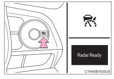
If the cruise control main switch is pressed and held for 1.5 seconds or more, the system turns on in constant speed control mode. (→P. 274)
