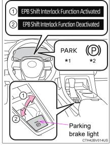
2 Turns automatic mode off (while the vehicle is stopped, press and hold the parking brake switch until a message is shown on the multi-information display)
