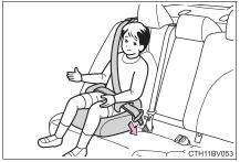
Check that the shoulder belt is correctly positioned over the child's shoulder and that the lap belt is as low as possible.  $(\rightarrow P. 30)$
