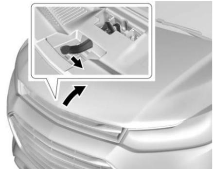
2. Go to the front of the vehicle and move the secondary hood release lever toward the driver side of the vehicle.
