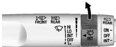
**INT** : Move the lever up to INT for intermittent wipes, then turn the
