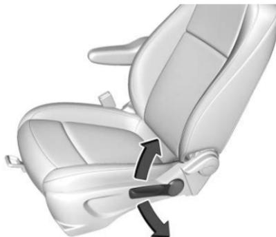
If available, move the lever up or down to manually raise or lower the seat.
