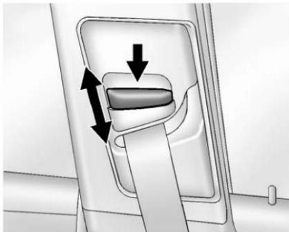
To move the shoulder belt height adjuster down, push down on the release button and move the height adjuster to the desired
