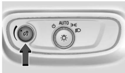
This feature adjusts the brightness of all illuminated controls. The instrument panel illumination control is next to the exterior lamp control.
