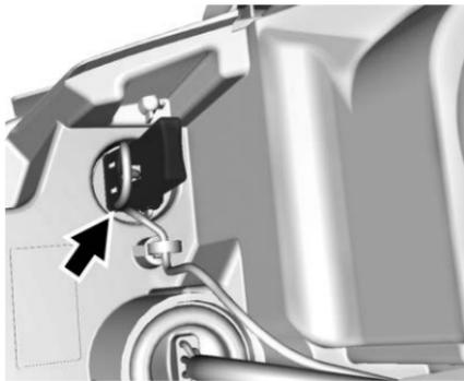
2. Remove the turn signal lamp bulb socket from the headlamp assembly by turning counterclockwise.
