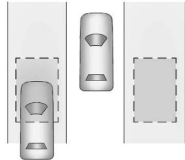
The SBZA sensor covers a zone of approximately one lane over from both sides of the vehicle, or 3.5 m (11 ft). The height of the zone is approximately between
