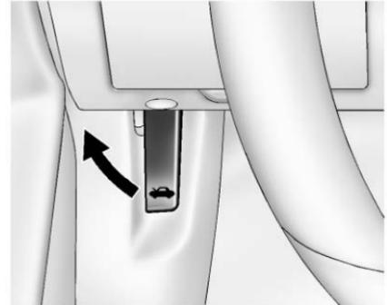
1. Pull the hood release handle inside the vehicle. It is on the lower left side of the instrument panel.
