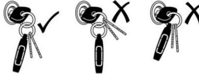
The ignition key and key rings, and RKE transmitter, if equipped, are designed to work together as a system to reduce the risk of unintentionally moving the key out of the RUN position. The ignition key has a small hole to allow attachment of the provided key ring. It is important that any replacement ignition keys have a small hole. See your dealer if a replacement key is required.
