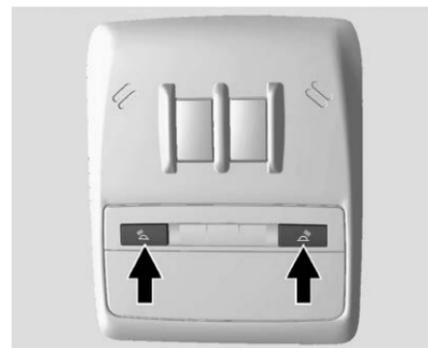
The front reading lamps are in the overhead console. These lamps come on when any door is opened,
