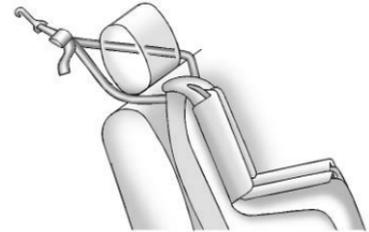
If the position you are using has an adjustable headrest or head restraint and you are using a dual tether, raise the headrest or head restraint and route the tether under the headrest or head restraint and around the headrest or head restraint posts.
