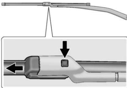
2. Press the release button on the top side of the wiper and pull the wiper blade out of the end of the wiper arm.
