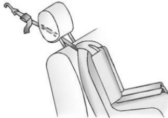
If the position you are using has an adjustable headrest or head restraint and you are using a single tether, raise the headrest or head restraint and route the tether under
