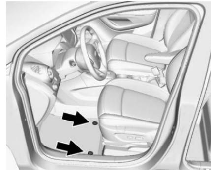
**Removing and Replacing the Floor Mats**
