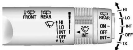
The windshield wiper/washer lever is on the right side of the steering column.
