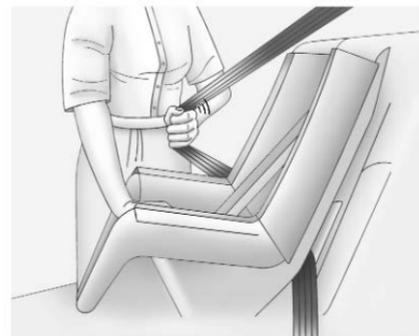
5. Pull the shoulder belt all the way out of the retractor to set the lock. When the retractor lock is set, the belt can be tightened but not pulled out of the retractor.
