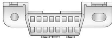
The DLC is under the instrument panel to the left of the steering wheel. Connecting devices that are not used to perform an Emissions Inspection/Maintenance test or to service the vehicle may affect vehicle operation. See *Add-On Electrical Equipment* ⇨ 165. See your dealer if assistance is needed.
