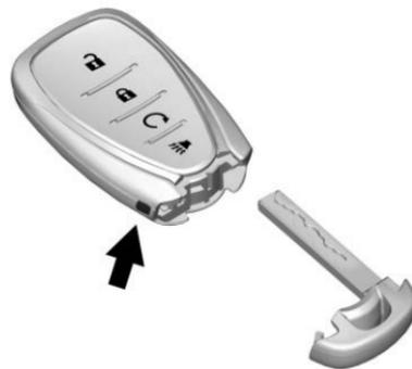
Press the key release button on the side of the RKE transmitter to release the key. Never pull out the key without pressing the button.
