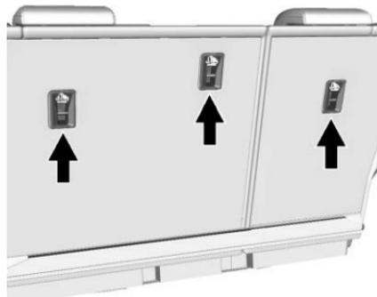
The top tether anchors are on the back of the rear seatbacks. Be sure to use an anchor located directly behind the seating position where the child restraint will be placed.
