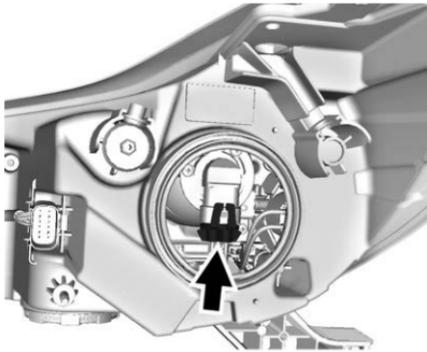
4. Disconnect the wiring harness connector from the bulb.
