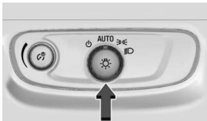
The exterior lamp control is on the instrument panel to the left of the steering column.
