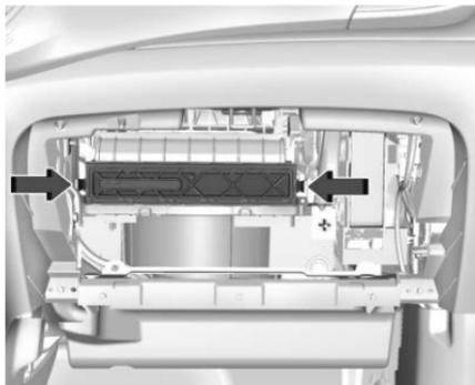
3. Open the filter cover by releasing tabs on both sides and pulling up the cover.
