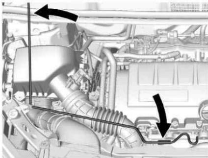
3. Lift the hood and release the hood prop from its retainer, above the radiator. Securely place the hood prop into the slot on the underside of the hood.
