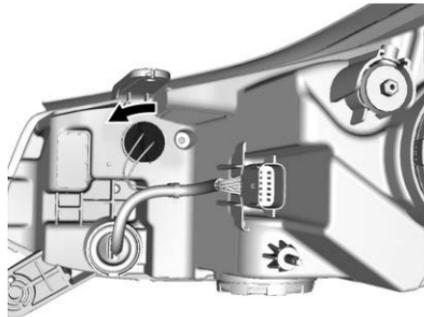
2. Remove the turn signal lamp bulb socket from the headlamp assembly by turning counterclockwise.
