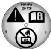
1. Remove the coolant surge tank pressure cap when the cooling system, including the coolant surge tank pressure cap and upper radiator hose, is no longer hot. Turn the pressure cap slowly counterclockwise about one-quarter of a turn. If you hear a hiss, wait for that to stop. This will allow any pressure still left to be vented out the discharge hose.
