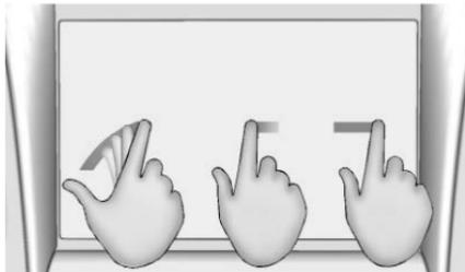
Fling or swipe is used to scroll through a list, or change page views. Do this by placing a finger on the screen then moving it rapidly up and down or right and left.
