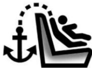
To assist in locating the top tether anchors, the top tether anchor symbol is on the trim near the anchor.
