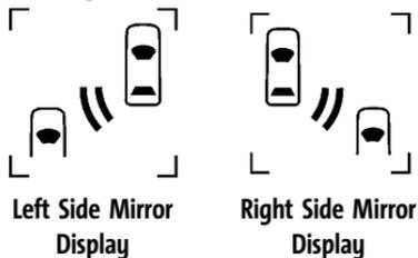
When the vehicle is started, both outside mirror SBZA displays will briefly come on to indicate the system is operating. When the vehicle is in a forward gear, the left- or right-side mirror display will light up if a moving vehicle is detected in that blind zone. If the turn signal is activated in the
