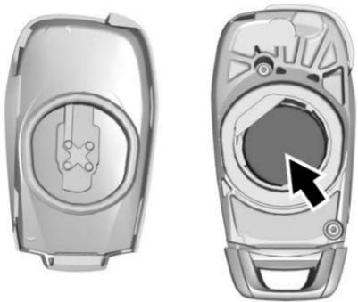
2. Remove the battery with a small tool by pushing it toward the top of the transmitter.
