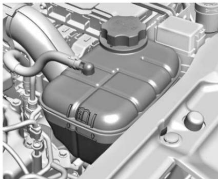
3. Fill the coolant surge tank with the proper mixture to the indicated level mark.
