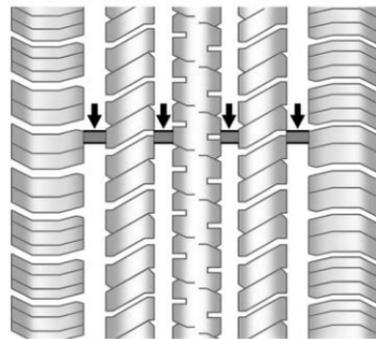
Treadwear indicators are one way to tell when it is time for new tires. Treadwear indicators appear when the tires have only 1.6 mm (1/16 in) or less of tread remaining. See *Tire Inspection* ⇨ 209 and *Tire Rotation* ⇨ 209 for additional information.
