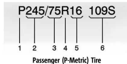
**(1) Passenger (P-Metric) Tire :** The United States version of a metric tire sizing system. The letter "P" as the first character in the tire size means a
