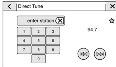
Access Direct Tune by touching the Tune icon on the AM, FM, or SXM screen to bring up the keypad. Navigate up and down through all frequencies using  $\llcorner$  or  $\lrcorner$ . Directly enter a station or channel using the
