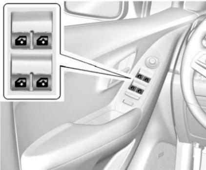
Power windows work when the ignition is on, in ACC/ACCESSORY, or when Retained Accessory Power (RAP) is active. See *Retained Accessory Power (RAP)* ⇨ 147.
