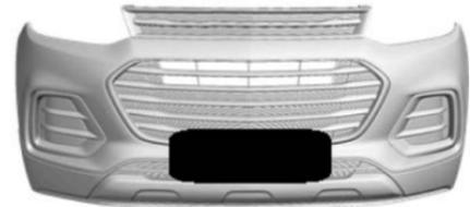
1. Center the winter grille cover and make sure that it is positioned correctly.
