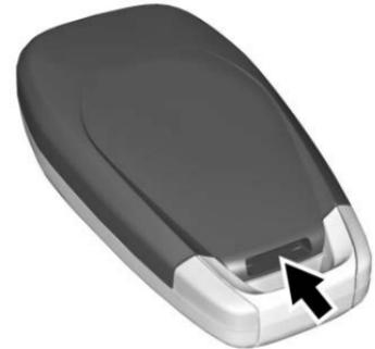
1. Separate the two halves of the transmitter by inserting a flat tool into the recess of the transmitter.
