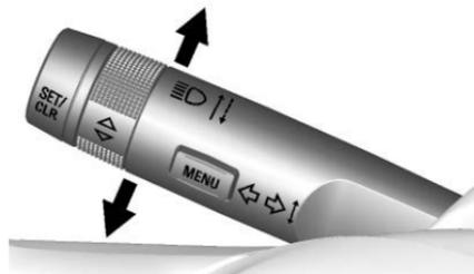
**☰** : Push the turn signal lever away from you and release, to turn the high beams on.
