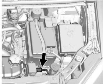
2. Open the hood and unwrap the electrical cord. The cord is in the driver side of the engine compartment, near the battery. It is shipped from the factory with a tie holding it in place. Use care in removing the tie so that the cord is not damaged. Check the heater cord for damage. If it is damaged, do not use it. See your dealer for a replacement. Inspect the cord for damage yearly.
