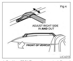
4. Position FRONT crossbar onto left and right roof rack rail; and adjust right support in and out until it fits securely into position. See Fig. 4.
