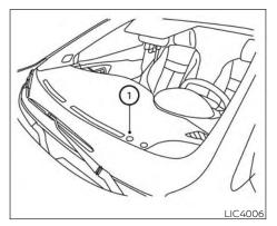
Be sure you do not put anything on top of the autolight sensor located in the top side ① of the instrument panel. The autolight sensor controls the autolight; if it is covered, the autolight sensor reacts as if it is dark out and the headlights will illuminate. If this occurs while parked with the engine off and the ignition switch placed in the ON position, your vehicle's battery could become discharged.
