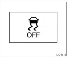
Push the VDC OFF switch again or restart the engine to turn on the system. For additional information, see "Vehicle Dynamic Control (VDC) system" (P. 5-134).
