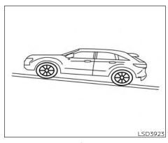
The Hill Start Assist function status can be checked in the Chassis Control mode in the vehicle information display (if so equipped). For additional information, see "Vehicle information display" (P. 2-24).
