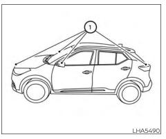
If dirt, rain or snow accumulates on any of the cameras (1), the MOD system may not operate properly. Clean the camera by wiping with a cloth dampened with a diluted mild cleaning agent and then wiping with a dry cloth.
