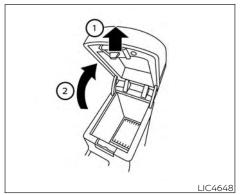
CONSOLE BOX (if so equipped) To open the console box, pull on the lever 1 and raise the lid 2.
