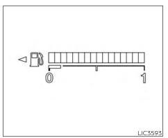
Type B (if so equipped) Refill the fuel tank before the gauge registers 0 (Empty).
