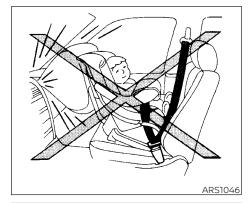
Even with the NISSAN Advanced Air Bag System, never install a rearfacing child restraint in the front seat. An inflating front air bag could seriously injure or kill your child. For additional information, see "Child restraints" (P. 1-21).
