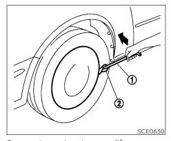
Removing wheel cover (if so equipped)
