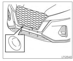
For alignment purposes, there are two marks on the radiator grille to indicate the correct position for each screw.
