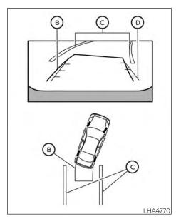
Slowly back up the vehicle adjusting the steering wheel so that the predicted course lines
