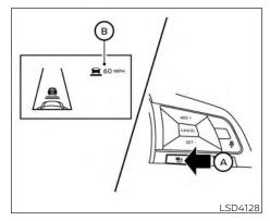
Operating vehicle-to-vehicle distance control mode
