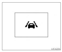
The Lane Departure Warning (LDW) switch is used to turn on and off the LDW system. When the LDW switch is pushed, the LDW system will turn on and the LDW indicator light will illuminate. When the LDW switch is pushed again, the LDW system will turn off and the LDW indicator light will turn off.
