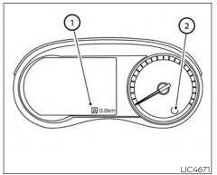
Type A (if so equipped) Odometer/Twin trip odometer
