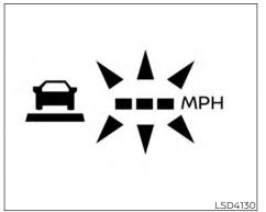
When the SET- switch is pushed under the following conditions, the system cannot be set and the ICC indicators will blink for approximately 2 seconds:
