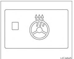
The heated steering wheel system is designed to operate only when the surface temperature of the steering wheel is below 68°F (20°C).
