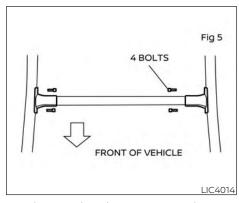
5. Make sure that the FRONT crossbar is in proper position with respect to the roof rack rail attachment positions, and loosely install all 4 bolts on FRONT crossbar using the T-30 TORX® screwdriver provided.
