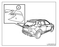
Request switches (if so equipped) for all doors and liftgate can be deactivated when the "Ext. Door Switch" setting is switched to OFF in "Vehicle Settings" of the vehicle information display (if so equipped). For additional information, see "Vehicle information display" (P. 2-24).
