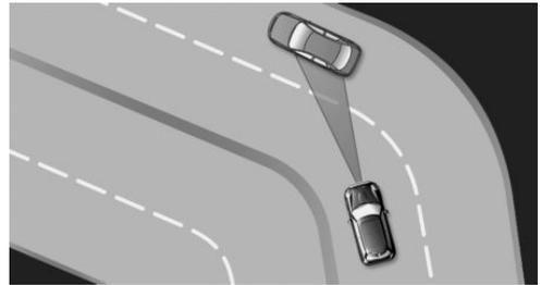
When you approach a curve the system may briefly report vehicles in the next lane due to the bend of the curve. If the system decelerates you may compensate it by briefly accelerating. After releasing the gas pedal the system is reactivated and controls speed independently.
