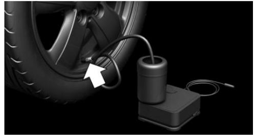
5. With the compressor switched off, insert the plug into the power socket inside the vehicle.
