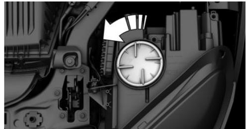
3. Turn the bulb holder counterclockwise, arrow 1, and remove, arrow 2.
