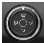
Turn the wheel to select the desired program or the desired intermediate setting.
