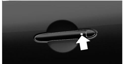
On the driver's or front passenger's door handle, press the button.
