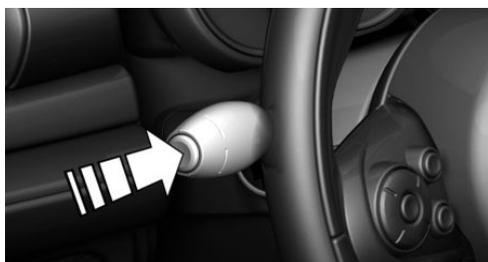
Press and hold button on signal lever.
