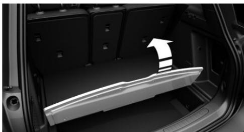
3. Grasp the cargo floor panel in the rear and fold up above the locking point of the upper position, refer to page 174.
