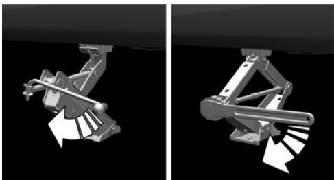
4. Take your hand away from the jack as soon as the vehicle jack is under load and continue turning the crank or lever with one hand.
