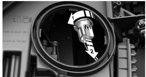
4. Press the bulb gently into the bulb holder, turn counterclockwise and remove.
