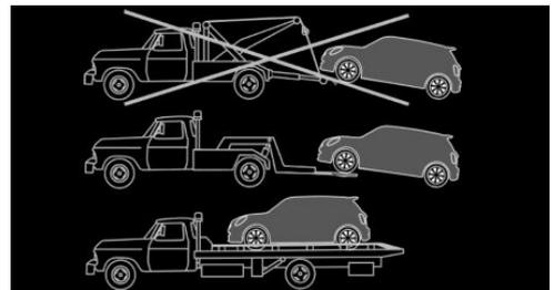
Have your vehicle transported with a tow truck with a so-called lift bar or on a flat bed.
