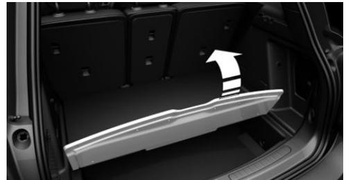
2. Place the MINI Picnic Bench on the part of the cargo area floor that is folded over and attach it using the four snaps.
