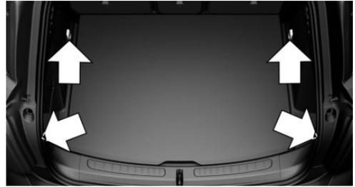
With storage package: to secure the cargo there are four lashing eyes in the cargo area.
