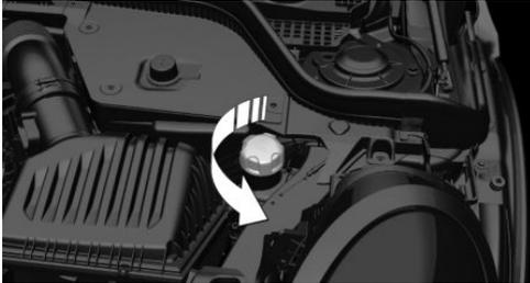
3. If the coolant is low, slowly add coolant up to the specified level; do not overfill.
