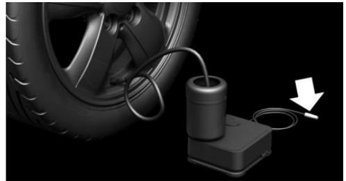
6. With the ignition turned on or the engine running, switch on the compressor.
