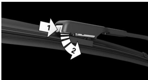
4. Attach a new wiper blade. The wiper blade must engage audibly.
