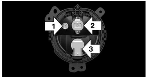
4. Pull the bulb out of the fixture.
