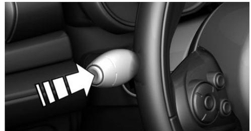
Press and hold button on blinker lever.
