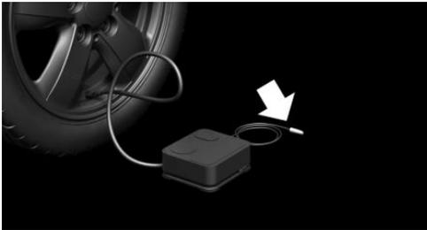
4. Correct the tire inflation pressure to at least 2.0 bar.
