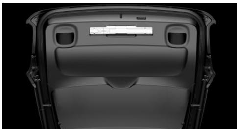
The warning triangle is located in the tailgate. To remove, loosen the brackets.
