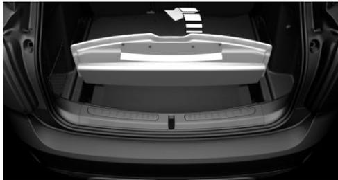
2. Grasp the MINI Picnic Bench in the middle and pull it back and up against the force of the magnets.
