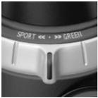
Turn MINI Driving Modes switch to the right until GREEN Mode is displayed in the instrument cluster.
