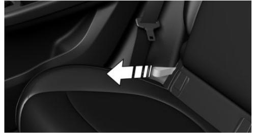
Pull the strap forward. The rear seat backrest folds forward.
