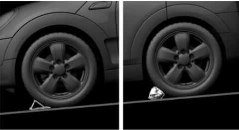
If you need to change a wheel on a slight downhill gradient, place chocks and other suitable objects, for example a rock, under the wheels of both the front and rear axles against the rolling direction.
