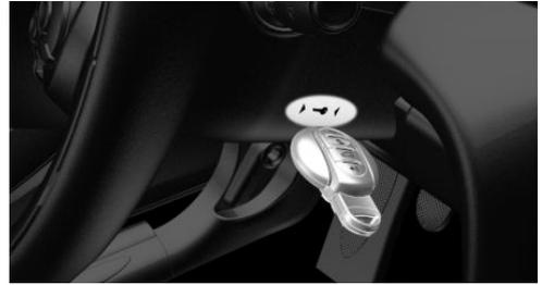
1. Hold the remote control as shown against the marked area on the steering column.
