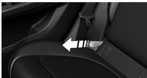
2. Fold the rear seat backrest rearward. The rear seat backrest first engages in the loading position.
