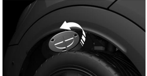
3. Unscrew the inner lid counterclockwise, and remove it.
