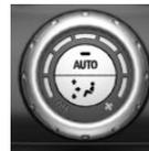
Turn wheel for air quantity to the left until the control switches off.
