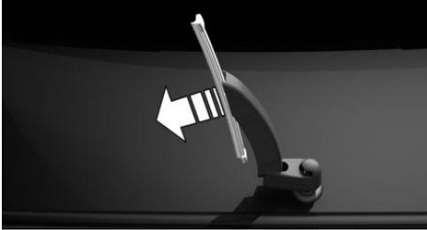
3. Attach a new wiper blade. The wiper blade must engage audibly.
