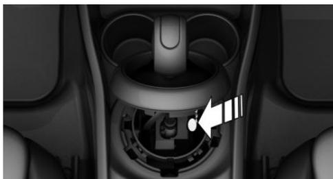
4. Move the selector lever slightly toward the rear; to do this press the button on the front of the selector lever. Release the release lever.
