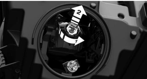
5. Pull the bulb out of the bulb holder.
