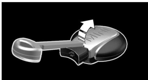
3. Slide the integrated key in the cover of the battery compartment and raise the cover.
