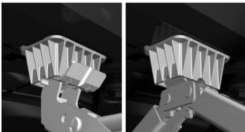
3. Extend the vehicle jack by turning the crank or lever clockwise.
