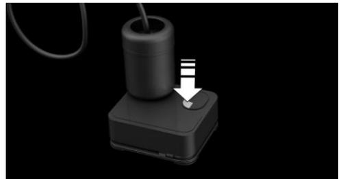
Let the compressor run for max. 10 minutes to fill the tire with sealant and achieve a tire inflation pressure of approx. 2.5 bar.
