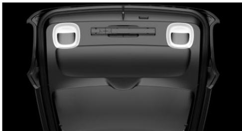
Recessed grips on the inside trim of the tailgate can be used to conveniently pull down the tailgate.
