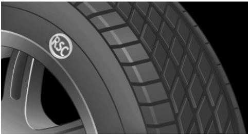
RSC label on the tire sidewall.
