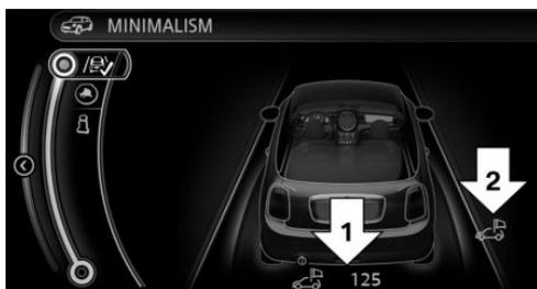
Color code green, arrow 1: distance traveled in the coasting driving condition. Symbol, arrow 2: coasting driving condition.
