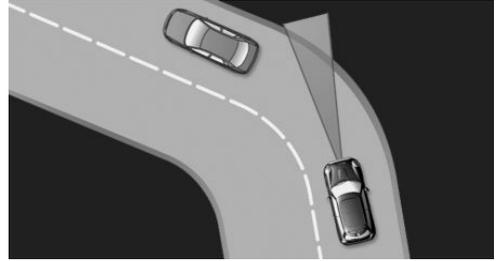
If the desired speed is too high for a curve, the speed is reduced slightly, although curves cannot be anticipated in advance. Therefore, drive into a curve at an appropriate speed.
