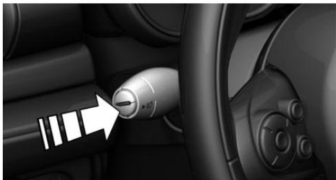
1. Depending on the equipment, turn the light switch into position
