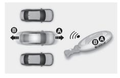
• Press and hold one of the Forward (🕪) or Backward (🕪) button on the smart key. Remote Smart Parking Assist will automatically control the steering wheel, vehicle speed and gearshift. The vehicle will move in the direction of the button pressed.
