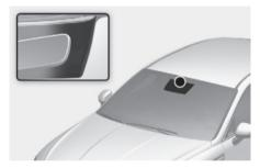
The rain sensor located on the upper end of the windshield glass senses the amount of rainfall and controls the interval of the wiping cycle.
