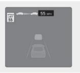
Manual Speed Limit Assist or Smart Cruise Control assists the vehicle to adjust its speed according to the speed limit. When the cruising speed is set as same as the speed limit, the vehicle automatically adjusts its speed if the speed limit changes. The function operates on the road which has a speed limit of 45 mph (70 km/h) or higher. When the function is active, the cruising speed on the instrument cluster appears in green.
