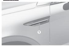
If the side repeater light (1) does not operate, have the system inspected by an authorized HYUNDAL dealer.
