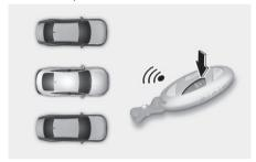
Press and hold the Remote Start button (♠) within 4 seconds until the engine starts.
