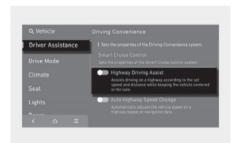
With the engine on, select or deselect **Setup > Vehicle > Driver Assistance > Driving Convenience** from the Settings menu to set whether to use each function.
