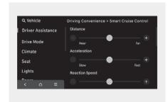
With the engine on, select **Setup** > **Vehicle** > **Driver Assistance** > **Driving Convenience** > **Smart Cruise Control** from the settings menu in the infotainment system to change Distance, Acceleration, Reaction Speed manually.
