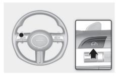
Press the Driving Assist (८७) button to turn Manual Speed Limit Assist off. The Speed Limit (४०००) indicator will go off.
