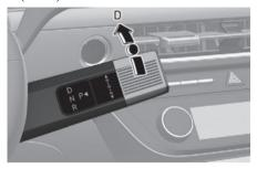
This is the normal forward driving position. The transmission automatically shift through an 8-gear sequence, providing the better fuel economy and power.
