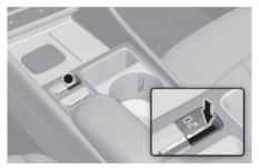
Press the Parking Safety (P<sub>4</sub>) button to turn on Parking Distance Warning. Press the button again to turn off the function.
