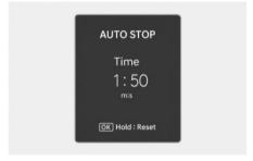
You can view the AUTO STOP elapsed time in the utility view. To view the elapsed time for AUTO STOP since the last reset, select Setup > Cluster > AUTO STOP elapsed time in the infotainment system.
