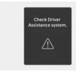
When Smart Cruise Control is not working properly, the "Check Driver Assistance system." warning message and the master (△) warning light will appear on the instrument cluster. Have your vehicle inspected by an authorized HYUNDAI dealer.
