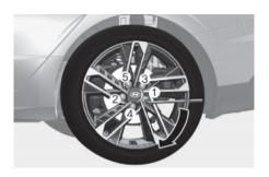
Check the tire pressure after installing the compact spare tire. The compact spare tire should be inflated to 60 psi (420 kPa).
