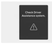
When High Beam Assist is not working properly, the "Check Driver Assistance system" warning message may appear, and the Awarning light may illuminate on the instrument cluster. Have the system inspected by an authorized HYUNDAI dealer.
