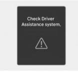
When Rear Cross-Traffic Collision-Avoidance Assist is not working properly, the "Check Driver Assistance system." warning message appears on the instrument cluster for several seconds, and the master (△) warning light illuminates on the instrument cluster. If this occurs, have your vehicle inspected by an authorized HYUNDAI dealer.
