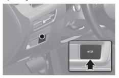
When the trunk is closed, press the trunk open button to open it.
