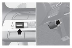
Press the INDswitch or depress the brake pedal to temporarily cancel Smart Cruise Control.
