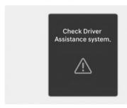
When Forward Collision-Avoidance Assist is not working properly, the "Check Driver Assistance system." warning message will appear, and the △, ♣ warning light will illuminate on the instrument cluster. Have your vehicle inspected by an authorized HYUNDAI dealer.
