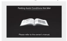
The "Parking Assist Conditions not met" message appears when Parking/View (E) button has been pressed and held while Remote Smart Parking Assist is in standby. After a while, press and hold the Parking/View (E) button again to see if Remote Smart Parking Assist works.
