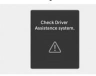
When Safe Exit Warning is not working properly, the "Check Driver Assistance system." warning message will appear on the instrument cluster for several seconds, and the master warning light (A) will appear on the instrument cluster. If this occurs, have your vehicle inspected by an authorized HYUNDAI dealer.
