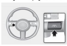
With the engine on, press and hold the Lane Driving Assist (IN) button located on the steering wheel to turn on and off. When Lane Keeping Assist is on, the INI indicator is on.
