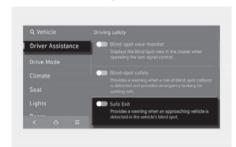
With the engine on, select **Setup** > **Vehicle** > **Driver Assistance** > **Driving Safety** > **Safe Exit** from the Settings menu to turn on Safe Exit Warning and deselect to turn off the function.
