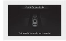
When Remote Smart Parking Assist is not working properly, the "Check Parking Assist" warning message will appear on the infotainment system. If the message appears, stop using Remote Smart Parking Assist, and we recommend that your vehicle be inspected by an authorized HYLINDAL dealer.
