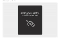
If the Driving Assist button, + switch, - switch or IIO switch is operated when Smart Cruise Control operating conditions are not satisfied, the "Smart Cruise Control conditions not met" will appear on the instrument cluster, and an audible warning will sound.
