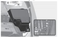
Pull the suspected fuse straight out.
