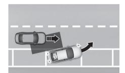
When you are driving forward out of a parking space, if Blind-Spot Collision-Avoidance Assist judges that there is a collision risk with an approaching vehicle in the blind spot, it can help avoid collision by applying the brake.
