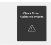
When Driver Attention Warning is not working properly, the "Check Driver Assistance system." warning message will appear on the instrument cluster for several seconds, and the master (△) warning light and the Inattentive Driving (⑤) warning light will appear on the instrument cluster. If this occurs, have your vehicle inspected by an authorized HYUNDAI dealer.
