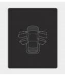
This warning appears if any door or hood or trunk is left open. The warning indicates which door is open on the cluster display.
