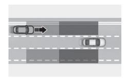
Blind-Spot Collision-Avoidance Assist helps detect and informs the driver that a vehicle is approaching at high speed from the blind spot area.
