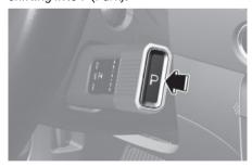
To shift the gear to P (Park), press the P button while depressing the brake pedal. If you turn the engine off in R (Reverse), N (Neutral) or D (Drive), the gear automatically shifts to P (Park).
