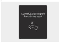
When the conversion from Auto Hold to EPB is not working properly, a warning sounds and a message appears.
