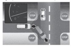
If a STOP, YIELD, or Roundabout sign is detected and the ISG system is deactivated by ISG inhibition at traffic signs, a message will appear on the cluster display (if equipped) when the "AUTO STOP" page on the instrument cluster is selected.
