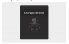
To warn the driver that emergency braking will be assisted, the "Emergency Braking" warning message appears and the (ﷺ) warning light blinks on the instrument cluster with a warning sound and the steering wheel vibrates.
