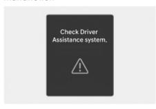
When Intelligent Speed Limit Assist is not working properly, the "Check Driver Assistance system." warning message will appear on the instrument cluster for several seconds, and the master (A) warning light and speed limit (D) warning light will appear on the instrument cluster. If this occurs, have your vehicle inspected by an authorized HYUNDAI dealer.
