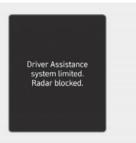
When the rear bumper around the rear corner radar or sensor is covered with foreign material, such as snow or rain, or installing a trailer or carrier, it can reduce the detecting performance and temporarily limit or disable Safe Exit Warning.
