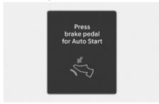
When the gear is shifted from N (Neutral) to R (Reverse), D (Drive), or Manual shift mode without the brake pedal depressed, a message appears on the cluster display. To activate auto start, depress the brake pedal.
