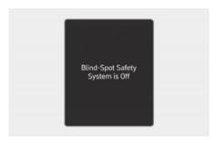
When the vehicle is restarted with Blind-Spot Collision-Avoidance Assist off, the "Blind-Spot Safety System is Off" message will appear on the instrument cluster.
