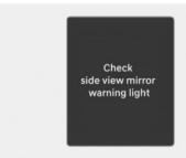
When the side view mirror warning light is not working properly, the "Check side view mirror warning light" warning message will appear on the instrument cluster for several seconds, and the master warning light (A) will appear on the instrument cluster. If this occurs, have your vehicle inspected by an authorized HYUNDAI dealer.
