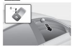
If a window senses any obstacle while it is closing automatically, it stops and lowers about 12 inches (30 cm) to allow the object to be cleared.
