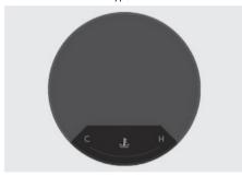
The engine coolant temperature gauge indicates the temperature of the engine coolant when the Engine Start/Stop button is in the ON position.
