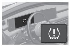
The TPMS Malfunction Indicator ( $\mbox{$\langle ! \rangle$}$ ) illuminates after it blinks for about one minute when there is a problem with the Tire Pressure Monitoring System.
