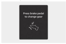
This message appears when the brake pedal is not depressed while shifting the gear.
