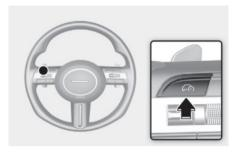
To turn Smart Cruise Control off, press the Driving Assist (A) button.
