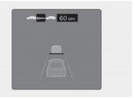
If you want to speed up temporarily without altering the set speed while Smart Cruise Control is operating, depress the accelerator pedal. While the accelerator pedal is depressed, the set speed, distance level and target distance will blink on the instrument cluster.
