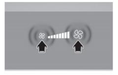
Press the right button to increase fan speed and airflow. Press the left button to decrease fan speed and airflow.
