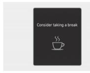
The "Consider taking a break" message will appear and the Inattentive Driving (\(\triangle\)) warning light will blink on the instrument cluster with a warning sound to suggest that the driver take a break, when the driver's attention level is below a certain level
