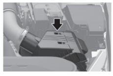
The air cleaner filter can be cleaned for inspection using compressed air.
