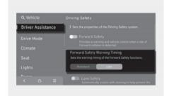
With the engine on, select Setup > Vehicle > Driver Assistance > Driving Safety > Forward Safety Warning Timing settings menu in the infotainment system to change the initial warning activation time for Forward Collision-Avoidance Assist. The warning time can be set to either Standard or Late
