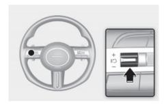
Press the IIO switch to temporarily pause the set speed limit. The set speed limit will turn off but the Speed Limit (ALMIT) indicator will stay on.
