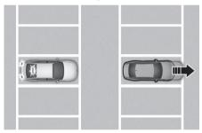
If a vehicle parked in front drives away from you, Leading Vehicle Departure Alert may alert you that the parked vehicle is driving away. When driving at a tollgate or intersection, etc.
