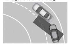
Blind-Spot Collision-Avoidance Assist may not operate properly when driving on a curved road. The function may recognize a vehicle in the same lane.
