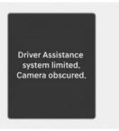
When the front windshield where the front view camera is located is covered with foreign material, such as snow or rain, it can reduce the detecting performance and temporarily limit or disable Intelligent Speed Limit Assist. If this occurs, the "Driver Assistance system limited.
