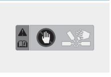
The electric motor for the cooling fan may continue to operate or start up when the engine is not running and can cause serious injury. Keep hands, clothing and tools away from the rotating fan blades of the cooling fan.
