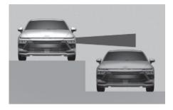
Blind-Spot Collision-Avoidance Assist may not operate properly when driving where the heights of the lanes are different. The function may not detect the vehicle on a road with different lane heights (underpass joining section, grade separated intersections, etc.). Always pay attention to road and driving conditions while driving.
