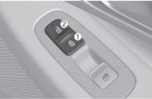
If any door is opened, the doors are not locked even though the lock switch (1) of the door is pressed.
