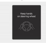
If the driver takes their hands off the steering wheel for several seconds, the "Keep hands on steering wheel" warning message appears on the instrument cluster, and an audible warning sounds in stages.
