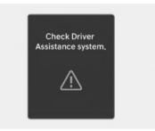
When Lane Keeping Assist is not working properly, the "Check Driver Assistance system." warning message and yellow Lane Keeping Assist (ﷺ) warning light appears on the instrument cluster. If this occurs, have your vehicle inspected by an authorized HYUNDAI dealer.
