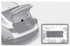
The Luggage compartment lamp turns on when the trunk is opened and off when the trunk is closed.
