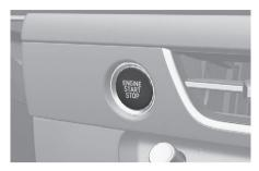
Whenever the front door is opened, the Engine Start/Stop button illuminates and goes off for a few seconds after the door is closed.
