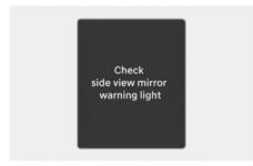
When the side view mirror warning light is not working properly, the "Check side view mirror warning light" warning message will appear on the instrument cluster for several seconds, and the master (△) warning light will appear on the instrument cluster. If this occurs, have your vehicle inspected by an authorized HYUNDAI dealer.
