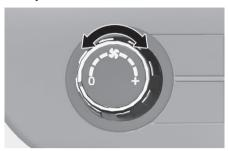
Turn the knob to the right to increase the fan speed and airflow. Turn the knob to the left to decrease fan speed and airflow. Setting the fan speed control knob to the "O" position turns off the fan.
