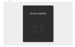
When the vehicle is stopped due to emergency braking, the "**Drive carefully**" warning message will appear on the instrument cluster.
