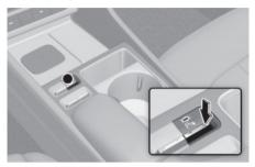
Press and hold the Parking Safety (P®) button more than 2 seconds, to turn the Parking Collision-Avoidance Assist on or off.
