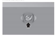
The mode selection button controls the direction of the air flow through the ventilation system.
