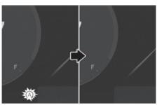
If the engine restarts automatically by the Early Engine Restart function, a message will appear on the cluster display (if equipped) when the "AUTO STOP" page on the instrument cluster is selected.
