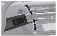
The wheels and transmission are not engaged.
