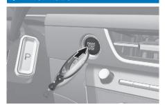
If the smart key battery is weak or the smart key does not work correctly, press the Engine Start/Stop button with the smart key.
