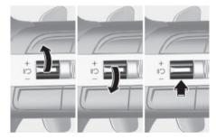
To resume Manual Speed Limit Assist after the function was paused, operate the +, -, or IIO switch.
