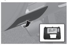
Inside the fuse panel cover, you can find the fuse/relay label describing fuse/relay names and ratings.
