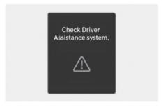
When Lane Following Assist is not working properly, the **Check Driver Assistance system.** warning message will appear on the instrument cluster for several seconds, and the master (△) warning light appears on the instrument cluster. If this occurs, have your vehicle inspected by an authorized HYUNDAI dealer.
