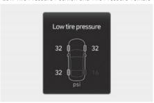
When the Tire Pressure Monitoring System warning indicator ((!)) is illuminated and a warning message appears on the cluster display, one or more of your tires is significantly under-inflated. The Low Tire Pressure Position Telltale will indicate which tire is significantly under inflated by illuminating the corresponding parking light.
