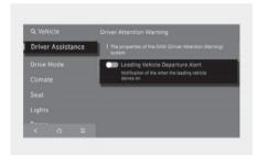
With the engine on, select Setup > Vehicle > Driver Assistance > Driver Attention Warning and then enable Leading Vehicle Departure Alert in the infotainment system to use the function.
