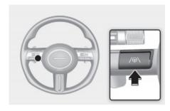
With the engine on, shortly press the Lane Driving Assist button located on the steering wheel to turn on Lane Following Assist. The gray or green ((a)) indicator light will appear on the instrument cluster.
