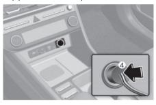
7. With the engine ON, switch on the compressor and let it run for about 5-7 minutes to fill the sealant up to proper pressure. (refer to the "Tires And Wheels" section in chapter 2). The inflation pressure of the tire after filling is unimportant and can be checked/corrected later.
