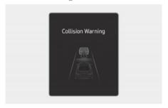
To warn the driver of a collision, the "Collision Warning" warning message appears and the (ﷺ) warning light blinks on the instrument cluster with a warning sound and the steering wheel vibrates.
