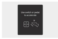
In traffic, your vehicle will stop if the vehicle ahead of you stops. Also, if the vehicle ahead of you starts moving, your vehicle will start as well. In addition, after the vehicle has stopped and a certain time have passed, the "Use switch or pedal to accelerate" message will appear on the instrument cluster. Depress the accelerator pedal or operate the + switch, - switch or || > switch to start driving.
