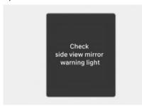
When the side view mirror warning light is not working properly, the "Check side view mirror warning light" warning message appears on the instrument cluster for several seconds, and the master (△) warning light illuminates on the instrument cluster. If this occurs, have your vehicle inspected by an authorized HYUNDAI dealer.
