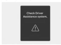
When Highway Driving Assist is not working properly, the "Check Driver Assistance system." warning message and yellow Lane Keeping Assist (A) warning light appears on the instrument cluster. If this occurs, have your vehicle inspected by an authorized HYUNDAI dealer.
