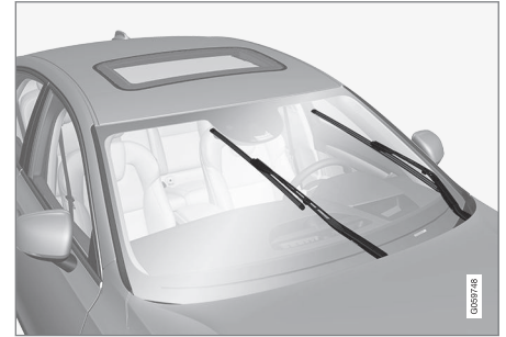
Windshield wipers in the service position.
