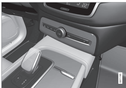
Overview of small gear selector, where it is not possible to deactivate the shiftlock.
