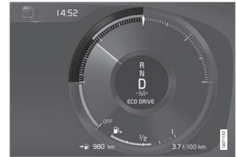
Eco gauge in 12" instrument panel*.
