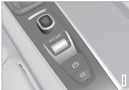
Start knob in the tunnel console.
