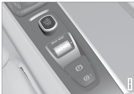
Start knob in the tunnel console.
