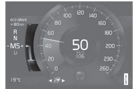
Eco gauge in 8" instrument panel.
