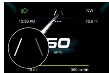
Left Lane Limit Detected
