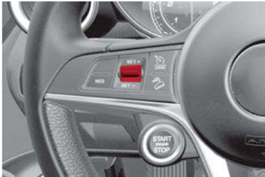
Set Switch Location
