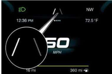
Left Lane Limit Detected
