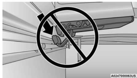
Improper Clamp Position
