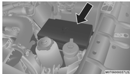
Power Distribution Center Location
