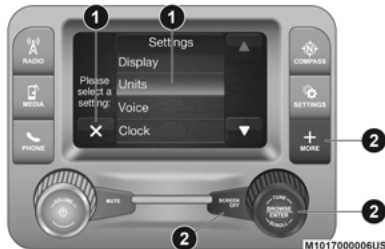
Uconnect 3 With 5-inch Display Buttons On The Touchscreen And Buttons On The Faceplate
