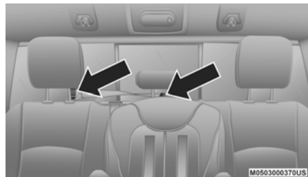
Tether Strap Through Center Tether Strap Loop And Attached To Outboard Tether Strap Loop
