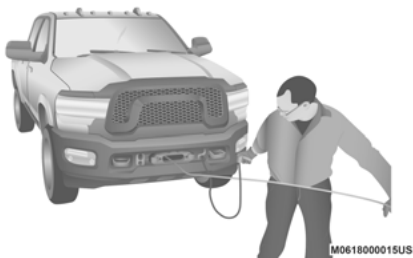
Pulling Synthetic Rope Under Tension
