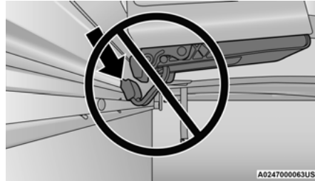
Improper Clamp Position
