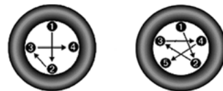
Four And Five Lug Nuts/Bolts Torque Pattern
