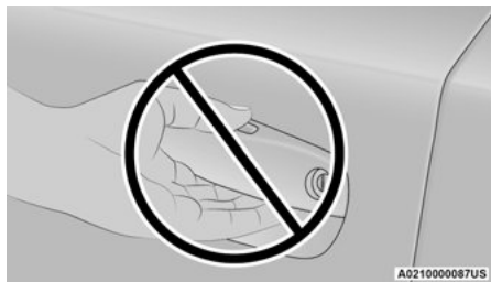
Do NOT Grab The Handle When Locking
