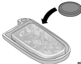
Key Fob Battery Replacement
