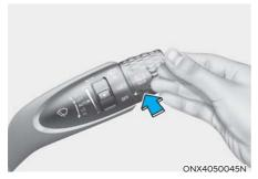
Push the lever away from you to spray rear washer fluid and to run the rear wipers 1-3 cycles. The spray and wiper operation continues until you release the lever.
