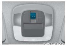
The sunroof can be operated when the ignition switch is in the ON or START position.
