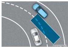
Blind-Spot Collision-Avoidance Assist may not detect a vehicle in an adjacent lane when driving on curves and may not activate a warning or brake your vehicle.
