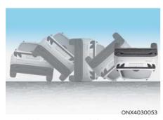
Front airbags may not inflate in rollover accidents because front airbag deployment would not provide additional occupant protection.
