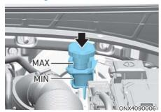
Check the fluid level in the reservoir periodically. The fluid level must be between the MAX and the MIN marks on the side of the reservoir.
