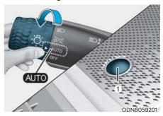
The headlights and parking lights are turned ON or OFF automatically depending on the amount of daylight as measured by the ambient light sensor ① in front of the instrument panel.
