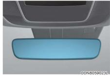
When the engine is running, the glare from vehicle headlights behind you is automatically controlled by the sensor mounted in the rearview mirror.
