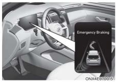
To warn you of a potential collision, the warning light on the side view mirror may blink, a warning message may appear on the instrument cluster, and an audible warning may sound.
