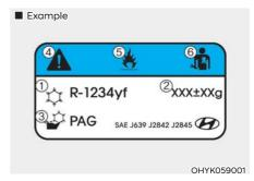
Each symbol and specification on the air conditioning refrigerant label is represented as the following:
