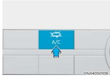
Press the A/C button to turn on the air conditioning system (indicator light ON). Press the button again to turn off the air conditioning system.
