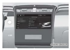
Vehicle Settings in the infotainment system provide user options for the settings including door lock/unlock, convenience features, and driver assistance.
