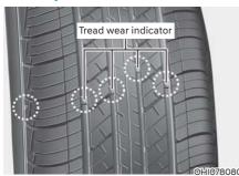
If the tire is worn evenly, a tread wear indicator appears as a solid band across the tread. This shows there is less than 1/16 inch (1.6mm) of tread left on the tire. Replace the tire when this happens.
