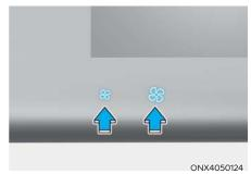
Press the **\$** button to increase fan speed and airflow. Press the **\$** button to decrease fan speed and airflow.
