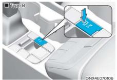
Press the Parking Safety (P<sub>M</sub>) button to turn on Parking Distance Warning.
