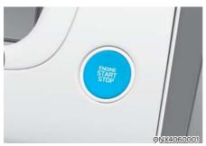
Whenever the front door is opened, the Push Button Start ignition switch illuminates and goes off 30 seconds after the door is closed.
