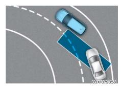
Blind-Spot Collision-Avoidance Assist may detect a vehicle in the same lane when driving on curves and activate a warning or brake your vehicle.
