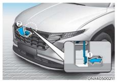
Go to the front of the vehicle, raise the hood slightly, push up the secondary latch ① inside of the hood center and lift the hood ②.
