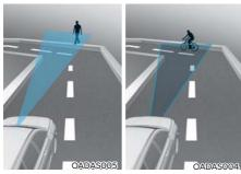
If a vehicle, pedestrian, or cyclist is detected in the next lane or outside the lane when driving on a curve, Forward Collision-Avoidance Assist may warn you and may brake your vehicle even when not needed.
