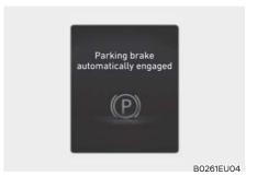
Parking brake automatically engaged
