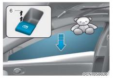
If a window senses any obstacle while it is closing automatically, it stops and lowers approximately 12 inches (30 cm) to allow the object to be cleared.
