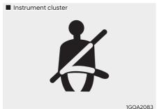
As a reminder to the driver, the seat belt warning light illuminates for about 6 seconds each time the ignition is moved to the ON position regardless of seat belt fastening. If the seat belt is not fastened, a warning chime sounds for 6 seconds.
