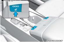
While the engine is running, press the switch to cool the driver's seat or the front passenger's seat.
