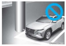
Remote Smart Parking Assist performance may be reduced when there is a narrow object, pillar (e.g. circular shaped or edge of a square shaped pillar, etc.), or pillar surrounded by objects such as fire extinguisher near the parking space.
