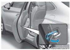
Doors without an outside key hole can be locked as follows:
