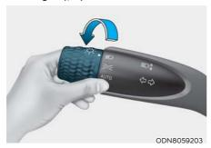
The headlight, parking light, license plate light, and instrument panel light are turned ON.
