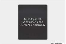
Auto Stop is Off. Shift to P or N and start engine manually
