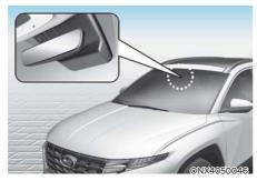
Auto defogging reduces the likelihood of fogging up the inside of the windshield by sensing moisture on the inside of the windshield.
