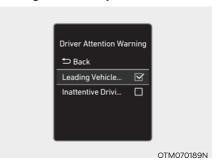
If **Leading Vehicle Departure Alert** is selected, the function informs you when a detected vehicle in front departs from a stop.
