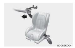
Pull the shoulder portion of the seat belt all the way out. When the shoulder portion of the seat belt is fully extended, it shifts the retractor to the Automatic Locking (child restraint) mode.
