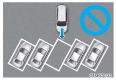
Remote Smart Parking Assist cannot park your vehicle in angled or diagonal spaces. Even if your vehicle can enter the parking space, do not use Remote Smart Parking Assist because the function does not operate normally.
