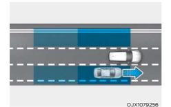
Blind-Spot Collision Warning helps detect and warns you that a vehicle is in the blind spot area.
