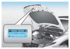
You can find out which air conditioning refrigerant is applied to your vehicle on the label located inside of the hood.
