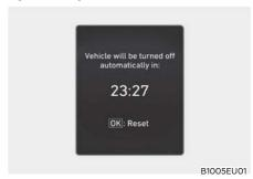
When all the conditions are satisfied, the Vehicle Auto-Shut Off operates and turns the engine off automatically after 60 minutes.
