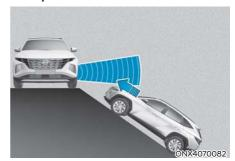
Rear Cross-Traffic Collision Warning may be limited when your vehicle is on a uphill or downhill slope, and may not detect any vehicle approaching from the left or right. If this occurs, the function may activate a warning even when not needed.
