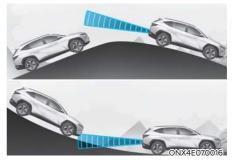
Blind-Spot Collision Warning may not detect a vehicle in an adjacent lane or may incorrectly detect the ground or another object when driving on hills and activate a warning.
