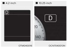
The Transmission Shift Indicator in the upper corner of the cluster display indicates the current gear or P (Park).
