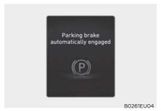
Parking brake automatically engaged When EPB is applied while Auto Hold is activated, a warning sounds and a message appears.
