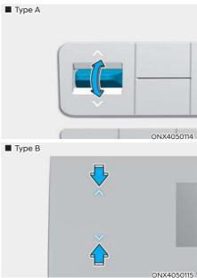
The temperature setting increases when you toggle up or press the UP arrow on the touchscreen (if equipped).
