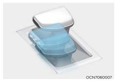
To shift into DS mode, move the shift lever from D (Drive) to the left, without upshifting to the + or downshifting to the -.
