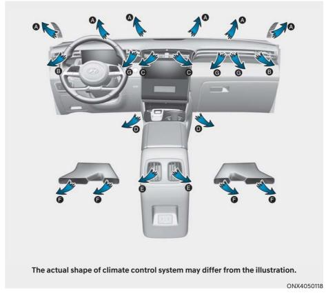
The mode selection button controls the direction of the air flow through the ventilation system.
