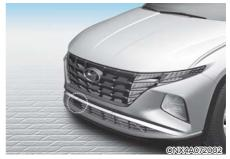
The front radar is mounted behind the front grill.
