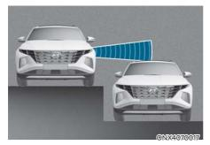
Blind-Spot Collision Warning may not operate properly when driving where the heights of the lanes are different. The function may not detect a vehicle on a road with a different lane height (underpass joining section, grade separated intersections, etc.) and not activate a warning.
