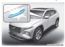
Welcome system helps keep the driver visible by turning on vehicle lights when the driver approaches the vehicle.
