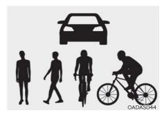
The illustration above shows the image the front view camera is capable of detecting as a vehicle, pedestrian, and cyclist.
