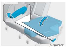
Pull up the seatback folding lever, then fold the seat toward the front of the vehicle.
