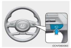
Press the II D button to temporarily cancel the set speed limit. The set speed turns off, but the Manual Speed Limit Assist ( O I IMIT ) indicator light stays on.
