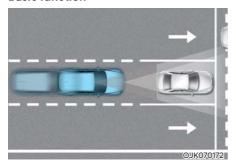
Forward Collision-Avoidance Assist uses the front view camera and front radar to help detect a vehicle, a pedestrian, or a cyclist ahead on the road. The function may warn you with a warning message on the instrument cluster and an audible warning if a collision is imminent. If necessary, it may assist with braking your vehicle to help reduce collision speed and avoid a collision.
