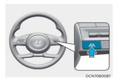
With the ignition switch ON, press the Lane Driving Assist button on the steering wheel to turn on Lane Following Assist. The white or green A indicator light illuminates on the instrument cluster.
