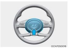
To sound the horn, press the area indicated by the horn symbol on your steering wheel (see illustration). The horn operates only when this area is pressed.
