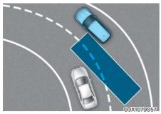
Blind-Spot Collision Warning may not detect a vehicle in an adjacent lane when driving on curves and may not activate a warning.
