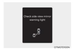
When the side view mirror warning light is not working properly, the "Check side view mirror warning light" warning message may appear, and the warning light may illuminate on the instrument cluster. Have the vehicle inspected by an authorized HYUNDAI dealer.
