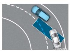
Blind-Spot Collision Warning may detect a vehicle in the same lane when driving on curves and activate a warning.
