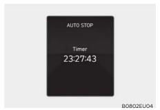
Displays the elapsed time of engine stop by the Idle Stop and Go system.
