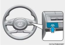
With the ignition switch ON, press and hold the Lane Driving Assist button located on the steering wheel to turn on and off. The white or green indicator light illuminates on the instrument cluster when the function is
