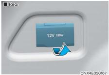
The power outlet is designed to provide power for mobile phones or other devices designed to operate with vehicle electrical systems. The devices should draw less than 180 watts with the engine running.
