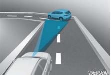
On curves, Smart Cruise Control may not detect a vehicle in the same lane, and may accelerate to the set speed. Your vehicle speed may be reduced if a vehicle is detected in an adjacent lane and your vehicle speed may rapidly decrease when a vehicle ahead is detected suddenly.
