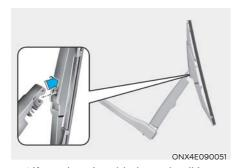
3. Lift up the wiper blade, and pull it out.
