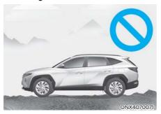
Remote Smart Parking Assist may cancel when your vehicle slips or cannot move due to road conditions such as pebbles or fragmented stones.
