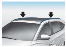
Your vehicle may come equipped with roof rack rails. If your vehicle is equipped with roof rack rails, you can add roof rack crossbars as an accessory (not shown).
