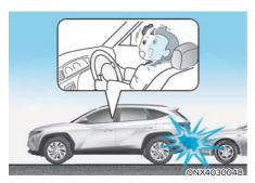
Front airbags are not designed to inflate in rear collisions, because occupants are moved backward by the force of the impact.
