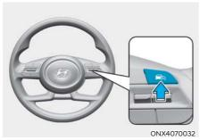
Press the Driving Assist ( ) button to to turn off Cruise Control. The Cruise ( CRUISE) indicator light goes off.
