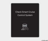
When Smart Cruise Control is not working properly, the "Check Smart Cruise Control system" warning message may appear, and the /\(\hat{\text{warning light may}}\) illuminate on the instrument cluster. Have the vehicle inspected by an authorized HYUNDAI dealer.
