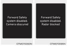
When the front view camera or front radar is covered or blocked, Forward Collision-Avoidance Assist may be temporarily limited or disabled.
