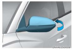
To fold the side view mirror, grasp the housing of the mirror and then fold it toward the rear of the vehicle.
