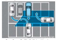
Rear Cross-Traffic Collision Warning may detect vehicles that are parking or pulling out near your vehicle (e.g. leaving beside your vehicle, parking or pulling out behind your vehicle, approaching your vehicle making a turn). If this occurs, the function may activate a warning even when not needed.
