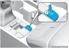
Press the Parking/View button ① to turn on Rear View Monitor.
