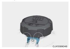
Make sure that the tiny protrusions inside the coolant cap is securely interlocked.
