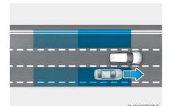
Blind-Spot Collision-Avoidance Assist helps detect and warns you that a vehicle is in the blind spot area.
