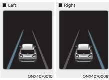
If the vehicle detects it is departing from the projected lane ahead, the green indicator light and the lane line blink on the instrument cluster depending on which direction your vehicle is veering, and an audible warning sounds.
