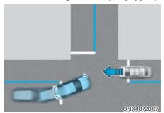
This function uses the front view camera and front radar to help detect oncoming vehicles in an adjacent lane when turning left at an intersection with the turn signal on. If there is a collision risk, it may assist with braking your vehicle to help avoid a collision.
