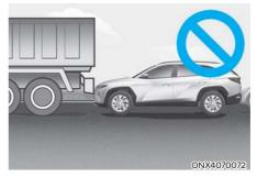
Do not use Remote Smart Parking Assist around vehicles with higher ground clearance such as bus or truck, etc. The other vehicle may not be detected and may cause a collision.
