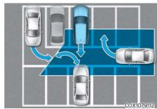
Rear Cross-Traffic Collision-Avoidance Assist may detect vehicles that are parking or pulling out near your vehicle (e.g. leaving beside your vehicle, parking or pulling out behind your vehicle, approaching your vehicle making a turn). If this occurs, the function may activate a warning and brake your vehicle even when not needed.
