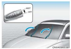
This vehicle has a "hidden" wiper design that cannot be lifted when in their bottom resting position.
