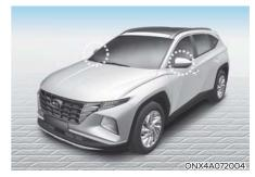
The wide-side view cameras are mounted to the bottom of the side view mirrors outside your vehicle.
