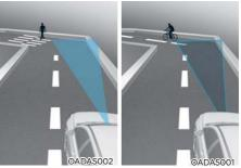
Forward Collision-Avoidance Assist may not detect other vehicles, pedestrians, or cyclists in front of you when driving on a curve and may not activate a warning or brake your vehicle when needed.
