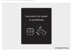
In traffic, your vehicle stops if the vehicle ahead of you stops. Also, if the vehicle ahead of you starts moving, your vehicle starts moving as well. In addition, after your vehicle has stopped and a certain amount of time has passed, the "Use switch or pedal to accelerate" message appears on the instrument cluster. Depress the accelerator pedal or push the +/- switch or || > button to start driving.
