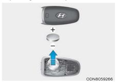
Battery type: CR2032 To replace the battery:
