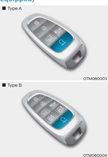
You can start the vehicle using the Remote Start button on the smart key.
