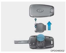
Battery type: CR2032 To replace the battery:
