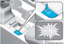
With the driver's door, hood, and liftgate (vehicles equipped with shift button) closed, press the AUTO HOLD switch. The white AUTO HOLD indicator comes on and the system is in standby.
