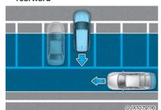
Rear Cross-Traffic Collision Warning may detect vehicles passing by behind you when parking in reverse into a parking space. If this occurs, the function may activate a warning even when not needed.
