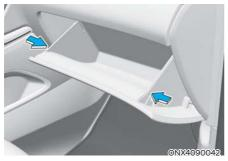
2. Push in both sides of the glove box to release the glove box stopper pins and allow the glove box to hang open.
