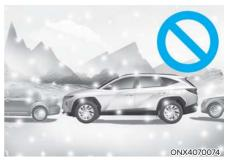
Snow may interfere with sensor operation, or Remote Smart Parking Assist may cancel if the road is slippery where you are parking.
