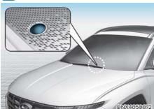
Never place anything near the sensor to ensure better control of the heating and cooling system.
