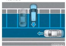
Rear Cross-Traffic Collision-Avoidance Assist may detect vehicles passing by behind you when parking in reverse into a parking space. If this occurs, the function may activate a warning and brake your vehicle even when not needed.
