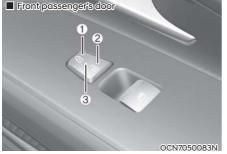
When pressing the  $(\frac{}{1})$  portion ① on the switch, all vehicle doors are locked.
