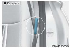
Routing the seat belt webbing through the rear seat belt guides helps keep the seat belts from being trapped behind or under the seats.
