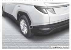
These ultrasonic sensors are mounted near the rear wheels outside your vehicle.
