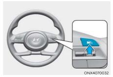
Press the Driving Assist ( ) button to turn off Manual Speed Limit Assist off. The Manual Speed Limit Assist ( ) LIMIT) indicator light turns off.
