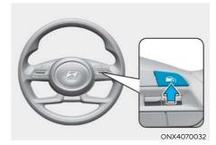
Press the Driving Assist ( ) button to turn off Smart Cruise Control.
