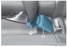
Insert the tongue plate ① into the buckle ② until an audible "click" is heard, indicating the latch is locked. Pull the shoulder portion of the belt to snug the belt across your hips and remove slack. Make sure the seat belt is not twisted.
