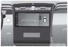
Surround View Monitor uses the widefront view camera, wide-side view camera, and wide-rear view camera to display images around your vehicle through the infotainment system screen when parking.
