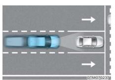
Forward Collision-Avoidance Assist uses the front view camera to help detect a vehicle, a pedestrian, or a cyclist ahead on the road. The function may warn you with a warning message on the instrument cluster and an audible warning if a collision is imminent. If necessary, it may assist with braking your vehicle to help reduce collision speed and avoid a collision.
