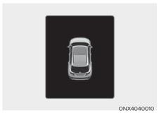
If the driver turns off the engine when the sunroof is not fully closed, the warning chime sounds for several seconds and the sunroof open warning appears on the cluster display.
