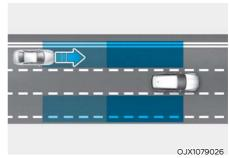
Blind-Spot Collision-Avoidance Assist helps detect and warns you that a vehicle is approaching at high speed from the blind spot area.
