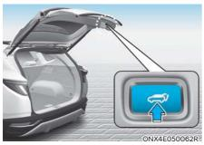
Press the power liftgate open/close button. The liftgate opens or closes automatically.
