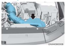
The air cleaner filter can be cleaned for inspection using compressed air. Do not attempt to wash or rinse it, because water can damage the filter. If soiled, replace the air cleaner filter.
