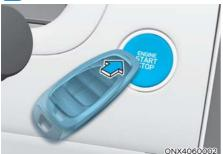
If the smart key battery is weak or the smart key does not work correctly, press the Push Button Start ignition switch with the smart key.
