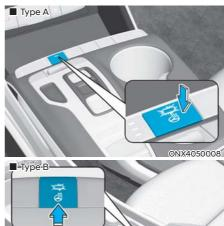
When the ignition switch is in the ON position or when the engine is running, press the steering wheel heater button to
