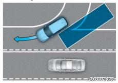
Blind-Spot Collision Warning may not detect a vehicle in an adjacent lane when the road merges or divides and may not activate a warning.
