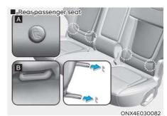
A: Lower Anchor Position IndicatorB: Lower Anchor
