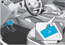
To release EPB (Electronic Parking Brake):
