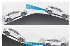
Blind-Spot Collision-Avoidance Assist may not detect a vehicle in an adjacent lane or may incorrectly detect the ground or another object when driving on hills and activate a warning or brake your vehicle.
