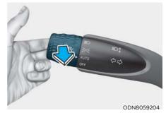
To flash the high beam headlight, pull the lever toward you, then release the lever. The high beams remain ON as long as you hold the lever.
