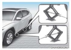
7. Place the jack at the designated jacking position under the frame closest to the tire you are changing. The jacking positions are plates welded to the frame with two notches. Never jack at any other position or part of the vehicle to prevent the vehicle slipping off of the jack or damaging the vehicle.
