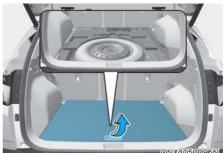
You can place a first aid kit, a reflector triangle (front tray), tools, etc. in the box for easy access.
