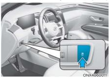
Electronic Stability Control helps stabilize the vehicle during cornering maneuvers.
