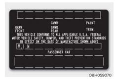
The certification label is located on the driver's door sill at the center pillar and shows the maximum allowable weight of the fully loaded vehicle. This is called the GVWR (Gross Vehicle Weight Rating). The GVWR includes the weight of the vehicle, all occupants, fuel, and cargo.
