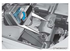
Pull down the lever to the UNLOCK @ position.
