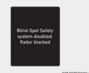
If the rear corner radar is blocked or covered, or when the rear bumper around the rear corner radar or sensor is covered by any foreign material, such as snow, rain, or dirt, or when a trailer or hitch mounted carrier is installed, the detecting performance may decrease and temporarily limit or disable Blind-Spot Collision Warning.
