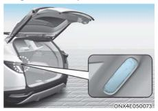
The cargo area lamp turns on when the liftgate is opened and off when the liftgate is closed.
