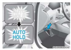
2. When you stop the vehicle completely by depressing the brake pedal, Auto Hold maintains the brake pressure to hold the vehicle stationary. The indicator changes from white to green.
