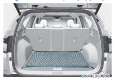
To keep items from shifting in the cargo area, use the 4 holders located in the cargo area side trim to attach the cargo net.
