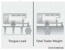
Check if the total load is within limits at a public scale. If a public scale is not available, add the estimated weight of your cargo load to the weight of your trailer (as specified by your trailer manufacturer). In addition, measure the tongue load with an appropriate scale or tongue gauge, or estimate it based on the cargo distribution.
