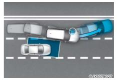
Blind-Spot Collision-Avoidance Assist may brake your vehicle if there is a detected collision risk when changing lanes.
