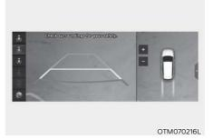
If Rear View Parking Guidance is selected, the parking guideline appears on the right side of the Surround View Monitor screen when the rear view is displayed.
