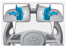
The paddle shifter is available when the shift button is in the D (Drive) position.
