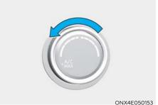
The MAX A/C mode is used to cool the inside of the vehicle faster. Air flow is directed toward the upper body and face.
