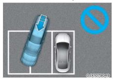
If Remote Smart Parking Assist is used, when parking in a parking space with a vehicle only on one side, your vehicle may cross the parking marking on the opposite side of the parked vehicle.
