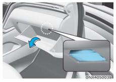
The glove box lamp turns on when the glove box is opened.
