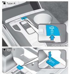
Press the ISG OFF button to turn off the ISG system. The ISG OFF button indicator illuminates. To use the system, press the ISG OFF button again.
