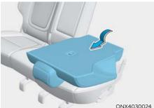
Pull the remote seatback release handle ① located on either side in the rear cargo area.
