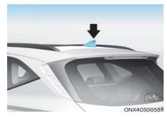
The shark fin antenna receives transmitted data (e.g. AM/FM, GPS).
