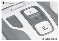
Depress the brake pedal whenever pressing the shift button to change gear or shifting to P (Park).
