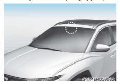
The rain sensor located on the upper end of the windshield glass senses the amount of rainfall and controls the interval of the wiping cycle.
