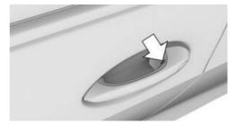
With your finger, touch and hold the grooved surface on a closed door handle without grasping the door handle.
