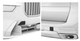
The thread for the towing eye is located behind a cover on the front and rear bumper.
