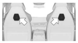
The mounts for attaching optional accessories are located behind the marked covers, as are the USB ports.
