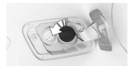
3. Place the fuel filler cap in the bracket on the fuel filler flap.
