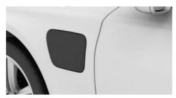
The charging socket flap is located in front on the left side of the vehicle.
