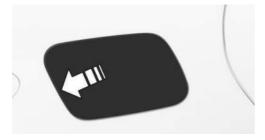
2. Open the fuel filler cap counterclockwise.
