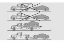
Have vehicle transported on a loading platform or use a tow dolly.
