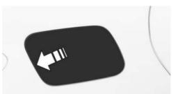
2. Open the fuel filler cap counterclockwise.
