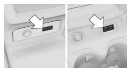
Two USB ports are located in the center console in the rear at one of the marked positions. Properties:
