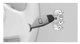
Turn the outer switch upward.
