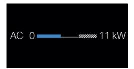
The shaded area indicates a limitation in the charging capacity that can occur, for instance due to the connected charging infrastructure.
