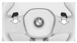
The shift paddles for Boost Control are located on the steering wheel.
