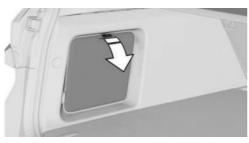
The onboard vehicle tool kit is located in the left storage compartment of the cargo area. Pull the lug.
