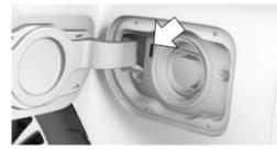
The charging status is indicated on the indicator light on the charging socket.
