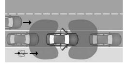
Two radar sensors in the rear bumper monitor the area behind the vehicle.
