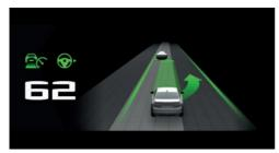
An example with active Driver Assistance: the indicator and warning lights for the distance control and the Lane Change Assistant indicate a lane change to the next lane. At the same time, the lane change to the next lane is shown with animation in the Assisted View.
