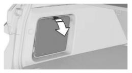
Storage for the first-aid kit is provided in the left storage compartment of the cargo area. Pull the lug.
