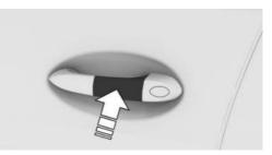
Hold the smartphone NFC antenna directly at the center of the driver's door handle. The po-
