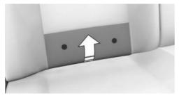
2. Slide the lug on the outside of each backrest into the gap.
