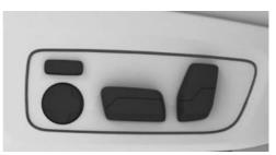
The switches for setting the seats are located on the front seats.
