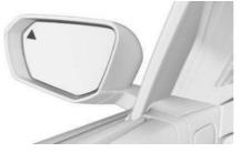
The warning light in the exterior mirror flashes if the rear sensors detect other vehicles when the vehicle is reversing. Display in the Park Distance Control view
