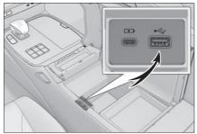
When connecting a USB flash drive, connect it directly to the USB port.
