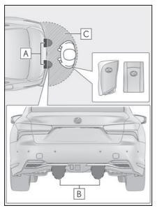
1 While carrying an electronic key, stand within the smart access system with push-button start operation area, approximately 11.8 to 19.7 in. (30 to 50 cm) from the rear bumper.
