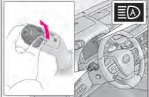
1 Press the Automatic High Beam switch.
