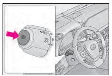
Press the Automatic High Beam switch.
