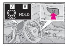
Turns the brake hold system on
