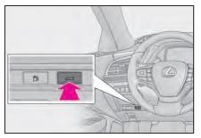
Press the trunk opener switch. The trunk lid will fully open.
