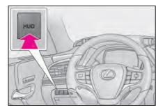
Pressing the switch turns the head-up display on/off.
