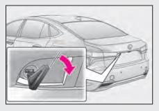
Turn the mechanical key clockwise to open.
