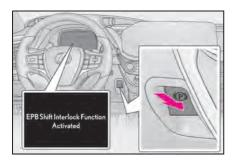
While the vehicle is stopped, press and hold the parking brake switch until a message is shown on the multi-information display.
