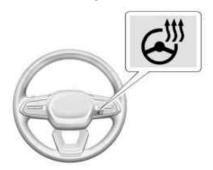
: Press to turn the heated steering wheel on or off. An indicator next to the button is lit when the feature is turned on.
