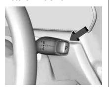
The vehicle uses an electric drive unit. The shift pattern is displayed on the front of the shift lever. The selected gear position will illuminate red on the shift lever, while all others will be displayed in white. If the shift is not immediate, as in very cold conditions, the indicator on the shift switch may blink until it is fully engaged.
