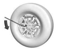
3. Turn the wheel wrench counterclockwise to loosen all the wheel nuts, but do not remove them yet.
