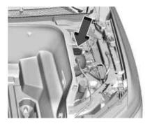
After the system has completely cooled, check that the coolant level in the reservoir.
