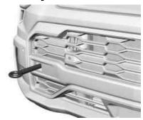
If the vehicle is equipped with a tow eye, only use the tow eye to pull the vehicle onto a flatbed car carrier from a flat road surface. Do not use the tow eye to pull the vehicle from snow, mud, sand, or a ditch.
