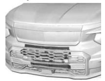
The vehicle may have a shutter system that automatically closes the frontal cooling openings. This system promotes airflow around the vehicle, reducing drag and providing energy savings. Ensure the shutter
