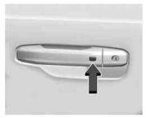
The remote key must be within 1 m (3 ft) of the eTrunk or door being opened or locked. Press the button on the door handle to open. See "Keyless Access Operation" in *Remote Key Operation*
