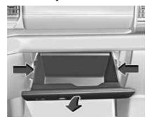
3. Press the sides of the glove box door inward and rotate the door downward to remove.
