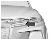
The headlight Charge Status Indicator bar is located on the headlights. As charging occurs, the blue light bars on the headlights fill towards the center of the vehicle.
