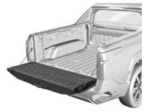
Press x̄z̄ twice quickly on the remote key until the tailgate moves. See Remote Key Operation ⇒ 7. The tailgate can be opened if the remote key is within 1 m (3 ft).
