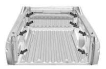
This vehicle is equipped with eight fixed cargo tie-downs.
