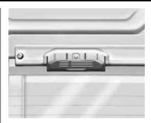
Once the glass stow retainer handle is in the locked position with the corner secures closed, the rear glass is securely stored.
