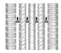
Treadwear indicators are one way to tell when it is time for new tires. Treadwear indicators appear when the tires have only 1.6 mm (1/16 in) or less of tread remaining. See *Tire Inspection* ♀ 323 and *Tire Rotation* ♀ 323.
