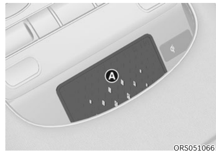
Ⓐ: Vehicle authentication pad (Wireless charging pad)
