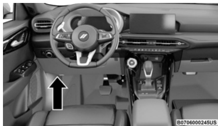
Interior Fuse Box Location
