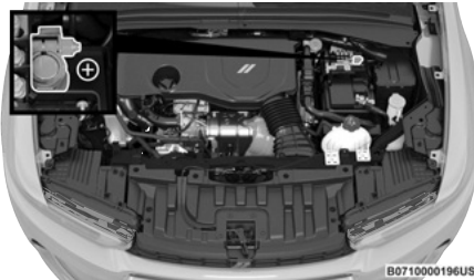
Positive (+) Battery Post
