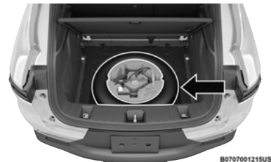
Damaged Tire Stowage
