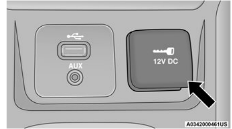
Front Power Outlet
