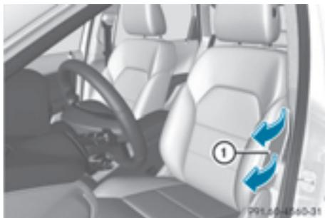
Side impact air bags ① deploy next to the outer bolsters of the seat backrests.
