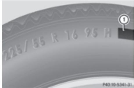
In addition to the load bearing index, load index **1** may be imprinted after the letters that identify speed index **6** on the sidewall of the tire (▷ page 293).
