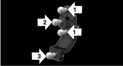
6. Proceed in the reverse order to insert the new bulb and attach the bulb holder. Make sure that the bulb holder engages in all fasteners.
