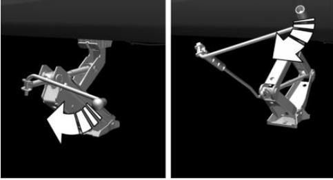
4. Take your hand away from the vehicle jack as soon as the vehicle jack is under load and continue turning the vehicle jack crank or lever with one hand.
