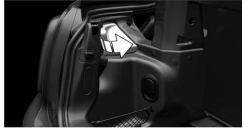
3. Through the opening, loosen the plug connector, arrow 2 on the bulb holder. Press the latches together, arrows 1, and remove the bulb holder.
