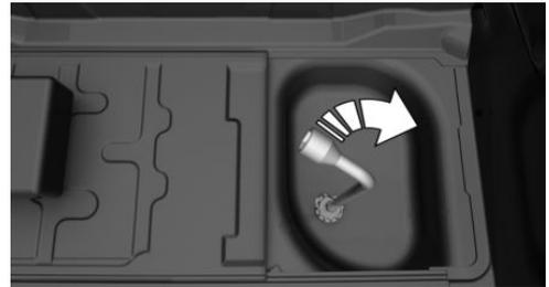
4. Unlock the locking hexagon of the emergency wheel well using the hexagon attached to retaining plate.
