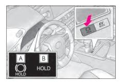
Turns the brake hold system on
