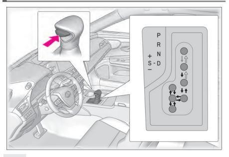
While the power switch is in ON mode and the brake pedal depressed\*, shift the shift lever while pushing the shift release button on the shift knob.
