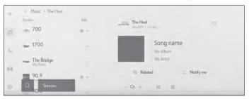
[Ch]: Touch [-] or [+] to search for the receivable channels. Touch and hold to switch channels. When released, the current channel is received.
