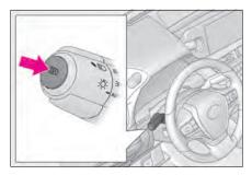
1 Press the Automatic High Beam switch.
