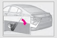
Turn the mechanical key clockwise to open.
