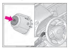
Press the Automatic High Beam switch.
