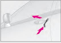
1 Pull the driver's door handle and insert the mechanical key.
