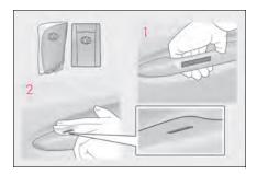
1 Grip the driver's door handle to unlock the door. Holding the driver's door handle for approximately 2 seconds unlocks all the doors. Grip the passenger's door handle to unlock all the doors.\*
