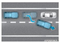
When driving in stop-and-go traffic, and a stopped vehicle in front of you merges out of the lane, FCA system may not immediately detect the new vehicle that is now in front of you. In this case, you must maintain a safe braking distance, and if necessary, depress the brake pedal to reduce your driving speed in order to maintain a safe distance.
