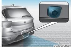
The Rear View Monitor will activate when the engine is running and the shift lever is in the R (Reverse) position.
