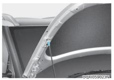
4. Pull out the support rod and hold the hood open with the support rod.
