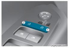
The driver side door armrest is equipped with a central door lock switch. The lock button is indicated by a ( $\widehat{}$ ) symbol. The unlock button is indicated by a ( $\widehat{}$ ) symbol.
