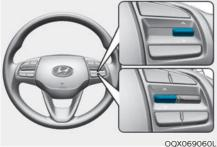
To change the trip mode, toggle the " $\land$ ,  $\checkmark$ " switch on the steering wheel.
