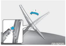
1. Raise the wiper arm and pull out the wiper blade assembly.
