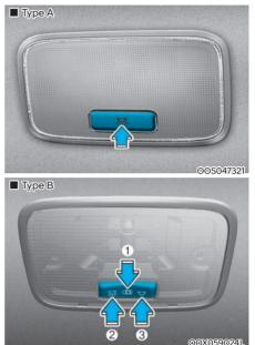
Rear Room Lamp (र्र्ग्नूर): Press this switch to turn the rear room lamp on and off.
