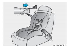
Slowly allow the shoulder portion of the seat belt to retract and listen for an audible "clicking" or "ratcheting" sound. This indicates that the retractor is in the "Automatic Locking" mode. If no distinct sound is heard, repeat steps 3 and 4.
