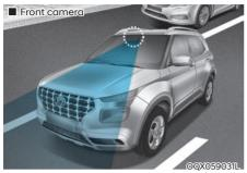
In order for FCA system to operate properly, always make sure the front view camera is clean and free of dirt, snow, and debris. Dirt, snow, or foreign substances on the surface may adversely affect the sensing performance of the camera.
