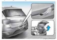
Before attempting to open the liftgate, make sure the vehicle is in PARK (P). To open the liftgate, perform the following.
