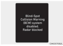
Blind-Spot Collision Warning system disabled. Radar blocked
