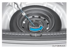
If it is hard to loosen the tire hold-down wing bolt by hand, you can loosen it easily using the jack handle.
