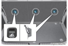
First secure the child restraint with the LATCH lower anchors or the seat belt. If the child restraint manufacturer recommends that the top tether strap be attached, attach and tighten the top tether strap to the top tether strap anchor.
