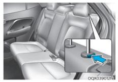
2. Lower the rear head restraints to the lowest position by pushing and holding the release button and pushing down on the head restraint.
