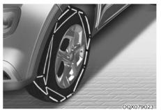
Since the sidewalls of radial tires are thinner than other types of tires, they may be damaged by mounting some types of tire chains on them. Therefore the use of snow tires is preferred over the use of tire chains.
