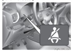
As a reminder to the driver, the seat belt warning light will illuminate for approximately 6 seconds each time you place the ignition switch to the ON position regardless of belt fastening. However, if the seat belt is unfasted, a warning chime will sound for approximately 6 seconds.
