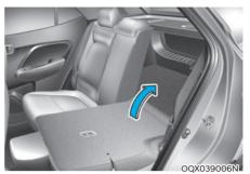
5. To use the rear seat, lift and unfold the seatback to the upright position. Push the seatback firmly until it clicks into place. Make sure the seatback is locked in place.
