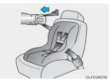
4. Pull the shoulder portion of the seat belt all the way out. When the shoulder portion of the seat belt is fully extended, it will shift the retractor to the "Automatic Locking" (child restraint) mode.
