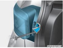
Stop/tail lamp and turn signal lamp replacement
