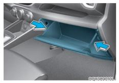
1. With the glove box open, push in both sides of the glove box as shown. This will ensure that the glove box stopper pins will get released from its holding location allowing the glove box to hang.
