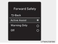
• Setting Forward Safety function The driver can activate FCA by placing the ignition switch to the ON position and by selecting:
