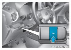
To activate/deactivate LKA system: With the ignition switch in the ON position, press LKA system button located on the instrument panel on the left hand side of the steering wheel. The indicator in the cluster display will initially illuminate white. This indicates LKA system is in the READY but NOT ENABLED state.
