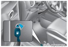
The fuel filler door is opened from inside the vehicle using the fuel filler door release lever.
