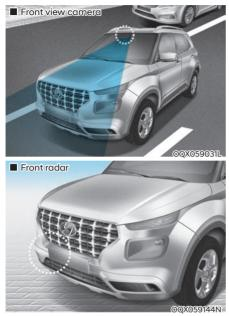
In order for FCA system to operate properly, always make sure the sensor cover or sensor is clean and free of dirt, snow, and debris.
