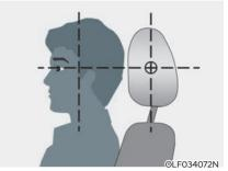
Adjust the head restraints so the middle of the head restraint is at the same height as the height of the top of the eyes.
