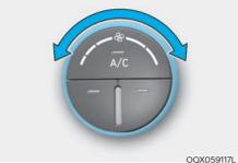
The fan speed can be set as desired by pushing the fan speed control button. More air is delivered with higher fan speeds.
