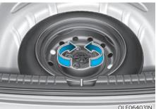
Turn the winged hold down bolt counterclockwise to remove the spare tire
