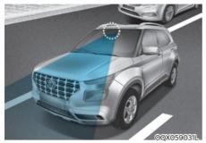
Lane Keeping Assist system helps detect lane markers on the road with a camera at the front windshield, and assists the driver's steering to help keep the vehicle between lanes.
