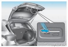
Your vehicle is equipped with an emergency liftgate safety release lever located on the bottom of the liftgate inside the vehicle. To unlock and open the liftgate manually from inside the luggage compartment, perform the following steps:
