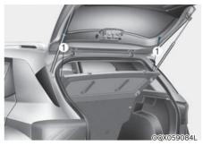
Use the cover to hide items stored in the cargo area. The cargo area cover will lift when the liftgate is opened. Disconnect the strap (1) from the holder if you want to return the cover to the original position. To remove the cargo area cover completely, pull the cover backward and out from the rail. To secure a wider space, pull the cargo area cover backward slightly and push down it.
