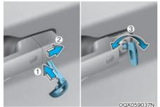
If you lock the driver's door with a mechanical key, all vehicle doors will lock. If you unlock the driver's door with a mechanical key, you can open and close the driver's door only.
