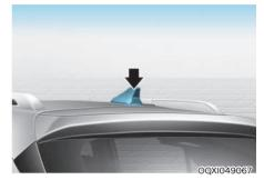
The shark fin antenna receives transmitted data. (for example: AM/FM, SXM, GPS, LTE)
