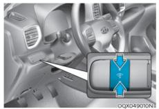
When the vehicle's parking lamps or headlamps are on, press the illumination control button to adjust the brightness of the instrument panel illumination.
