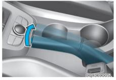
Check the stroke of the parking brake by counting the number of "clicks" heard while fully applying it from the released position. Also, the parking brake alone should securely hold the vehicle on a fairly steep grade. If the stroke is more or less than specified, have the parking brake adjusted by an authorized HYUNDAI dealer.
