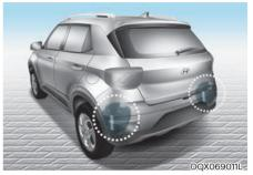
The rear corner radars are located inside the rear bumper for detecting the side and rear areas. Always keep the rear bumper clean for proper operation of the system.
