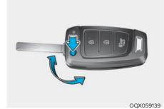
If the remote key does not operate normally, you can lock or unlock the driver's door by using the mechanical key. To unfold the mechanical key, press the release button on the remote.
