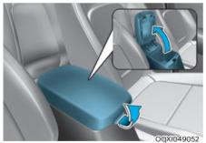
To open: Grab and hold the latch (1) on the arm rest then lift the lid.
