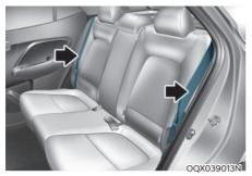
3. Locate the seatbelt toward the outboard position before folding down the seatback. If not, the seatbelt system may be interfered by the seatback.
