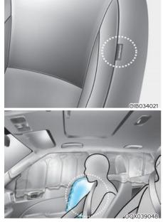
Your vehicle is equipped with a side air bag in each front seat. The purpose of the air bag is to provide the vehicle's driver and the front passenger with additional protection than that offered by the seat belt alone.
