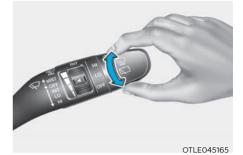
The rear window wiper and washer switch is located at the end of the wiper and washer switch lever. Turn the switch to the desired position to operate the rear wiper and washer.
