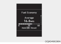
The trip computer mode displays information related to vehicle driving parameters including fuel economy, trip meter information and vehicle speed.
