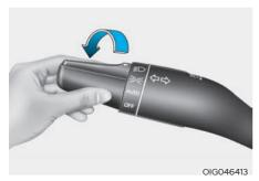
Headlamp position (ﷺ) The headlamp, parking lamp, license plate lamp and instrument panel lamp are turned ON.
