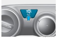
Push the A/C button to turn the system on (indicator light will illuminate) and off.
