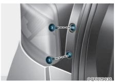
4. Remove the rear combination lamp assembly from the body of the vehicle.
