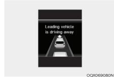
The system notifies the driver with the alert message and a warning sound when the leading vehicle drives away while a stop.
