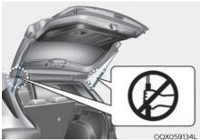
Do not hold on to or try to pull on the liftgate strut. Be aware that the deformation of the liftgate strut may cause vehicle damage and risk of injury.
