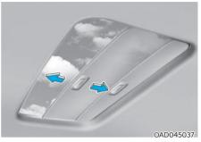
The sunshade can be opened and closed manually. However, the sunshade will open automatically with the sunroof when the glass panel moves. If you want it closed, move the sunshade manually.
