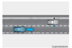
Blind-Spot Collision Warning system will alert you when it detects a vehicle is approaching in an adjacent lane at a high rate of speed. If the driver activates the turn signal when the system detects an oncoming vehicle, the system sounds an audible alert.
