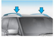
If your vehicle comes equipped with roof side rails, then roof side rails crossbars can be installed on top of your vehicle.
