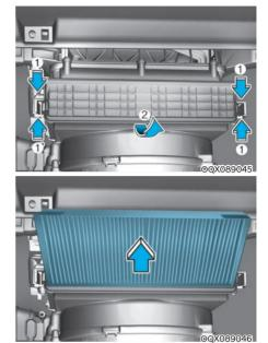
2. Open the climate control air filter cover (2) by pushing or pressing the clip (1) on the right and left side.
