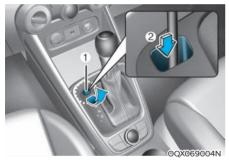
If the shift lever cannot be moved from the P (Park) position into R (Reverse) position with the brake pedal depressed, continue depressing the brake, and then do the following:
