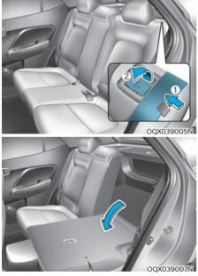
Pull out the seatbelt from guide (1) and pull up the seatback folding lever (2), then fold the seat toward the front of the vehicle.
