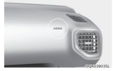
The purpose of the SRS is to provide the vehicle's driver and front passengers with additional protection than that offered by the seat belt system alone.
