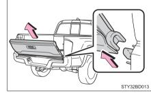
3 Slide the tailgate a little to the right to unhook the left side being mindful of tailgate right-hand side clearance to vehicle's rear bumper.
