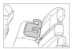
2 Sit the child in the child restraint system. Fit the seat belt to the child restraint system according to the manufacturer's instructions and insert the plate into the buckle. Make sure that the belt is not twisted.
