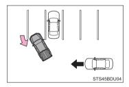
Vehicles that the sensors cannot detect due to obstructions
