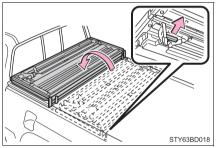
4 Secure by using the storage straps.
