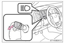
Press the Automatic High Beam switch.
