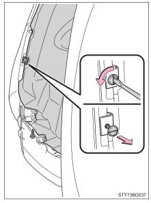
2 Open the fender liner and turn the bulb counterclockwise.
