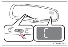
3 Drive the vehicle at 5 mph (8 km/h) or less in a circle until a direction is displayed.
