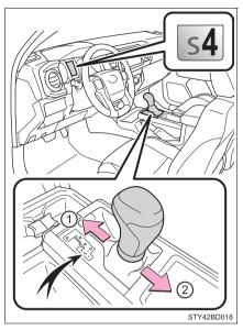
The initial shift range in S mode is set automatically to 5 or 4 according to vehicle speed. However, the initial shift range may be set to 3 if the AI-SHIFT has operated while the shift lever was in the D position.  $(\rightarrow P. 213)$
