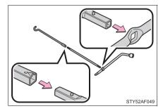
Insert the end of the jack handle extension into the lowering screw and turn it counterclockwise.
