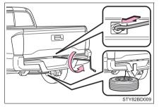
3 After the tire is lowered completely to the ground, remove the holding bracket.
