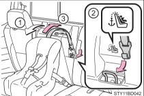
3 Secure the child restraint system using the seat belt or the lower anchors, and tighten the top tether strap.
