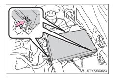
Under the instrument panel Remove the cover.
