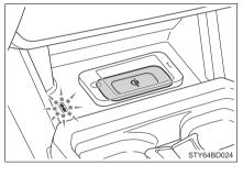
When placing the mobile device on the wireless charging surface of the tray, make sure that there are no objects in-between the mobile device and the tray. They may interfere with charging.
