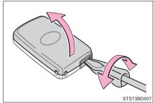
Remove the depleted battery.
