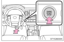
Continue depressing the brake pedal until the engine is completely started.
