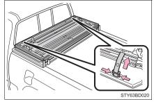
Close the tonneau cover and push down on the top surface (latch position) until it clicks.
