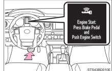
Press the engine switch shortly and firmly.
