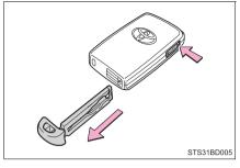
After using the mechanical key, store it in the electronic key. Carry the mechanical key together with the electronic key. If the electronic key battery is depleted or the entry function does not operate properly, you will need the mechanical key. (→P. 528)
