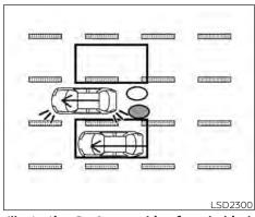
Illustration 2 - Approaching from behind Illustration 2: If the driver activates the turn signal when another vehicle is in the detection zone, then the system chimes (twice) and the side BSW/RCTA indicator light flashes.
