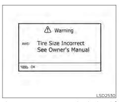
The tire size message may be displayed if there is a large difference between the diameters of front and rear wheels. Pull off the road in a safe area, with the engine idling. Check that all tire sizes are the same, that the tire pressure is correct and that the tires are not excessively worn.
