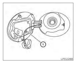
To remove the fuel-filler cap:
