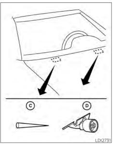
If you wax the surface of the hood, be careful not to let wax get into the washer nozzle ①. This may cause clogging or improper windshield-washer operation. If wax gets into the nozzle, remove it with a needle or small pin (3).
