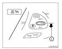
To set cruising speed, accelerate your vehicle to the desired speed, push the SET/-© switch and release it. (The color of the cruise indicator changes to green and set vehicle speed indicator comes on.) Take vour foot off the accelerator pedal. Your vehicle will maintain the set speed.
