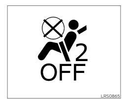
7 If the booster seat is installed in the front passenger seat, place the ignition switch in the ON position. The front passenger air bag status light 3 may or may not illuminate, depending on the size of the child and the type of booster seat being used. For additional information, see "Front passenger air bag and status liaht" (P. 1-60).
