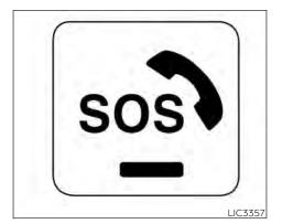
The E-call (SOS) button is used in combination with a NissanConnect® Services subscription to call for assistance in case of an emergency.
