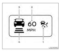
Vehicle-to-vehicle distance control mode display and indicators
