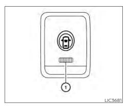
The dynamic driver assistance switch is used to temporarily activate the Intelligent Lane Intervention (I-LI) system that is enabled using the settings menu of the vehicle information display.
