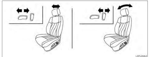
FRONT POWER SEAT ADJUSTMENT (if so equipped)
