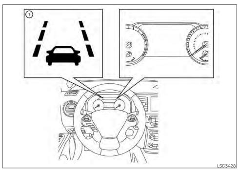
are clear. When the vehicle approaches either the left or the right side of the traveling lane, the steering wheel will vibrate and the LDW indicator ① on the instrument panel will blink to alert the driver.
