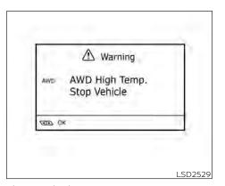
The AWD high temperature message may be displayed while trying to free a stuck vehicle due to increased oil temperature. The driving mode may change to 2-Wheel Drive (2WD). If this message is displayed, stop the vehicle with the engine idling, as soon as it is safe to do so. Then if the message turns off, you can continue driving.
