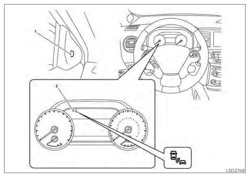
When the shift position is in R (Reverse) and the vehicle speed is less than approximately 5 mph (8 km/h), the RCTA system is operational.
