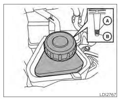
Check the fluid level in the reservoir.
