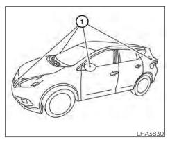
If dirt, rain or snow accumulates on any of the cameras (1), the MOD system may not operate properly. Clean the camera by wiping with a cloth dampened with a diluted mild cleaning agent and then wiping with a dry cloth.
