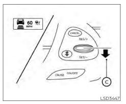
To set cruising speed, accelerate your vehicle to the desired speed, push the SET/switch (a) and release it. The ICC system set indicator (green), vehicle ahead detection indicator set distance indicator and set vehicle speed indicator (B) will come on. Take your foot off the accelerator pedal. Your vehicle will maintain the set speed.
