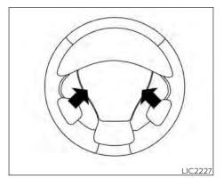
To sound the horn, push near the horn icon on the steering wheel.
