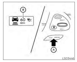
Operating vehicle-to-vehicle distance control mode
