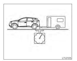
The Gross Combined Weight Rating (GCWR) equals the combined weight of the towing vehicle (including passengers and cargo) plus the total trailer load. Towing loads greater than these or using improper towing equipment could adversely affect vehicle handling, braking and performance.
