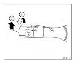
When the vehicle speed lowers to less than approximately 16 mph (25 km/h), the head-light uses the low beam.
