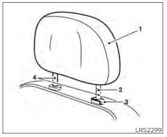
NON-ADJUSTABLE HEAD RESTRAINT/HEADREST COMPONENTS
