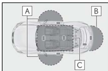
**A** When locking or unlocking the doors
