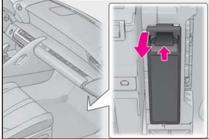
**3** Remove the fuse with the pullout tool.
