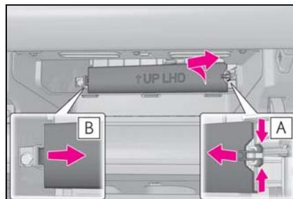
**5** Remove the filter case.
