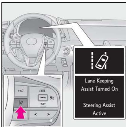
**B** Operation display of steering wheel operation support
