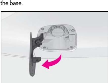
**3** Turn the fuel tank cap slowly and remove it, then put it into the holder on the fuel filler door.
