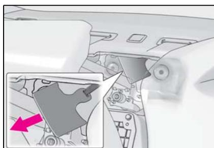
LC500h: Using the tab to open the fuel filler door may not allow for an adequate reduction in fuel tank pressure before refueling. To prevent fuel from spilling out, turn the cap slowly when removing it. During refueling, fuel may spill out from
