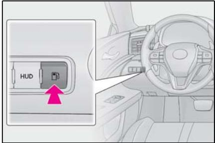
**2** Open the fuel filler door until it is securely locked.
