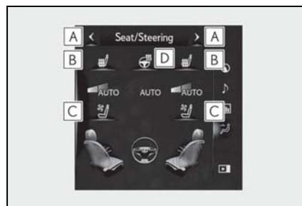
**A** Display the air conditioning control screen (→P.255)
